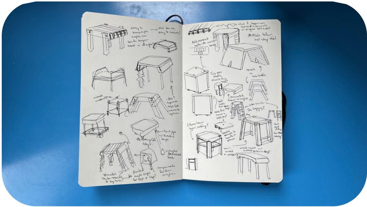
Figure 3. Sketches of the side table series. Note. This photo demonstrates phase 2 in the design process of rapid sketches of forms and details.
