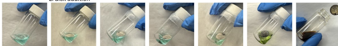
Figure S4.6. Compatibility tests of NST and Li metal disks in two electrolytes: 1 M LiPF 6 in EC/DMC (top row) and 1M LiTFSI in DOL/DME (bottom row). Each row shows (from left to right) the electrolyte containing NSB before Li addition, immediately after the addition of the Li disk, and after 3, 6, 24, 48 and (for LiPF 6 ) 168 h.
