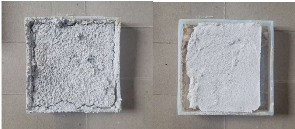
Figure 4.6 Early recycled gypsum prototypes, using powder that is too coarse (left) or too much water (right). Image by Elizabeth Vince.
