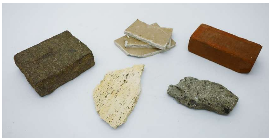
Figure 5.22 Construction waste presented to participants. Clockwise from top left: stone block, drywall, brick, concrete, planed stone. Image by Elizabeth Vince.
