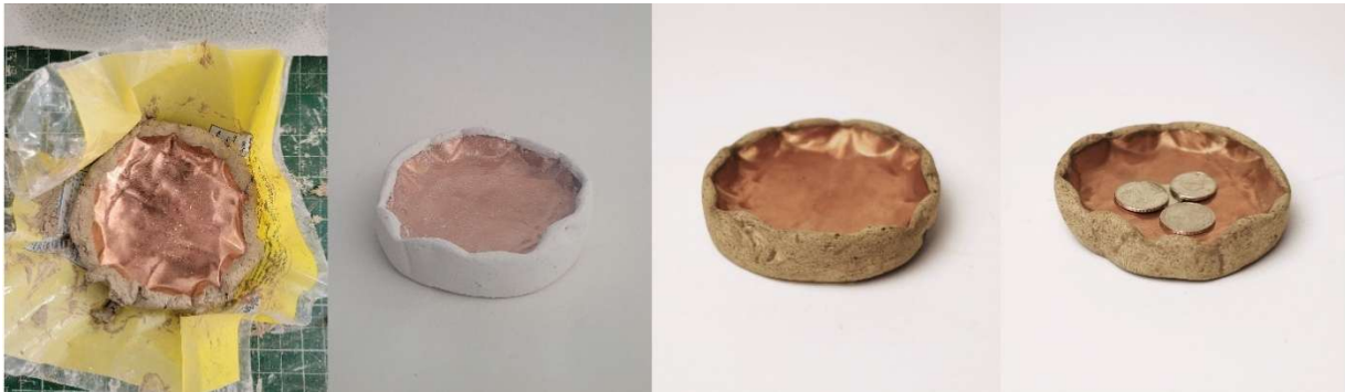
Figure 5.10 From left to right: Recycled gypsum Tray #2 in the mold, after carving and sanding, and after sealing. This is an example of the carving required for most prototypes. Image by Elizabeth Vince.
