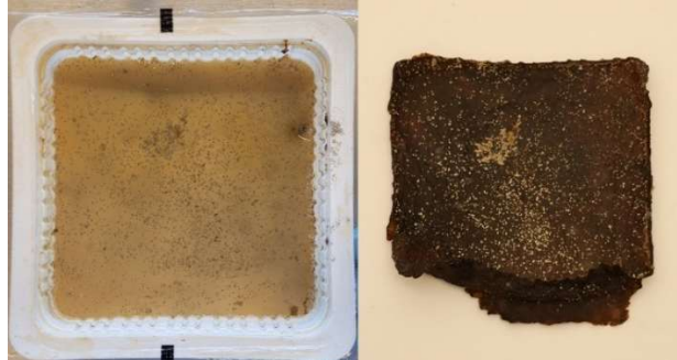
Figure 4.13 The process of adding CR to an in-progress SCOBY, and the SCOBY after drying. Image by Elizabeth Vince.
