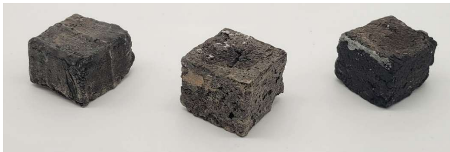
Figure 4.11 Refined CR biocomposite prototypes with different finishes, from left to right: beeswax, no finish, drying oil. Image by Elizabeth Vince.
