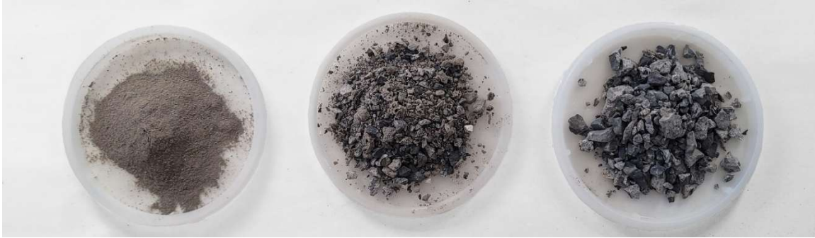
Figure 4.8 Construction residue grades. From left to right: dust, fine aggregate, medium aggregate. Image by Elizabeth Vince.
