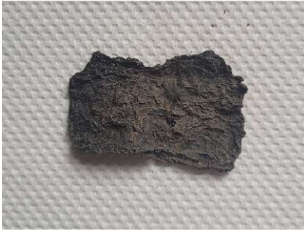
Figure 4.12 A piece of SCOBY after being massaged with CR and drying. Image by Elizabeth Vince.
