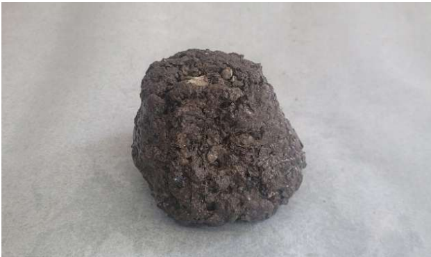
Figure 5.3 CR biocomposite deforming after being molded. Image by Elizabeth Vince.
