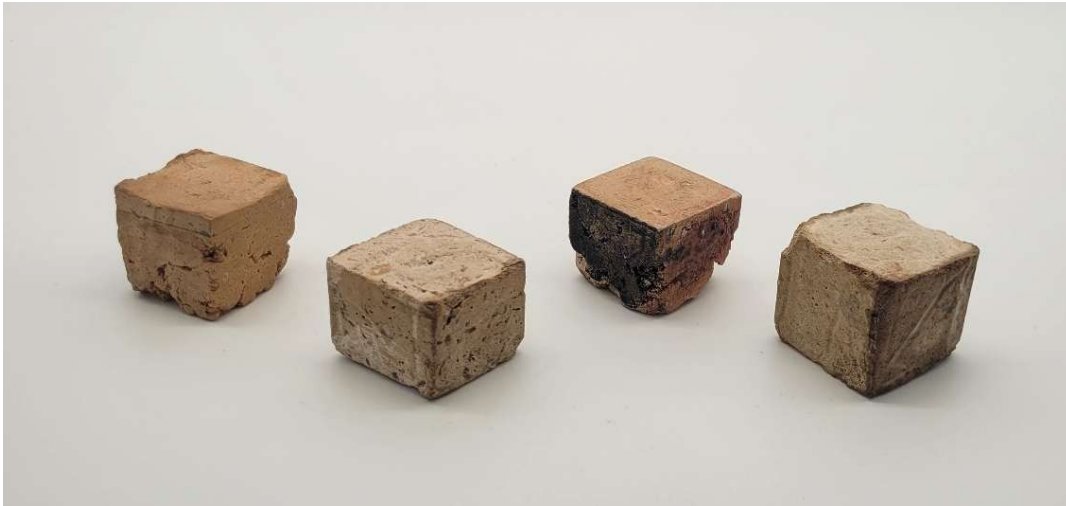
Figure 4.7 Refined recycled gypsum prototypes. From left to right: sealed with drying oil, no sealant, testing various colourants in beeswax, and wax polish. Colourants were not pursued past the material prototyping stage. Image by Elizabeth Vince.
