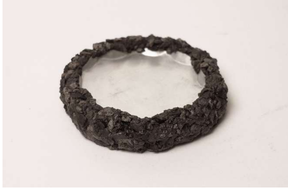
Figure 5.15 Tray #1 : CR biocomposite base, aluminum inlay. Image by Elizabeth Vince.
