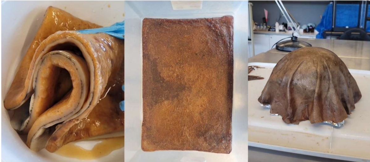
Figure 5.21 From left to right: The layers of construction residue in the SCOBY, the SCOBY drying flat, and the SCOBY draped over a form. Image by Elizabeth Vince.
