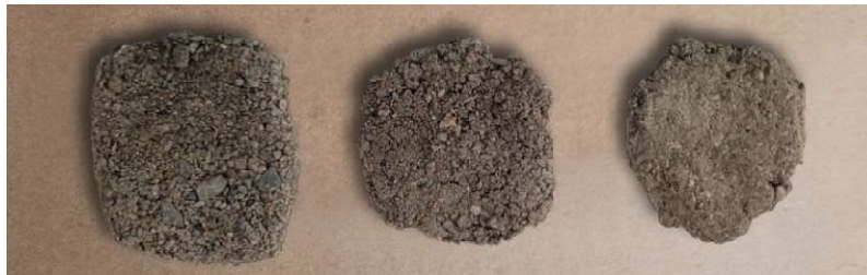
Figure 4.10 Testing different grades of construction residue in the biocomposite. From left to right: only fine aggregate, a mix of fine aggregate and dust, and only dust. Image by Elizabeth Vince.
