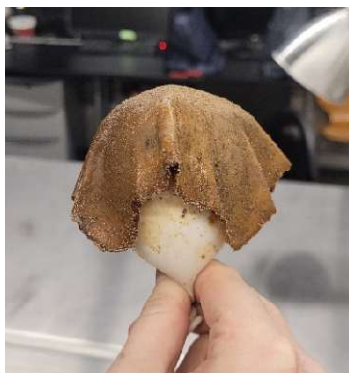
Figure 4.14 Testing draping SCOBY over a balloon. Image by Elizabeth Vince.
