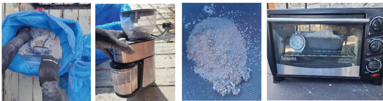
Figure 4.5 Gypsum recovery process. From left to right: crushing, grinding, sieving/filtering, and calcining. Image by Elizabeth Vince.
