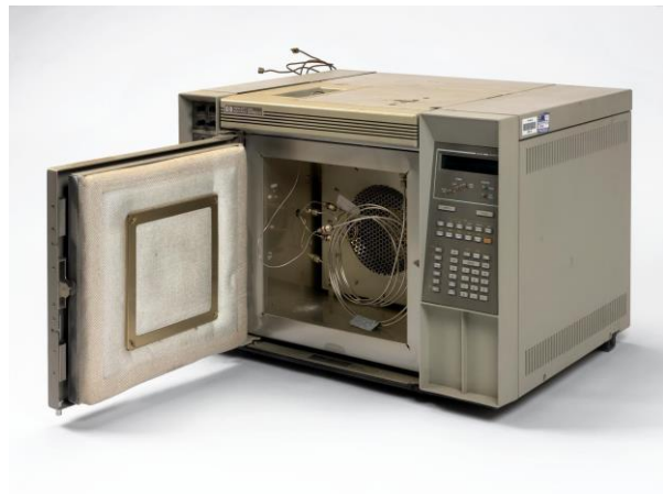
Figure 4.14 Gas Chromatograph HP 5890 by Hewlett-Packard. Computer aided interfaces are now ubiquitous in instruments. 1995. United States. Photo: Science Museum Group. License CC0 1.0 and CC BY 4.0
