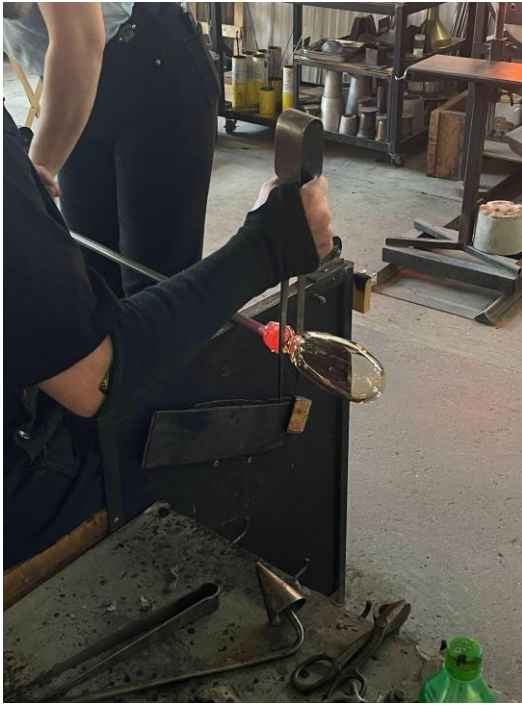
Figure 3.15 Jacklining a bubble, Philippe Vandal, 2024. Matane, Canada. Photo: Philippe Vandal
