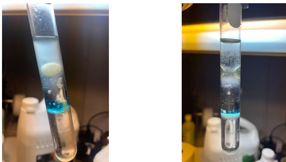
Figure 3.20 Solvent experiments. The various density layers through the test tube starting from the bottom: water, blue coloured engine oil, kerosene, mineral spirits, paraffin. 2024. Montreal, Canada. Photo: Philippe Vandal
