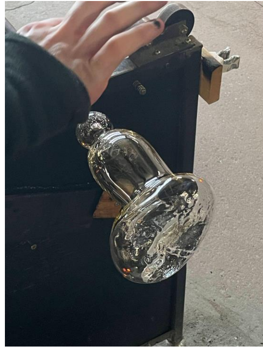
Figure 3.16 Finalizing the bubble before annealing, Philippe Vandal, 2024. Matane, Canada. Photo: Philippe Vandal
