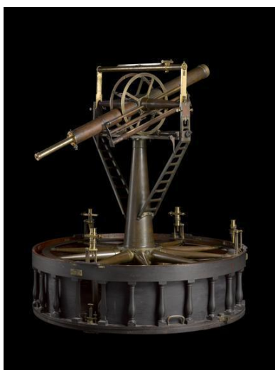
Figure 4.9 Main part of three-foot geodetic theodolite made by Jesse Ramsden. Carved columns can be seen on the base of the instruments. 1791. London, United Kingdom. Photo: Science Museum Group. License CC0 1.0 and CC BY 4.0
