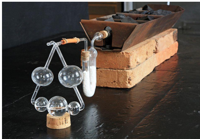
Figure 3.9 The Kaliapparat, invented by Justus von Liebig, 1831. Photo: Eberhard Theophel. License CC BY-SA 3.0 DE
