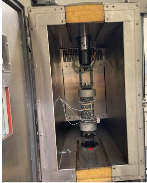
Figure 30: Cylinder Testing Set-up
