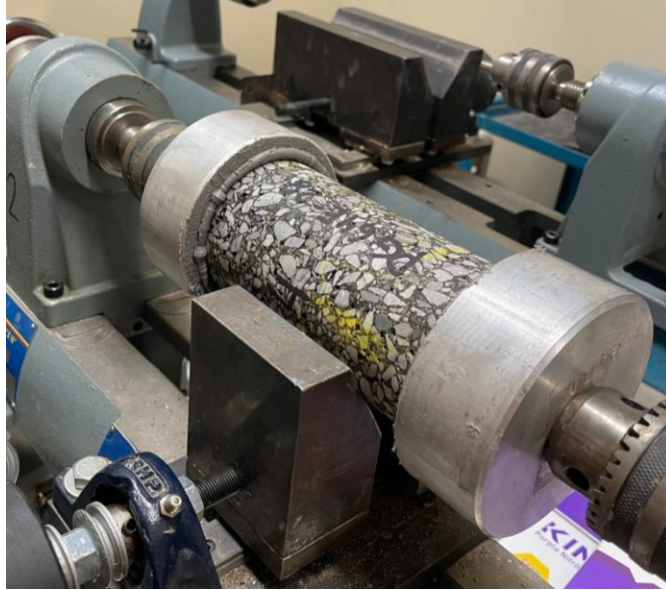
Figure 28: Cylindrical Sample Epoxy Gluing
