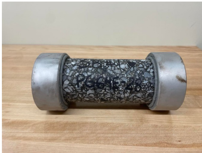
Figure 29: Glued Sample Prepared for Testing
