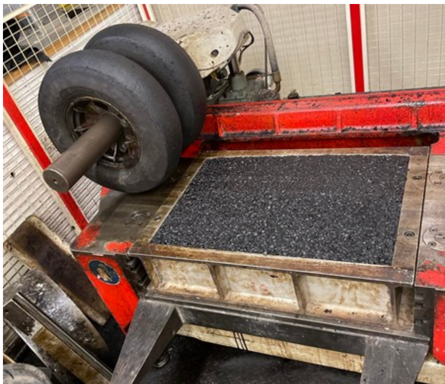
Figure 22: Asphalt Slab Compaction
