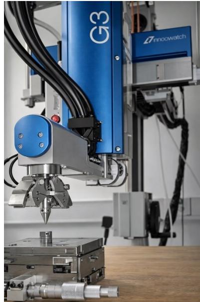
Fig 4.13 Residual stress measurement using the G3 X3000 diffractometer from Stresstech
