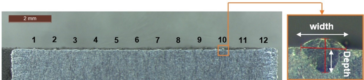
Fig 4.6 Micrographs of vertical cross-sections (Y-Z plane) of samples with 20 \mu m layer thickness
