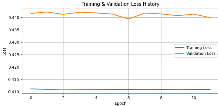
Figure 3.3: Training and validation loss curves of the Refined Gated WaveNet, showing stable convergence and good generalization.
