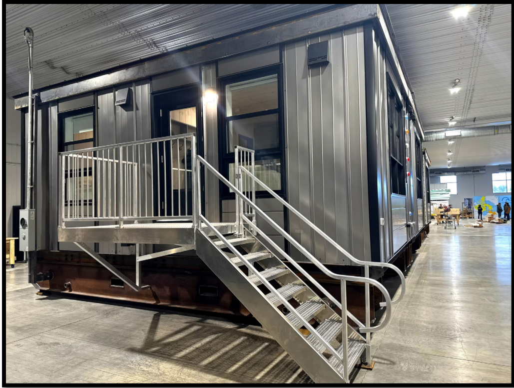
Figure 5: Prefabricated Unit (16 × 24 ft)
