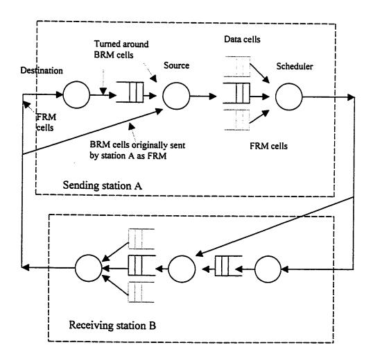
Figure 1: Overview of ABR PEFSM machines and cell flow<sup>[2]</sup>
