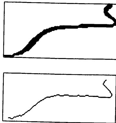
Figure 3-5: A sample sub-word image and its skeleton
