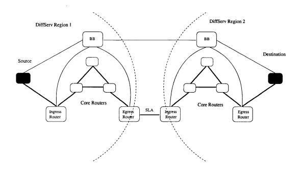
Figure 3: DiffServ Architecture
