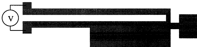
Figure 3-5. Schematic diagram of micro-switch design (I) for MUMPs technology.
