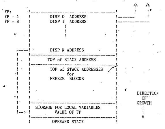
The activation record contains pointers to all the activation records for procedures that surround it. These are needed to reference variables which are not local to the current procedure.
