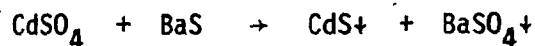
Figure 39. Coprecipitation of Cadmium Sulfide and Barium Sulfate (Cadmium Yellow Lithopone) From Cadmium Sulfate and Barium Sulfide.
