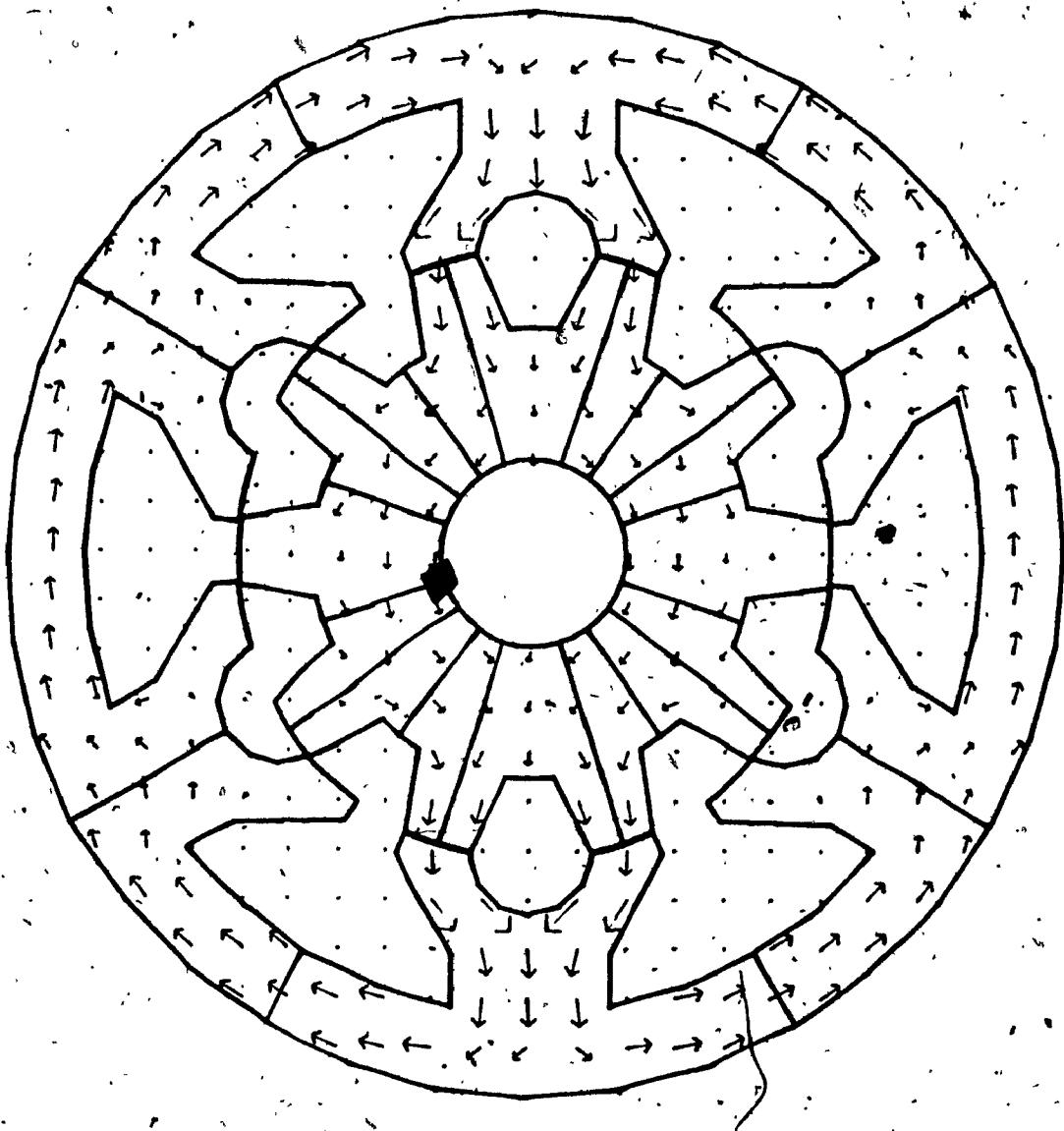
Fig. 8.11 Flux density plot for 3D-solution
