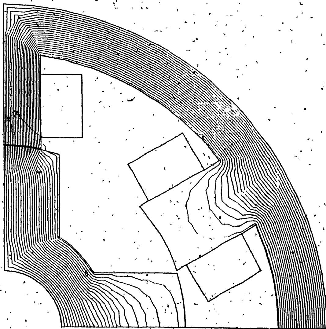
Fig. 3.5 Flux plot. Aligned position.
