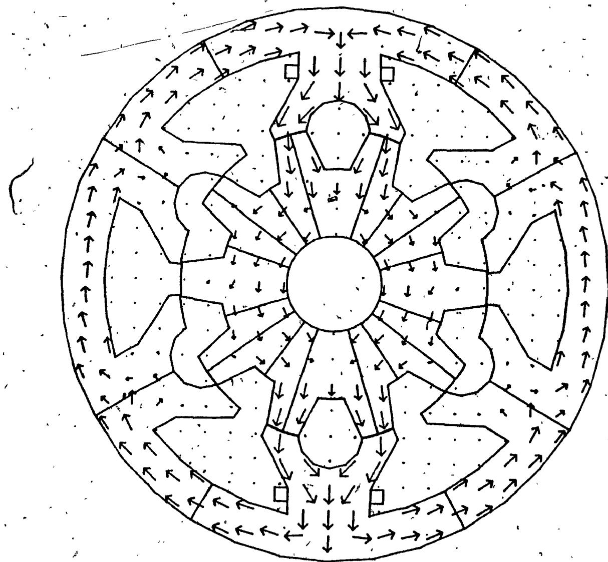
Fig. 6.9 Flux density plot for 2D solution
