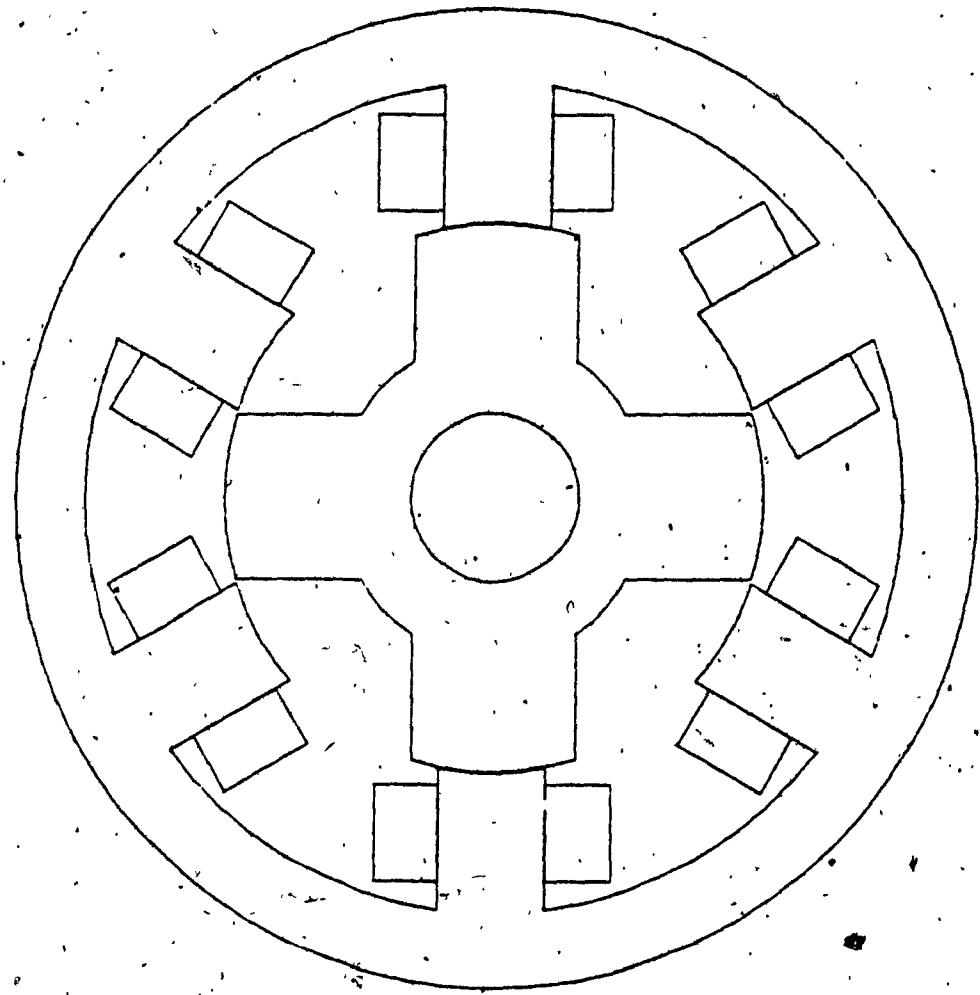
Fig. 3.1 Motor configuration in aligned position (6/4 motor)
