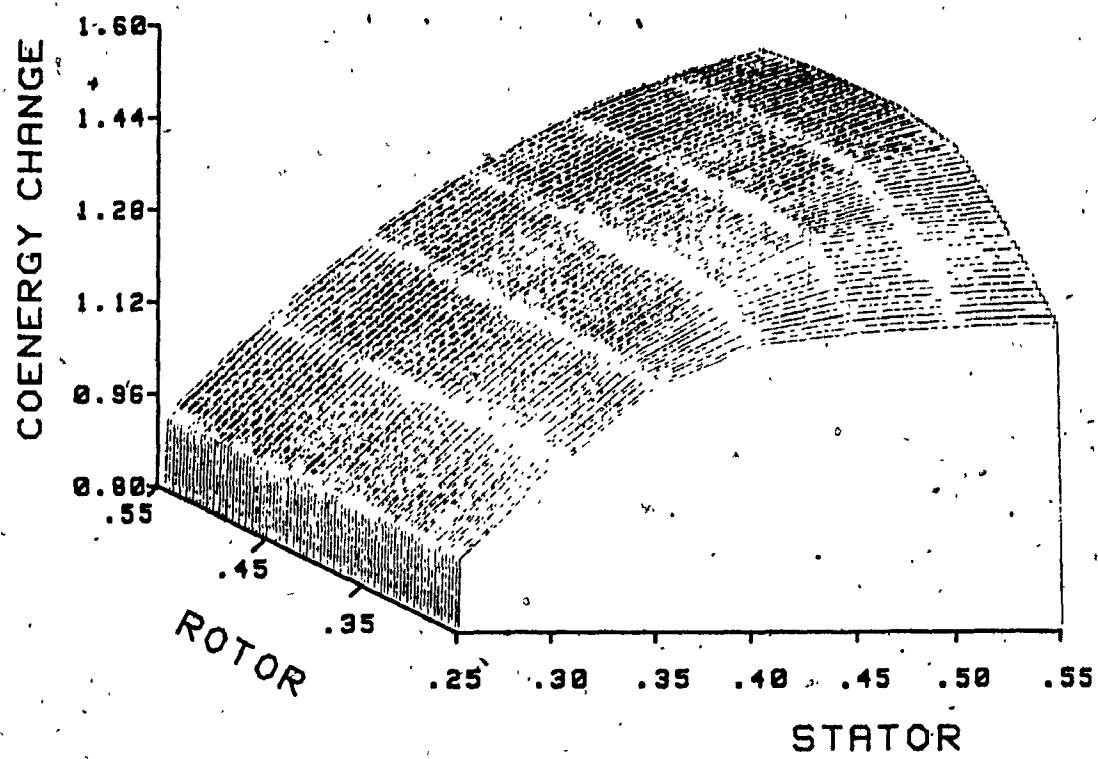
Fig. 4.4 Average torque vs pole arc/pole pitch ratios of stator
