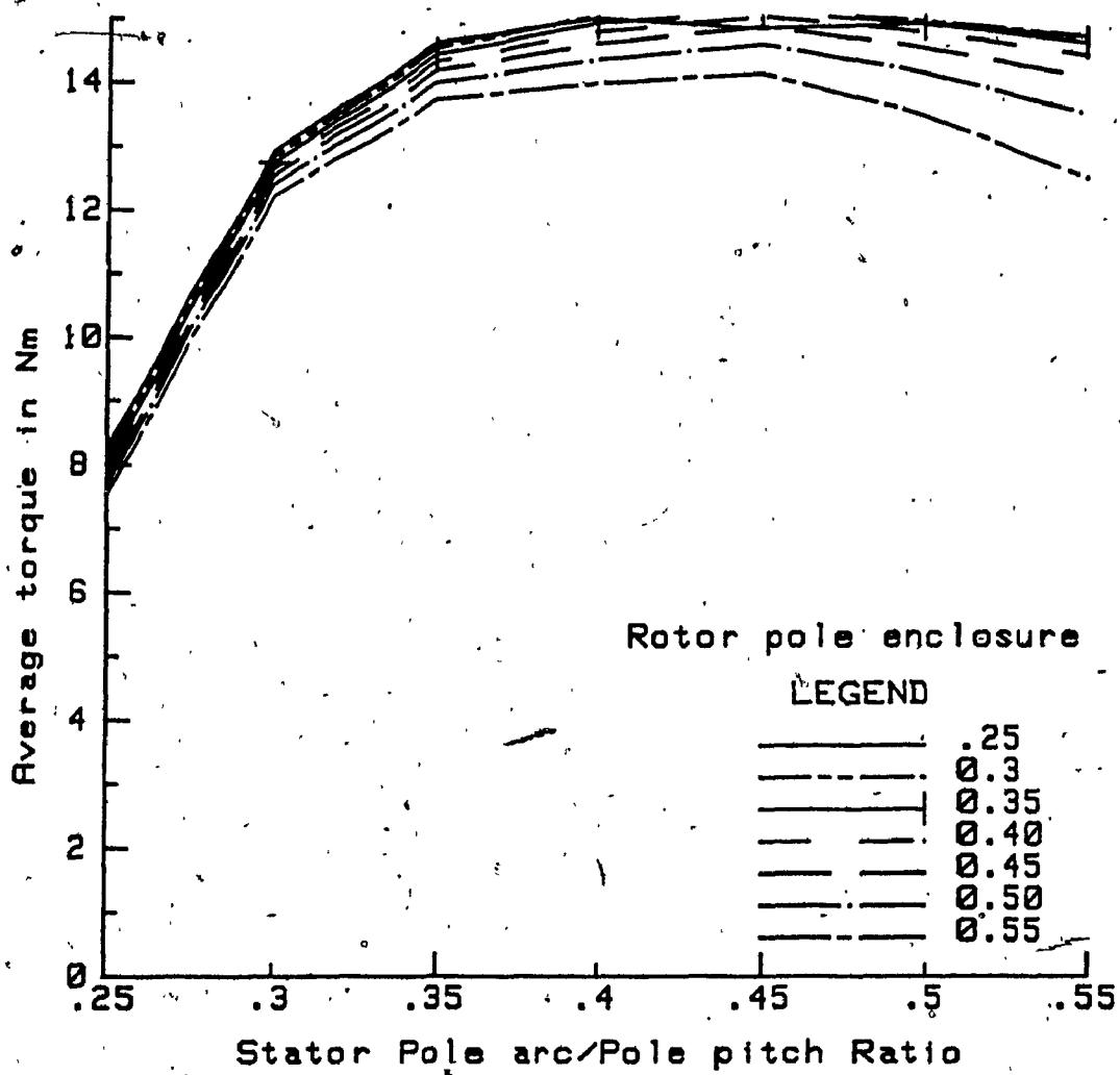
Fig. 4.2      Average torque vs stator pole arc/pole pitch ratio
