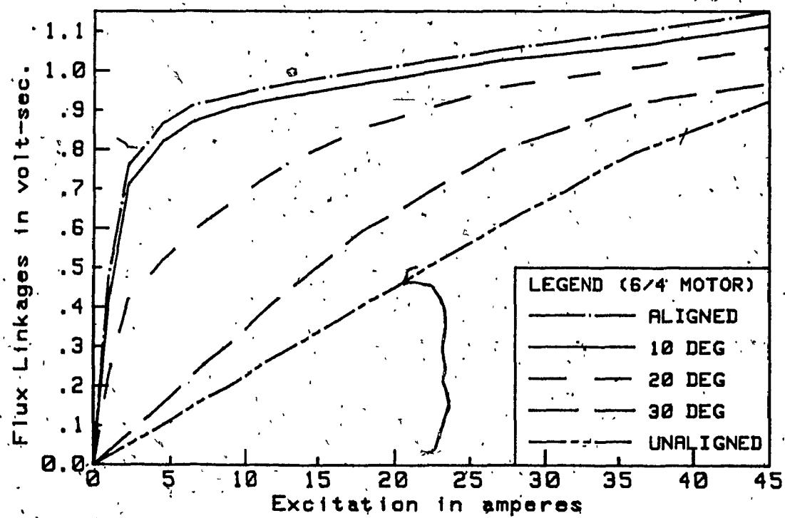
Fig. 3.10 Flux linkages per pole vs current characteristic
