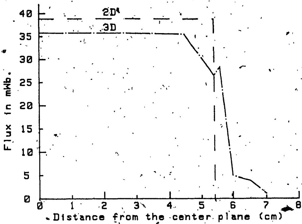
Fig. 6.17 Flux under a stator pole in the axial direction
