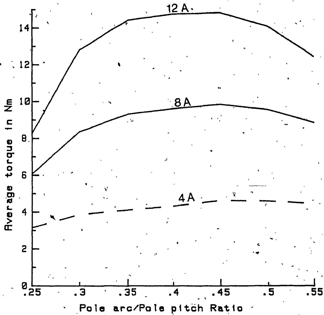
Fig. 4.3      Average torque vs pole arc/pole pitch ratio
