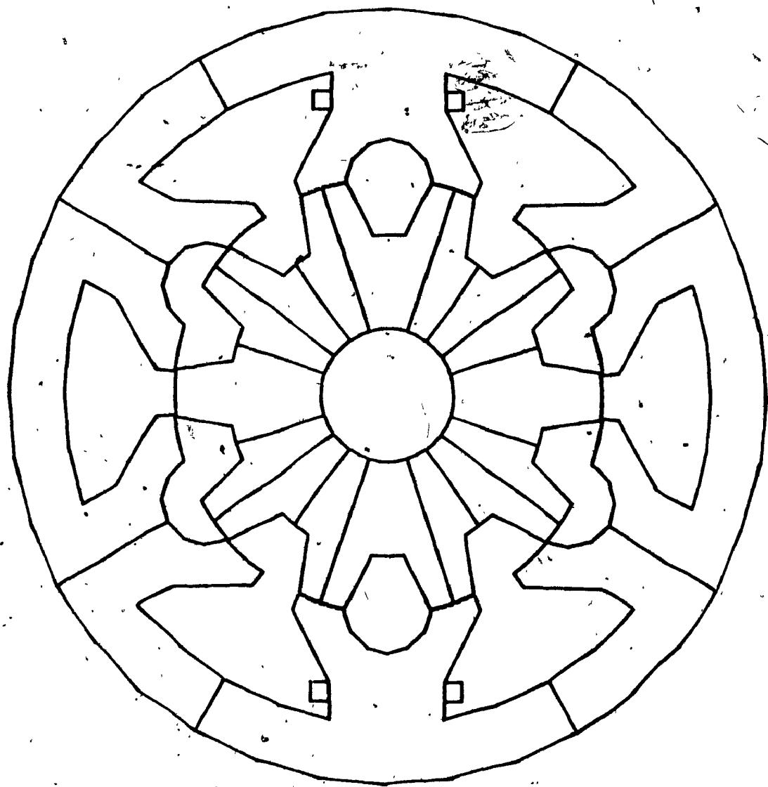
Fig. 6.1. Motor configuration used for 2D analysis
