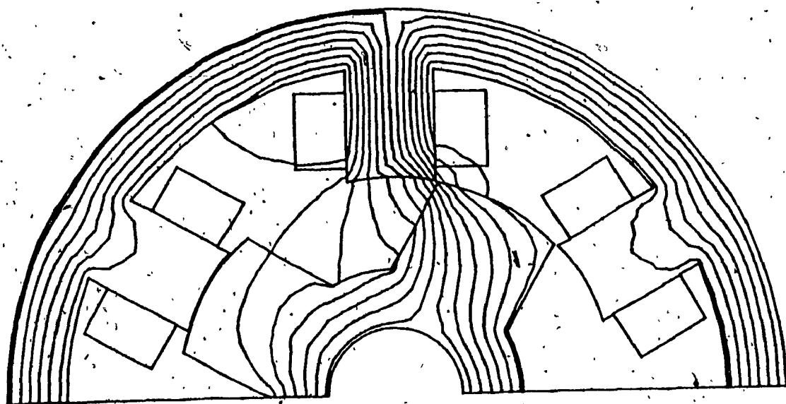
Fig. 3.9 Flux plot. Rotor pole axis at 30 degrees from the aligned position.
