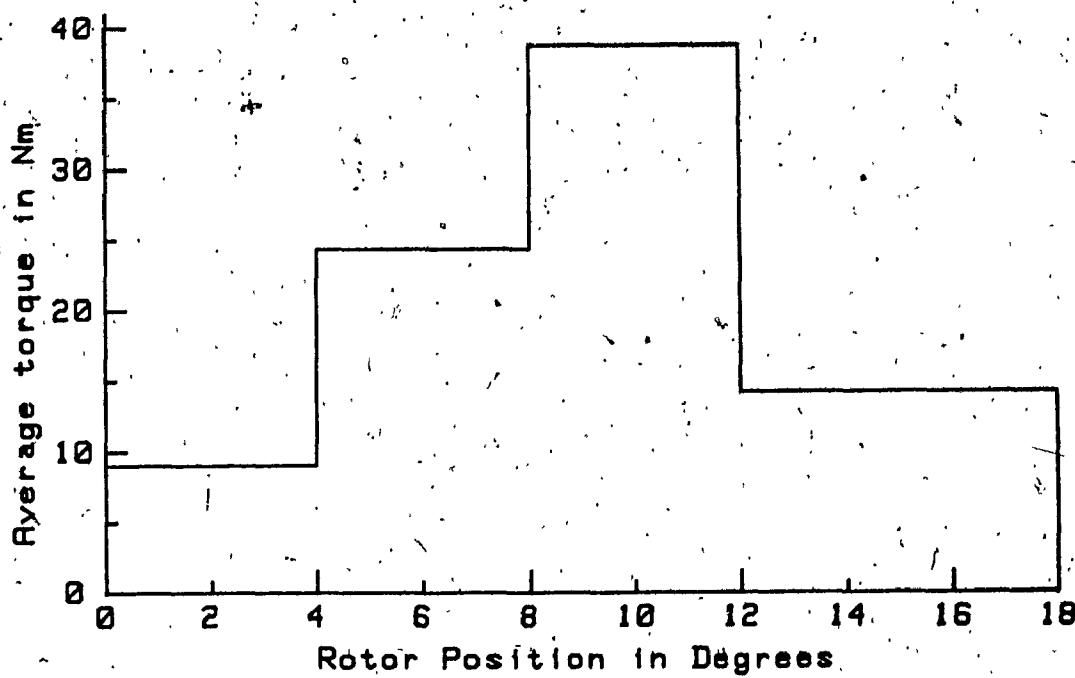
Fig. 3.27      Average torque vs rotor position for 6 A excitation
