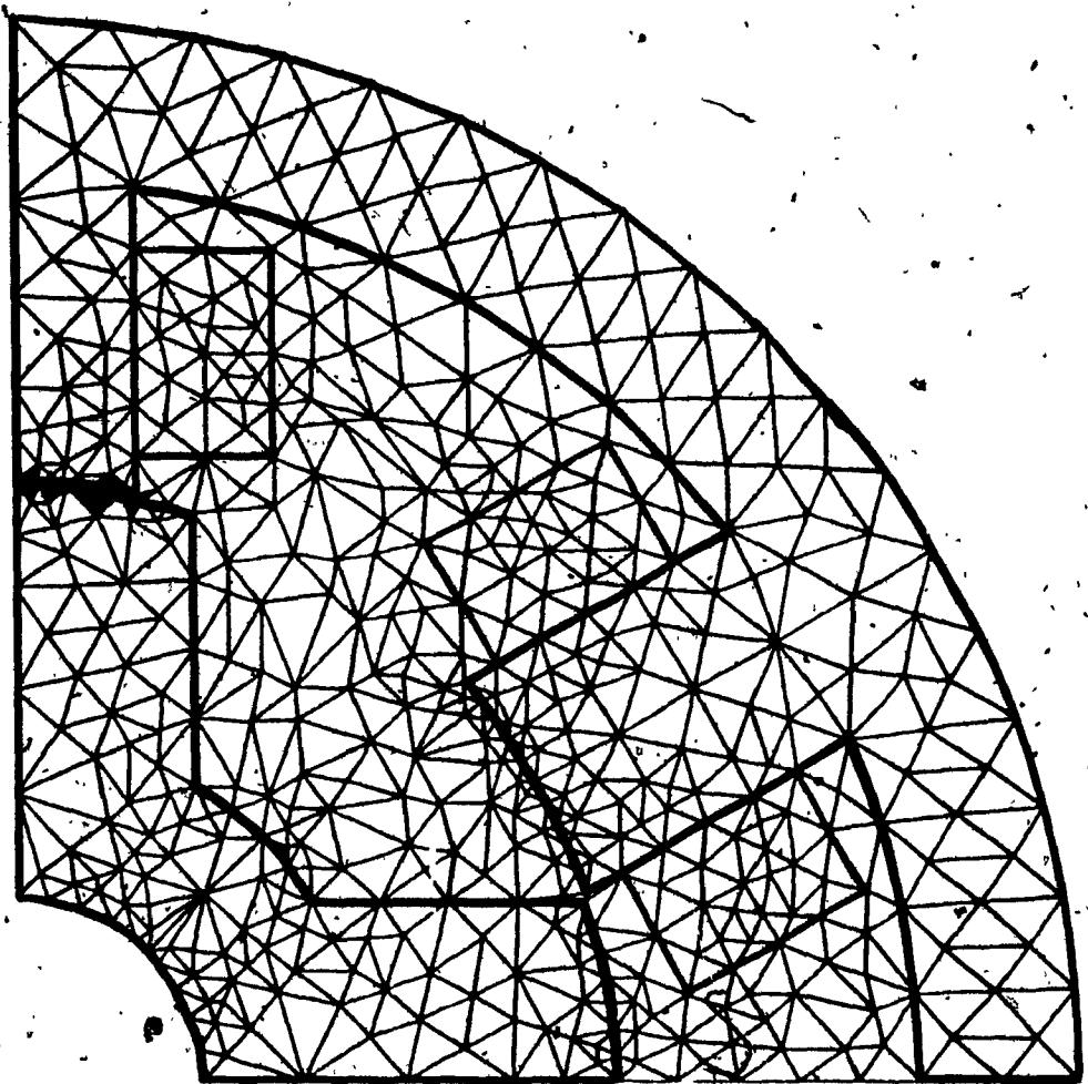
Fig. 3.4 Finite element subdivision of the motor model
