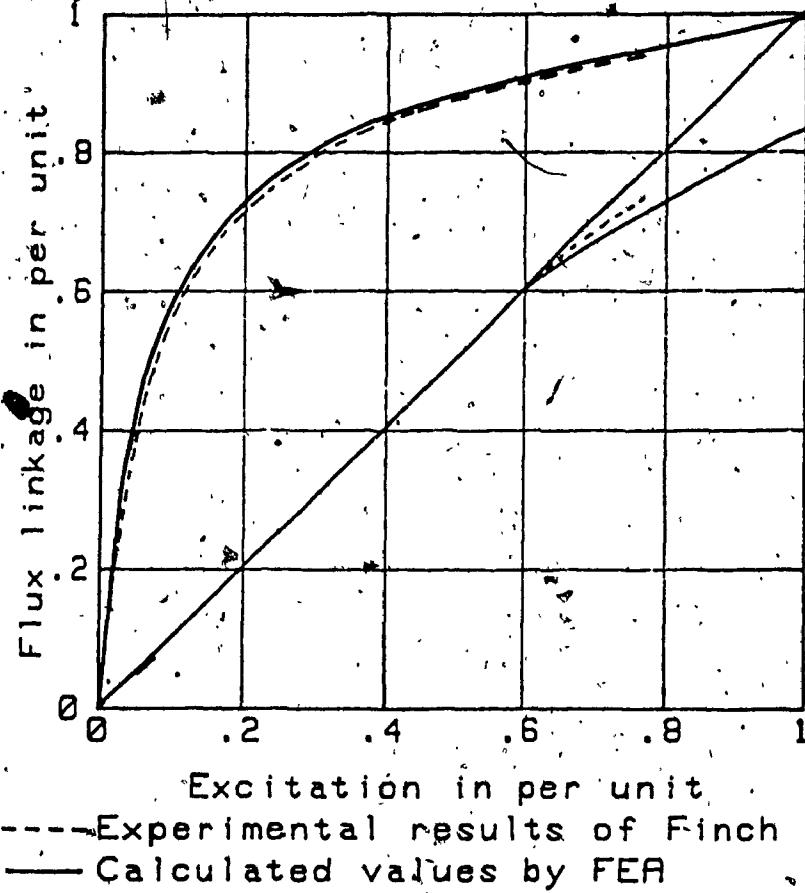
Fig. 3.23 Comparison of flux linkages
