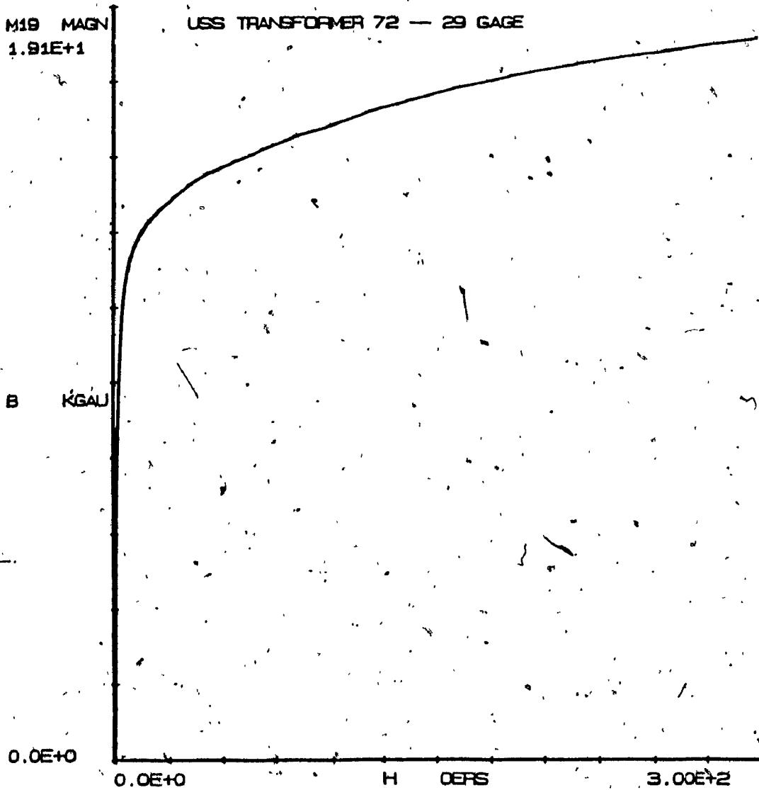
Fig. 6.8 B-H Curve used for 2D and 3D analysis
