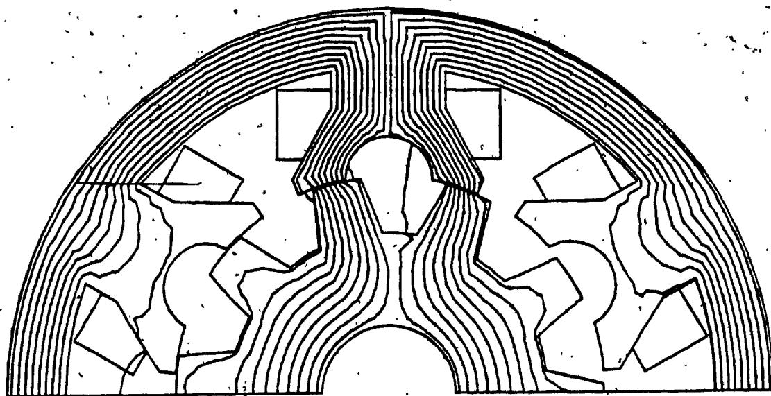
Fig. 3.19 Flux plot. Rotor pole axis at 4 degrees from the aligned position
