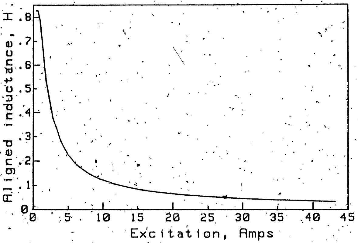
Fig. 5.4 Terminal inductance vs excitation
