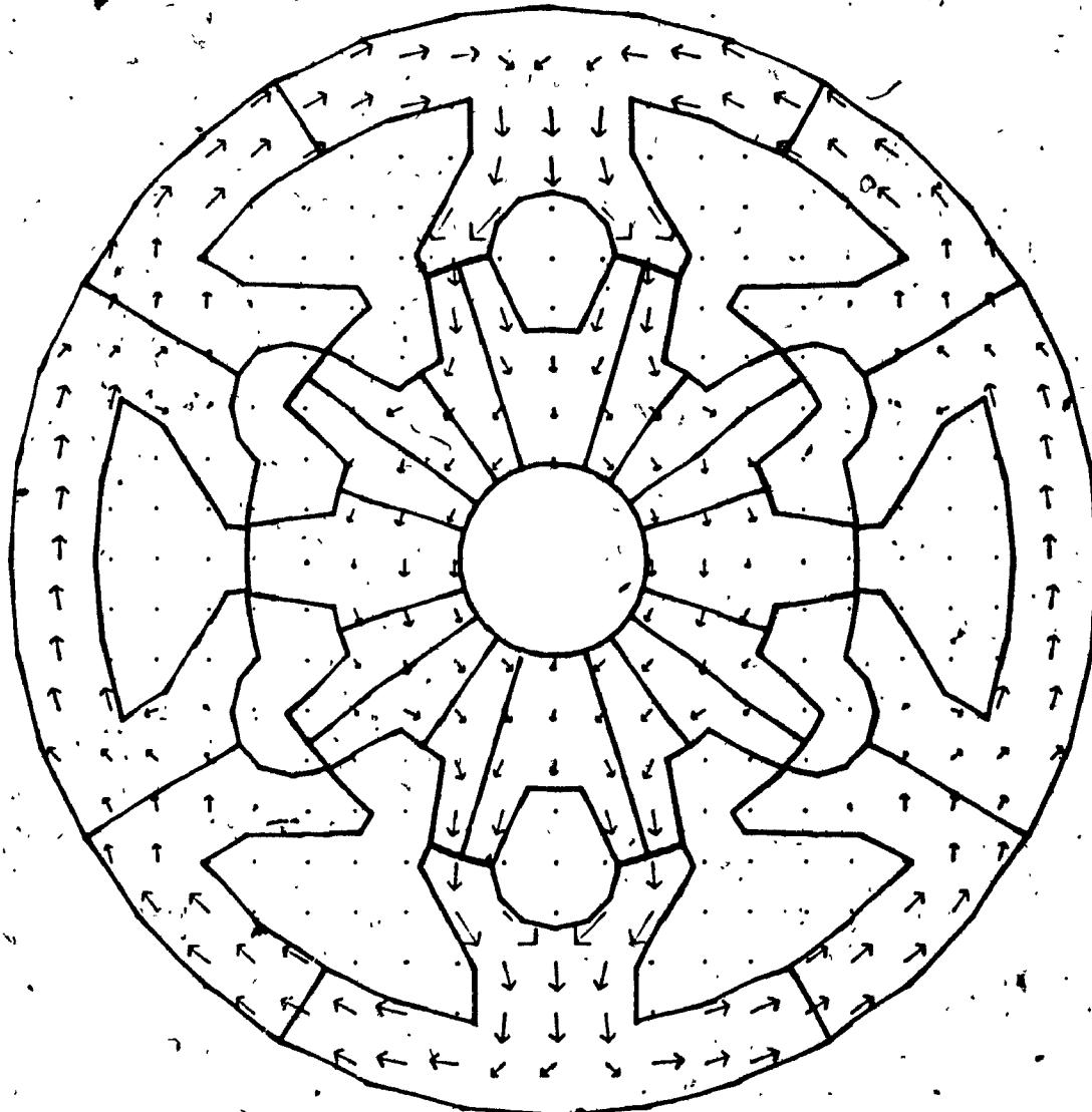
Fig. 6.10 Flux density plot for 3D solution
