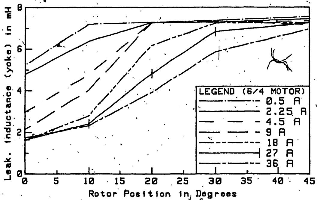
Fig. 3.12 Leakage inductance vs rotor position, due to leakage flux to yoke of one phase
