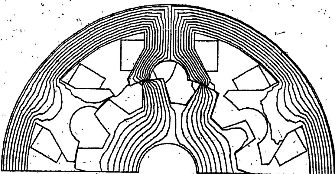
Fig. 3.20 Flux plot. Rotor pole axis at 8 degrees from the aligned position
