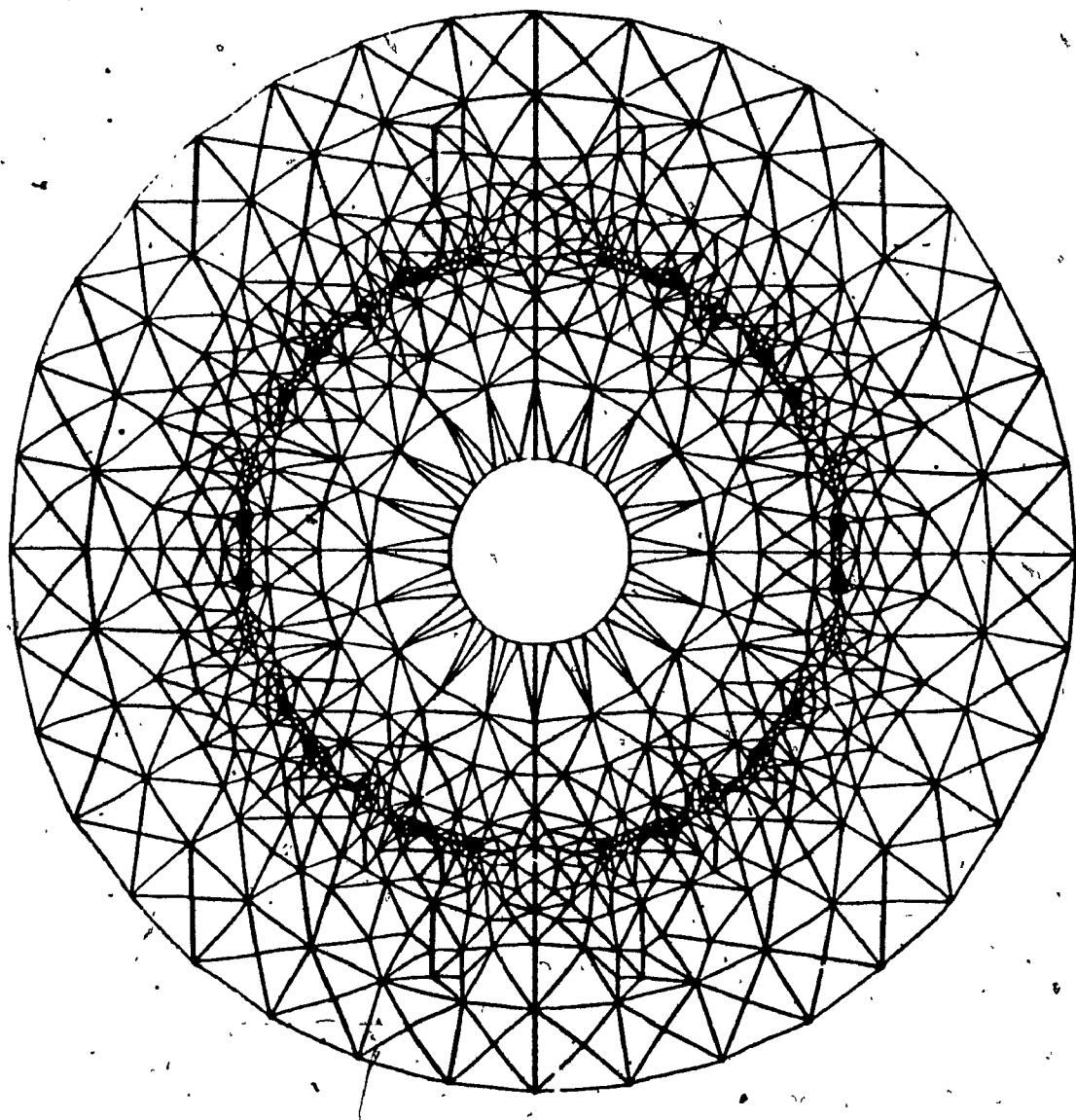
Fig. 6.2      2D Finite element mesh for aligned position
