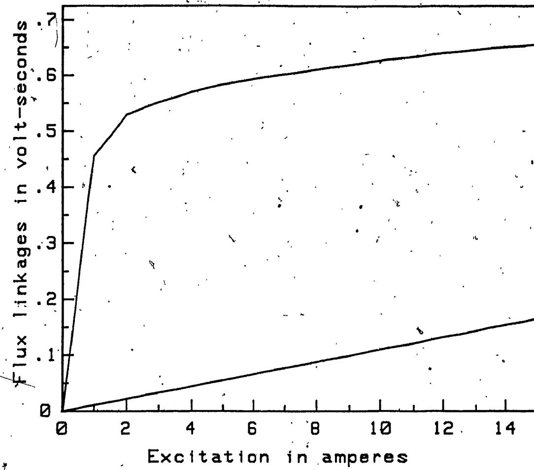
Fig. 4.1      Flux linkages vs excitation characteristic
