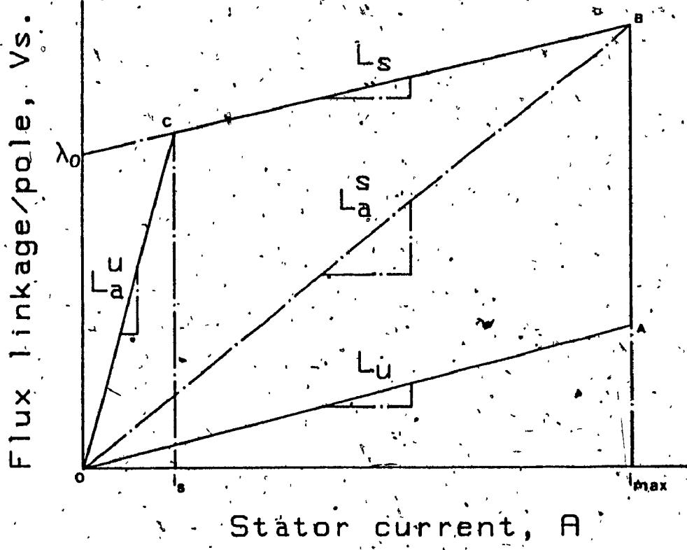
Fig. 5.2      Approximate flux linkages vs current characteristic
