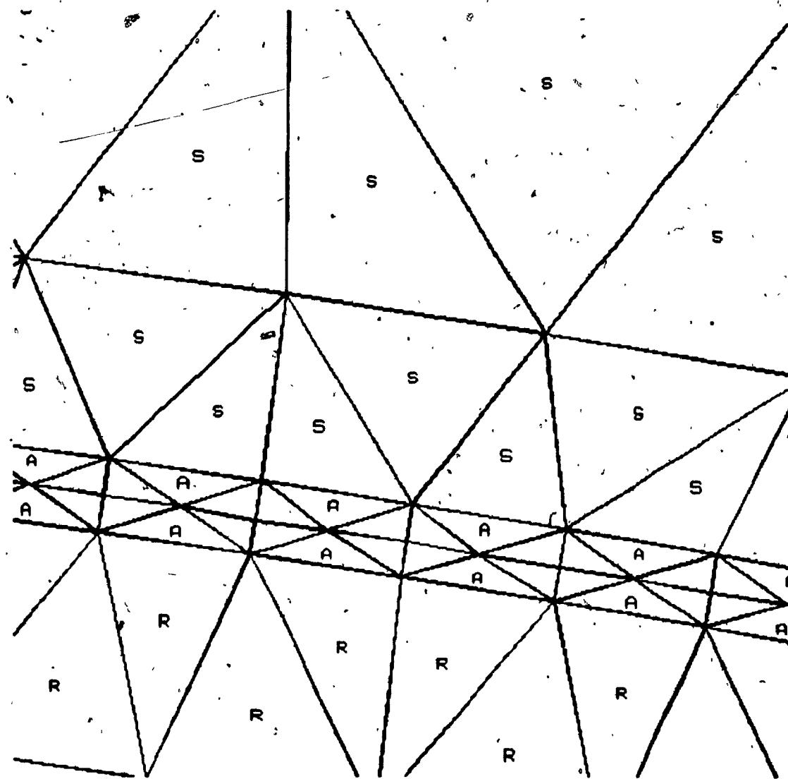
Fig. 2.4      Finite element subdivisions in the airgap region
