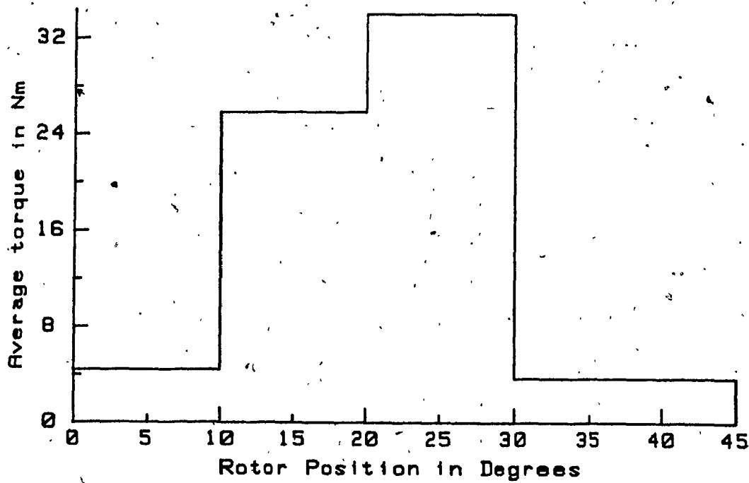
Fig. 3.14 Average torque vs rotor position for 9 A excitation
