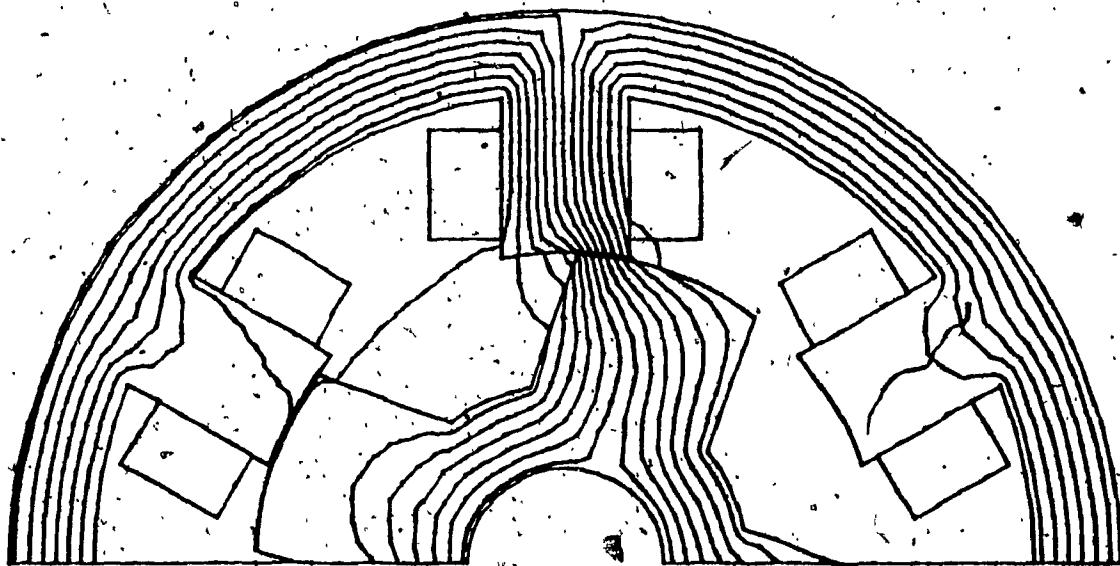
Fig. 3.8 Flux plot. Rotor pole axis at 20 degrees
