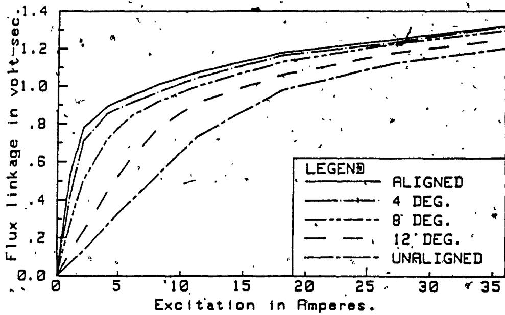
Fig. 3.22 Total flux linkages vs excitation of one pole winding
