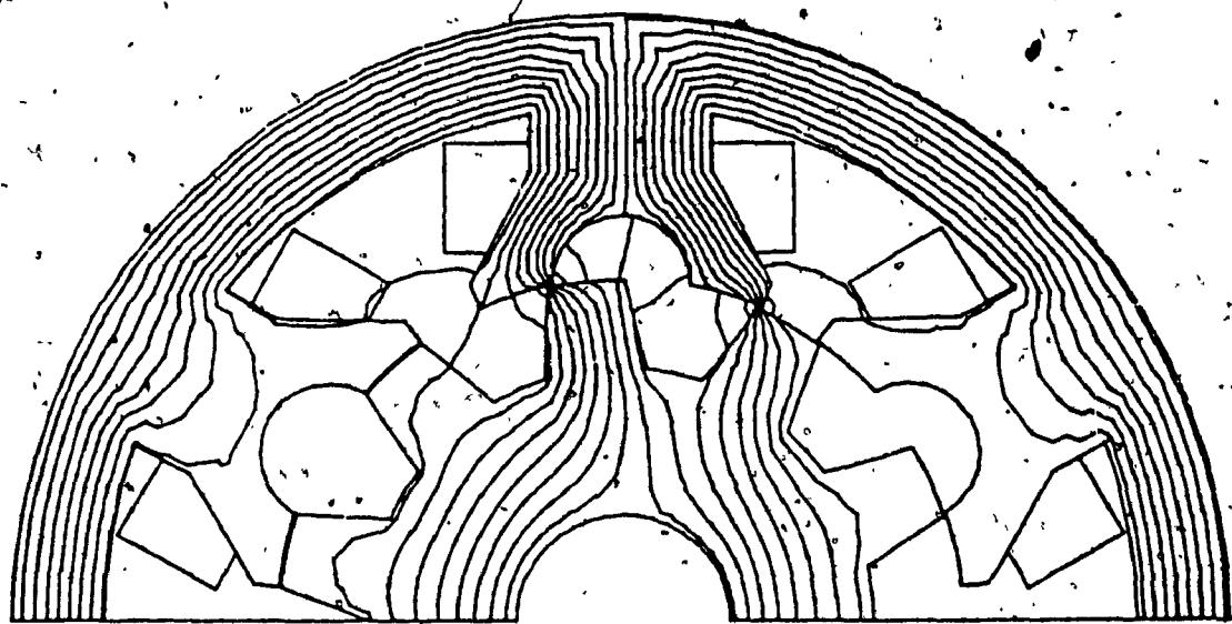
Fig. 3.21 Flux plot. Rotor pole axis at 12 degrees from the aligned position
