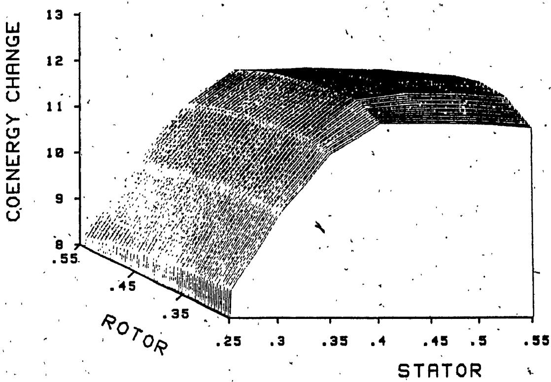
Fig. 4.7 Average torque vs pole arc/pole pitch ratios of stator
