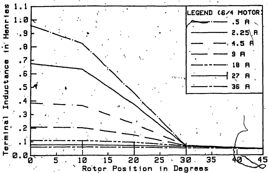
Fig. 3.11 Terminal inductance vs rotor position
