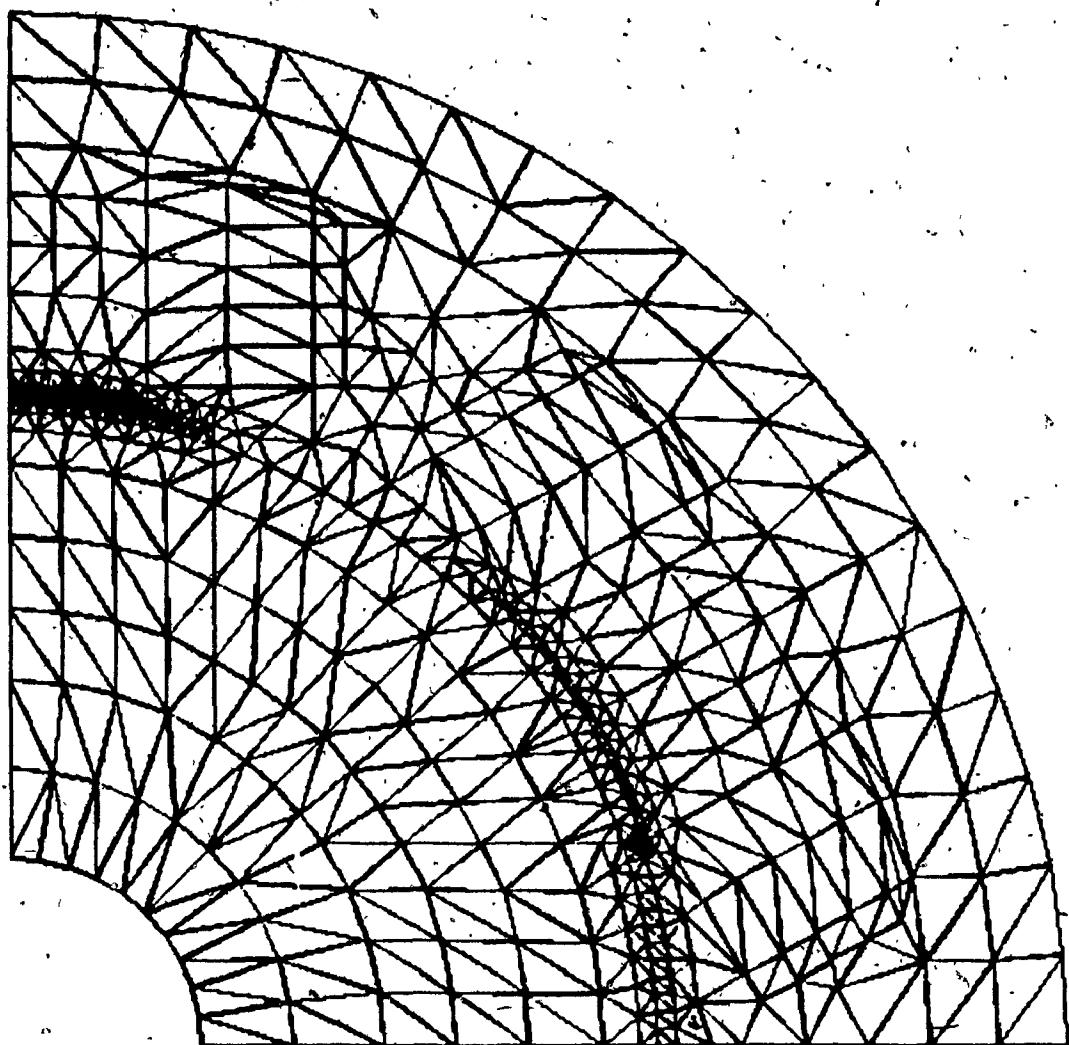
Fig. 2.2 Finite element subdivisions (6/4 motor)
