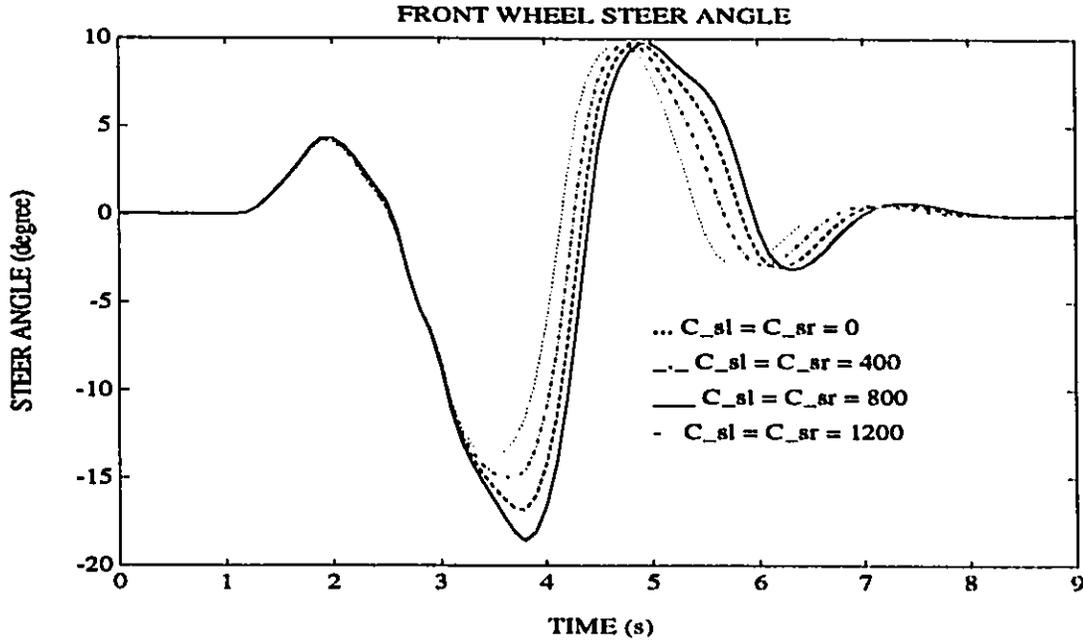
Figure 3.18: Front Wheel Steer Angle required to perform an Evasive Maneuver at 100 km/h
