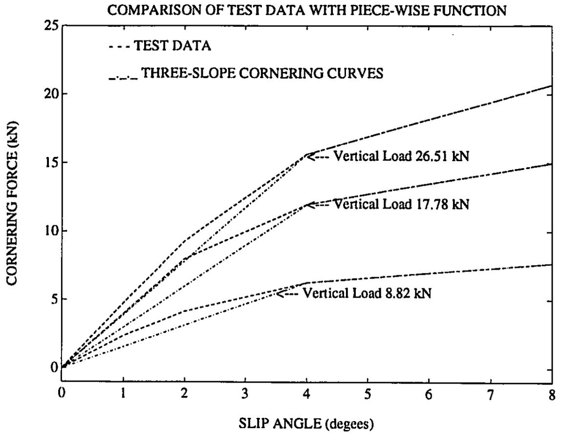
Figure 2.8: Cornering force of tire developed by Piecewise Linear Function
