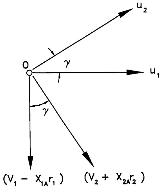
Figure 2.5: Forces and velocities at the articulation joint
