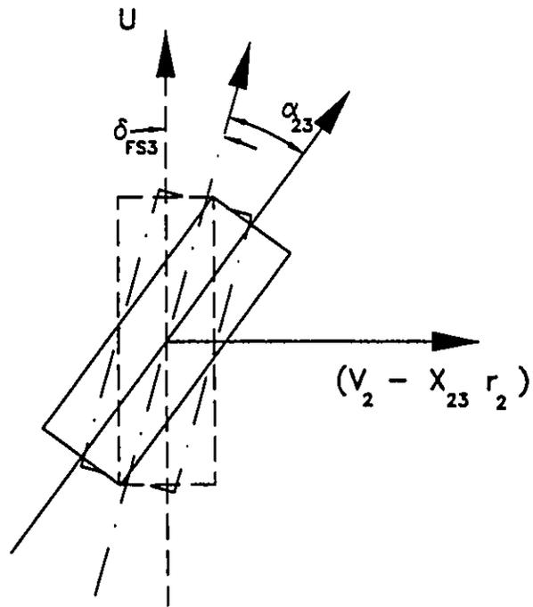
Figure 2.11: Force-steer and slip angles of tire on axle 23
