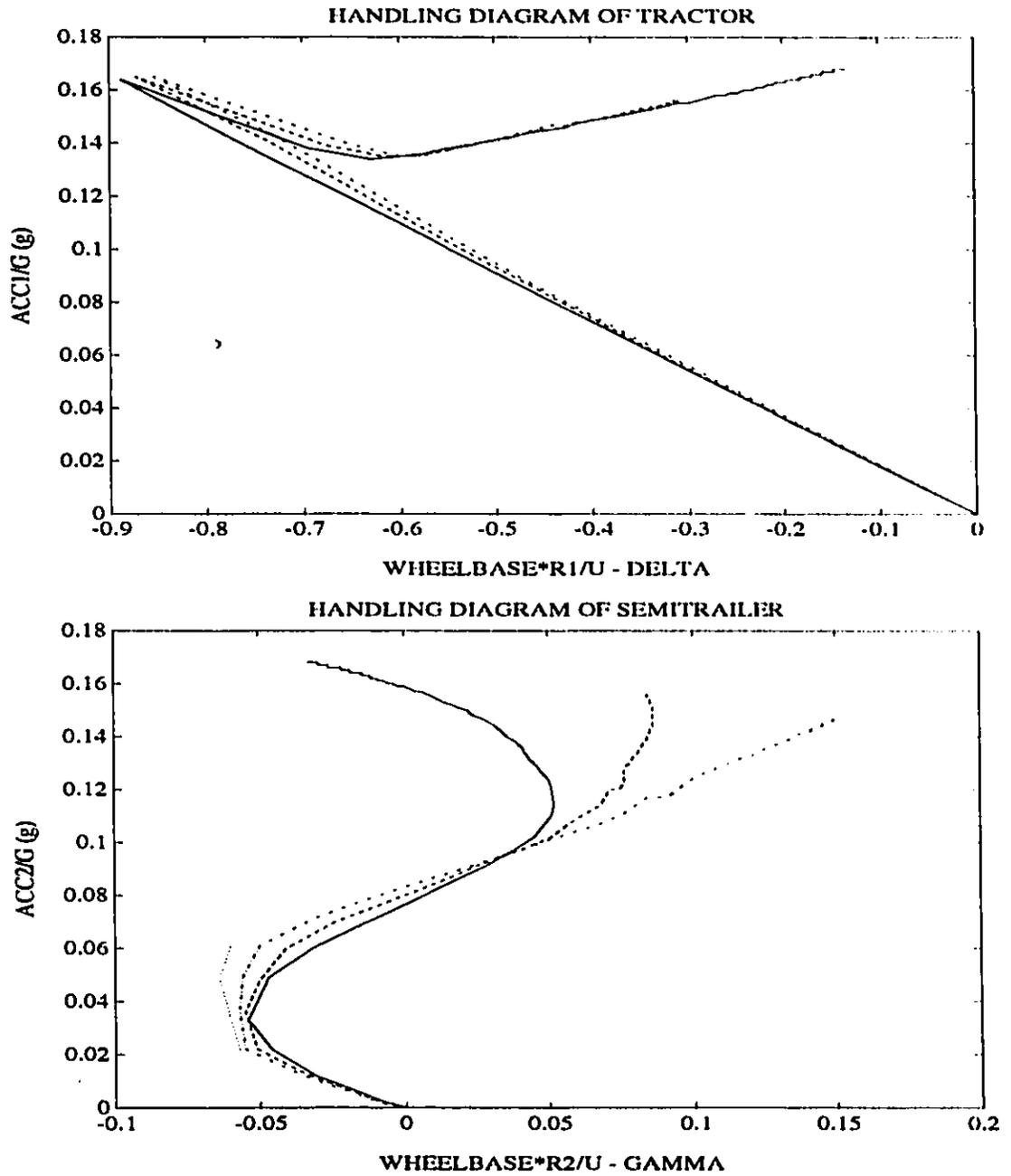
Figure 3.10: Handling Diagrams of Tractor and Semitrailer under a Constant Steer Maneuver at 50 km/h
