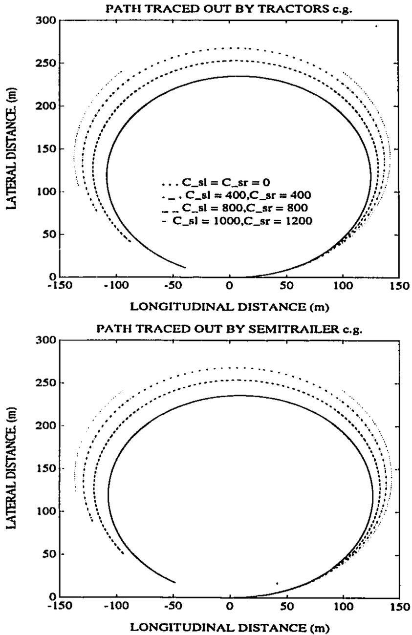
Figure 3.5: Path traced by the Tractor and Semitrailer under a Constant Steer input at 50 km/h
