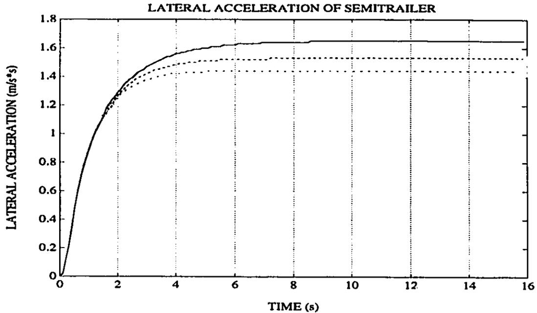
Figure 3.7: Lateral Acceleration Response of the Semitrailer under a Constant Steer Maneuver at 50 km/h
