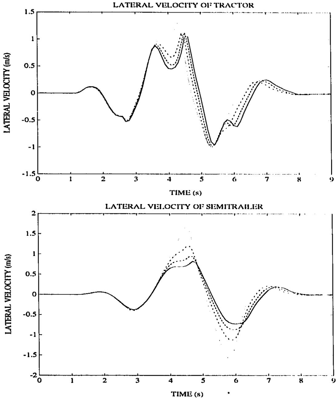
Figure 3.20: Lateral Velocity Response of Tractor and Semitrailer for an Evasive Manuever at 100 km/h
