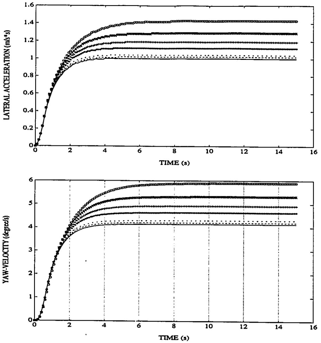
Figure 3.4: Lateral Acceleration and Yaw-Velocity response, for different locations for Axle 21 at 50 km/h
