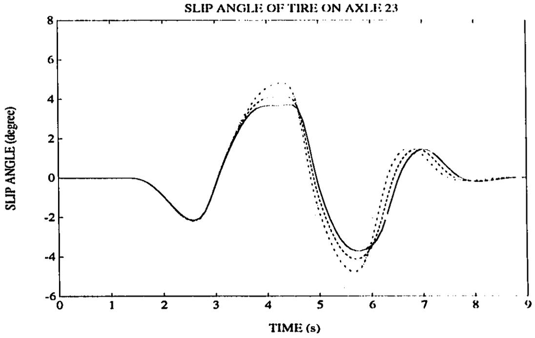
Figure 3.26: Side-Slip Angles of tires on Axles 22 and 23 of Articulated vehicle for an Evasive Maneuver at 100 km/h
