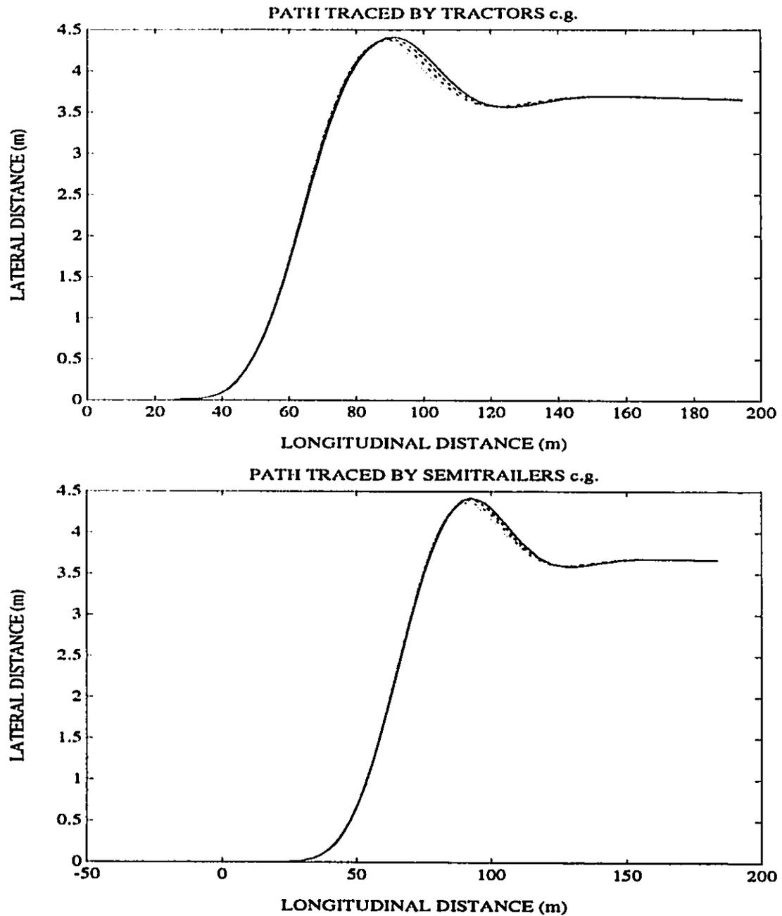
Figure 3.15: Path followed by the Tractor and Semitrailer c.g.s for a Lane-Change Maneuver at 100 km/h
