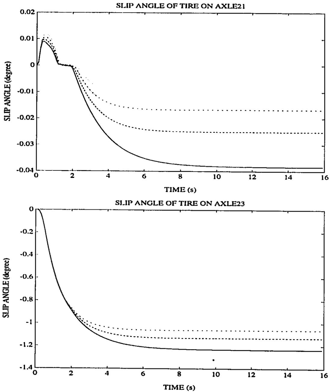
Figure 3.9: Side-Slip Angle response of axle 21 and 23 under a Constant Steer Maneuver at 50 km/h
