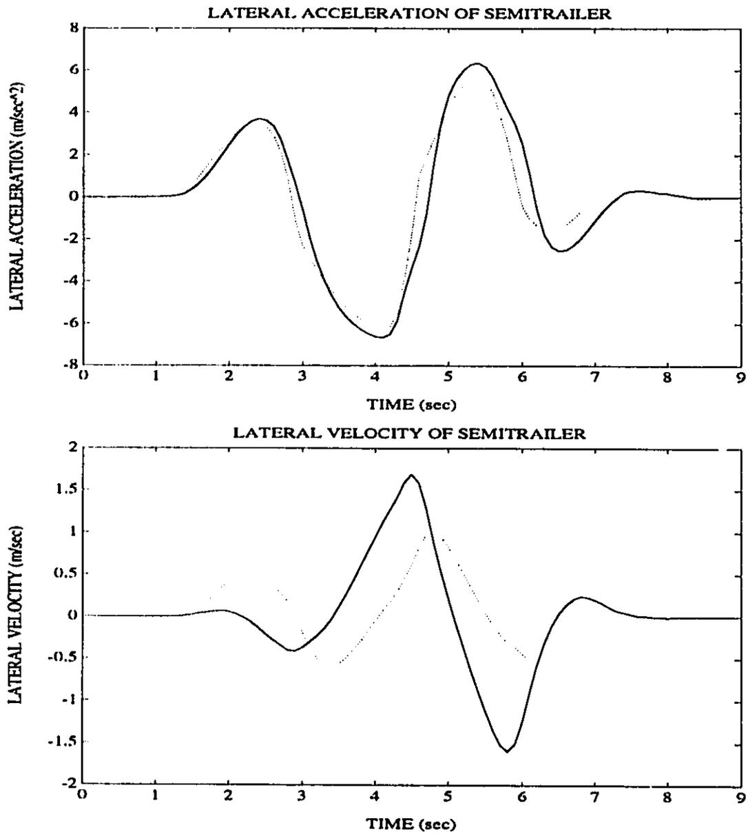
Figure 4.36: SCHEME IV: Transient Response of lateral acceleration and Lateral Velocity of Semitrailer for an Evasive Maneuver at 100 km/h
