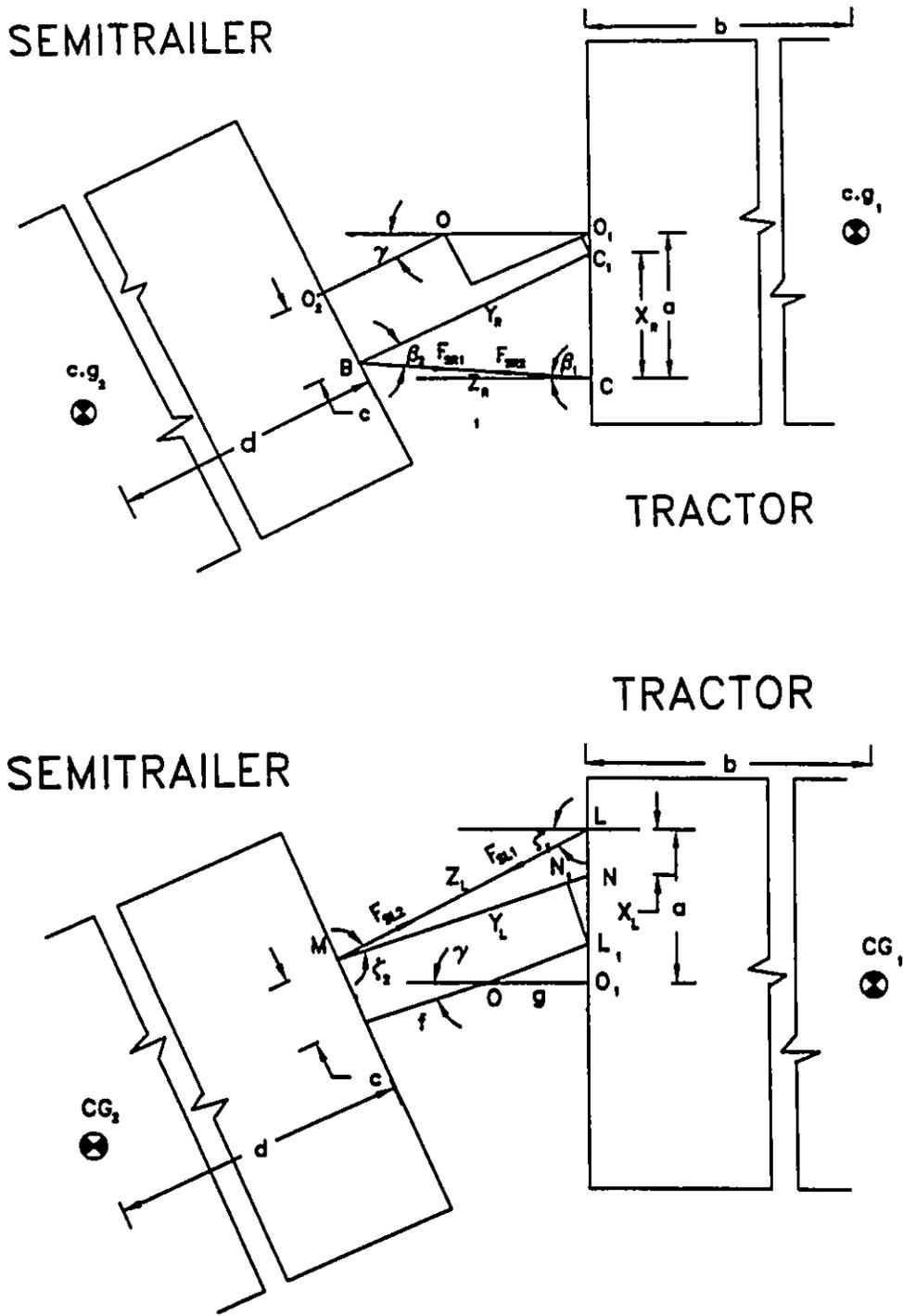
Figure 2.3: Kinematic model of the articulation damper and damper forces acting on the two units
