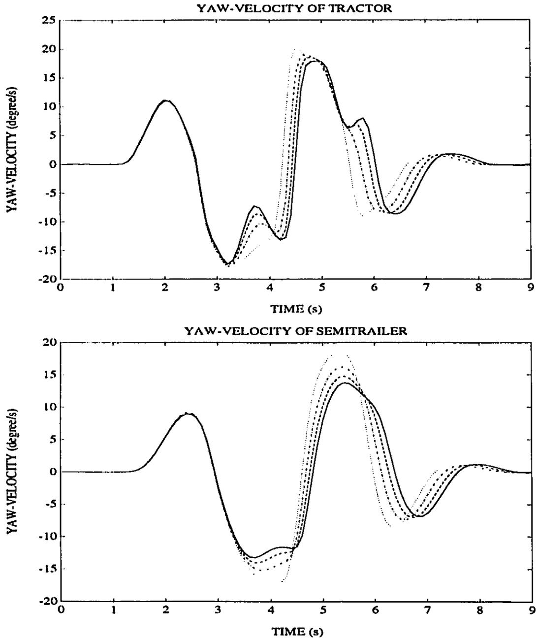
Figure 3.21: Yaw-Velocity Response of Tractor and Semitrailer for an Evasive Maneuver at 100 km/h
