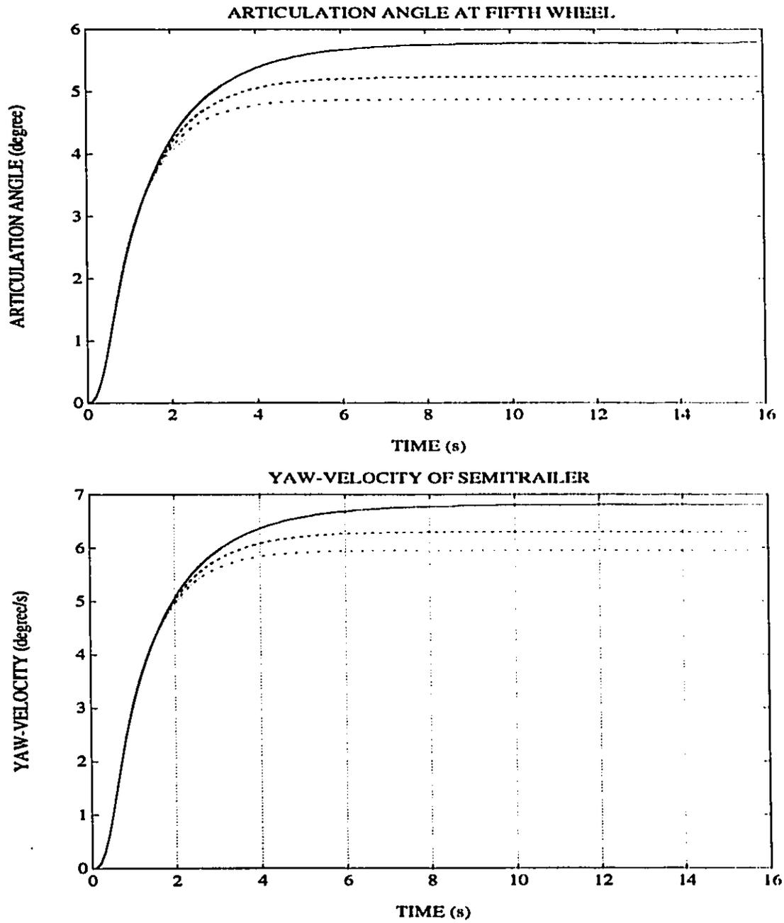
Figure 3.6: Articulation angle and Yaw Velocity response of the semitrailer under a Constant Steer Maneuver at 50 km/h
