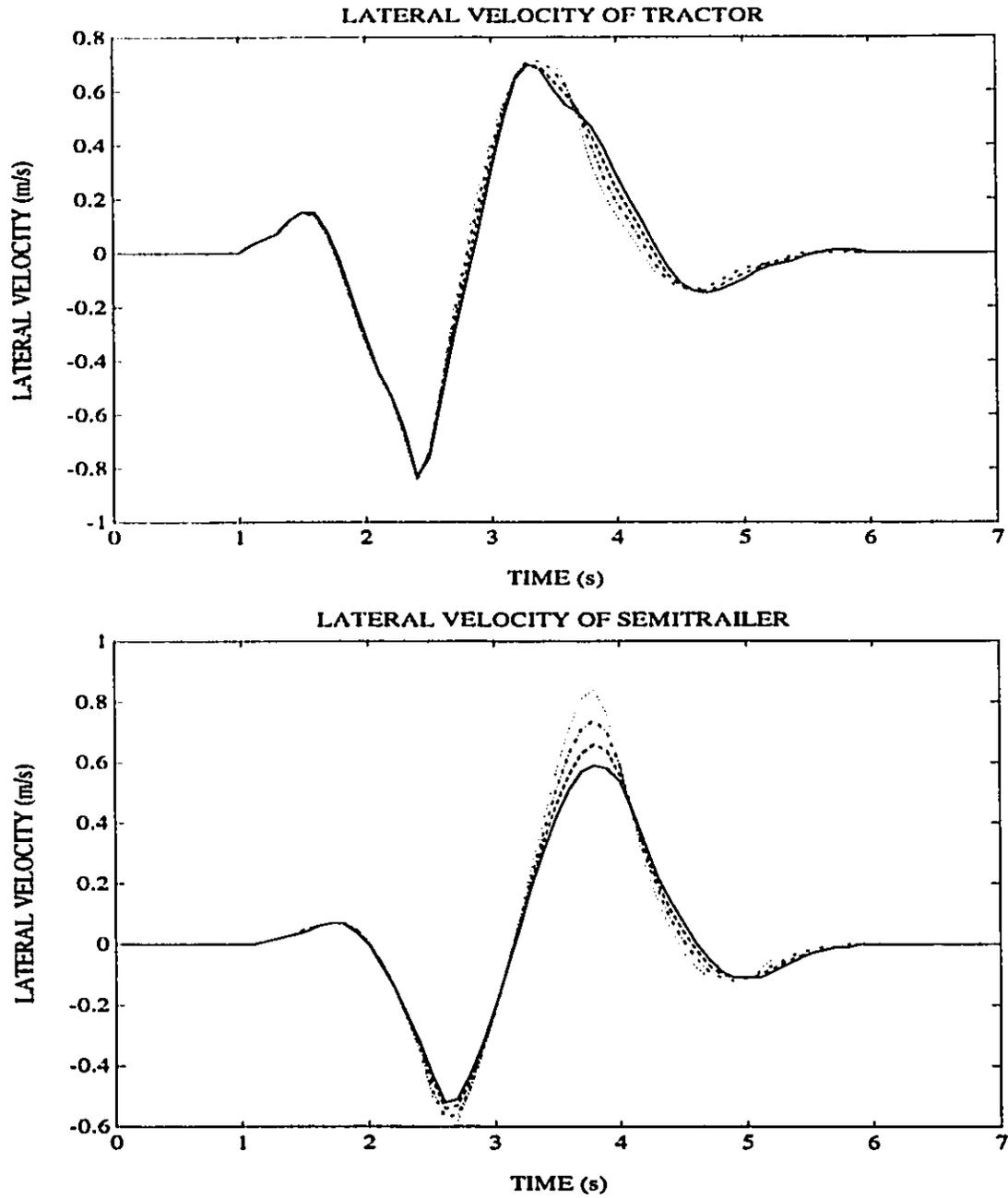
Figure 3.13: Lateral Velocity Response of Tractor and Semitrailer for a Lane-Change Maneuver at 100 km/h
