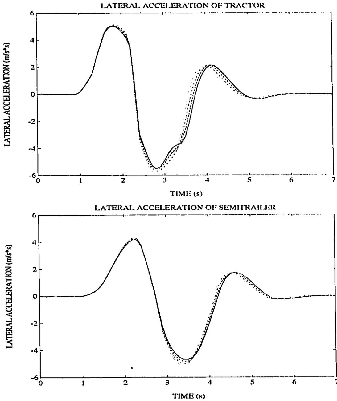
Figure 3.12: Lateral Acceleration Response of Tractor and Semitrailer for a Lane-Change Maneuver at 100 km/h
