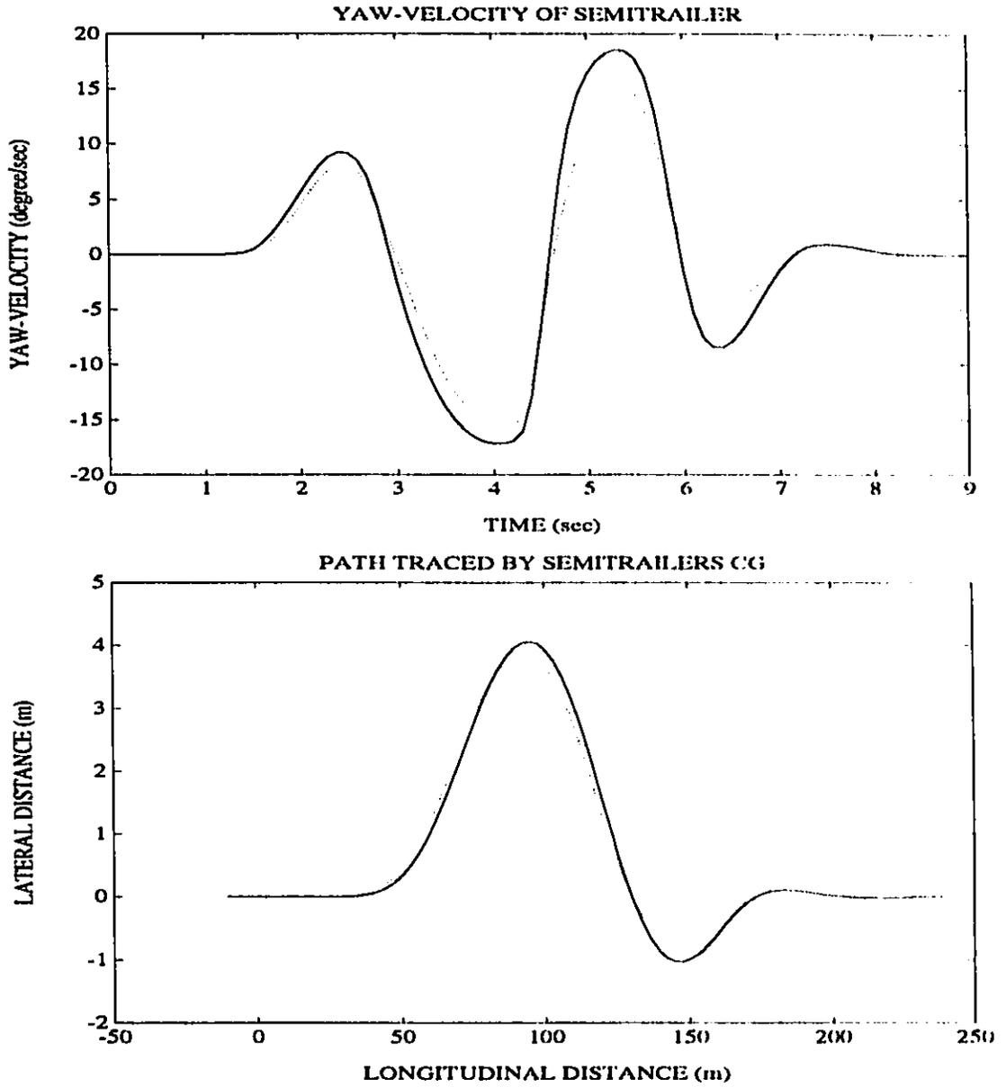
Figure 4.37: SCHEME IV: Transient Response of Yaw-Velocity and path and over-shoot made by Semitrailer for an Evasive Maneuver at 100 km/h
