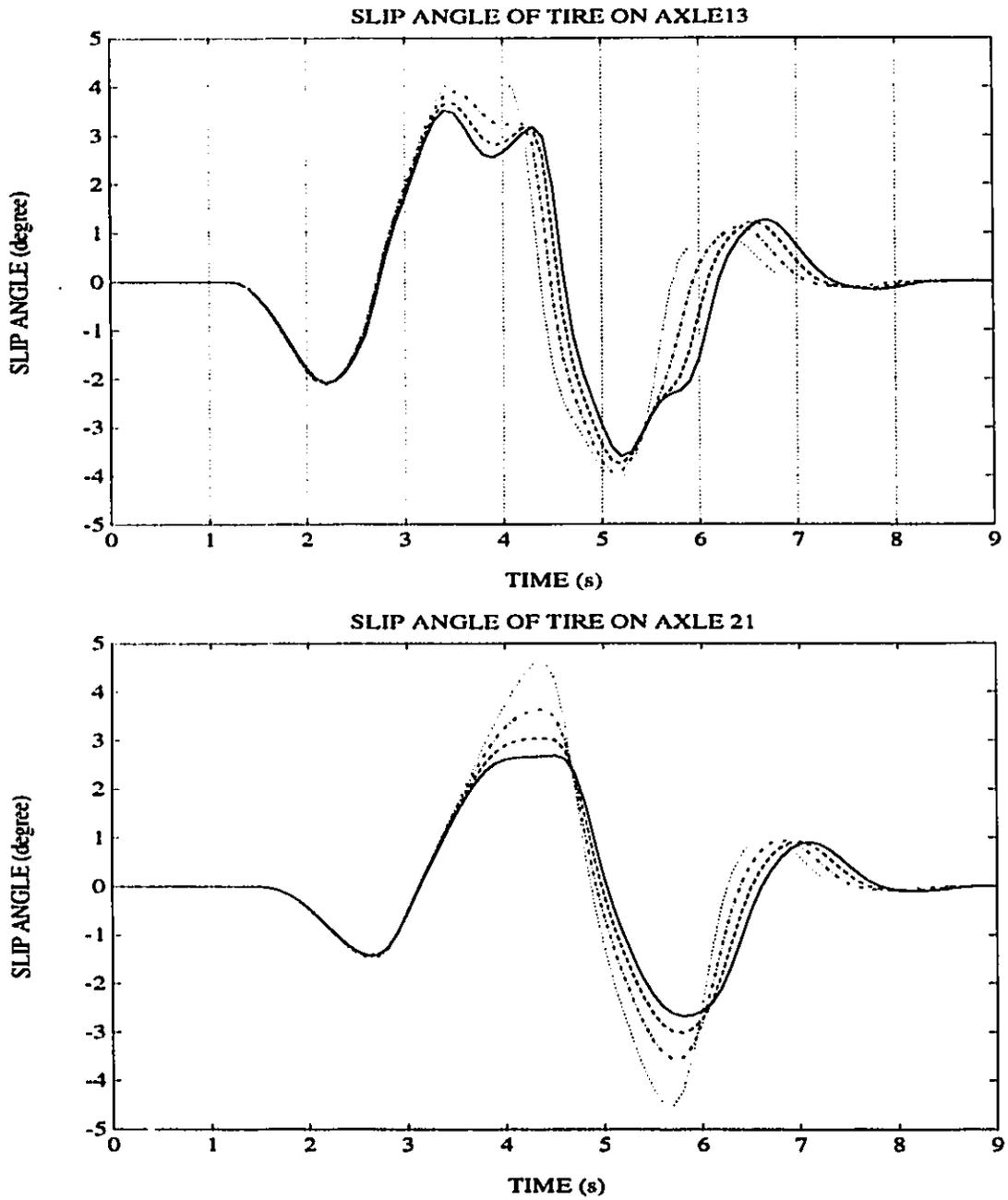
Figure 3.25: Side-Slip Angles of tires on Axles 13 and 21 of Articulated vehicle for an Evasive Maneuver at 100 km/h
