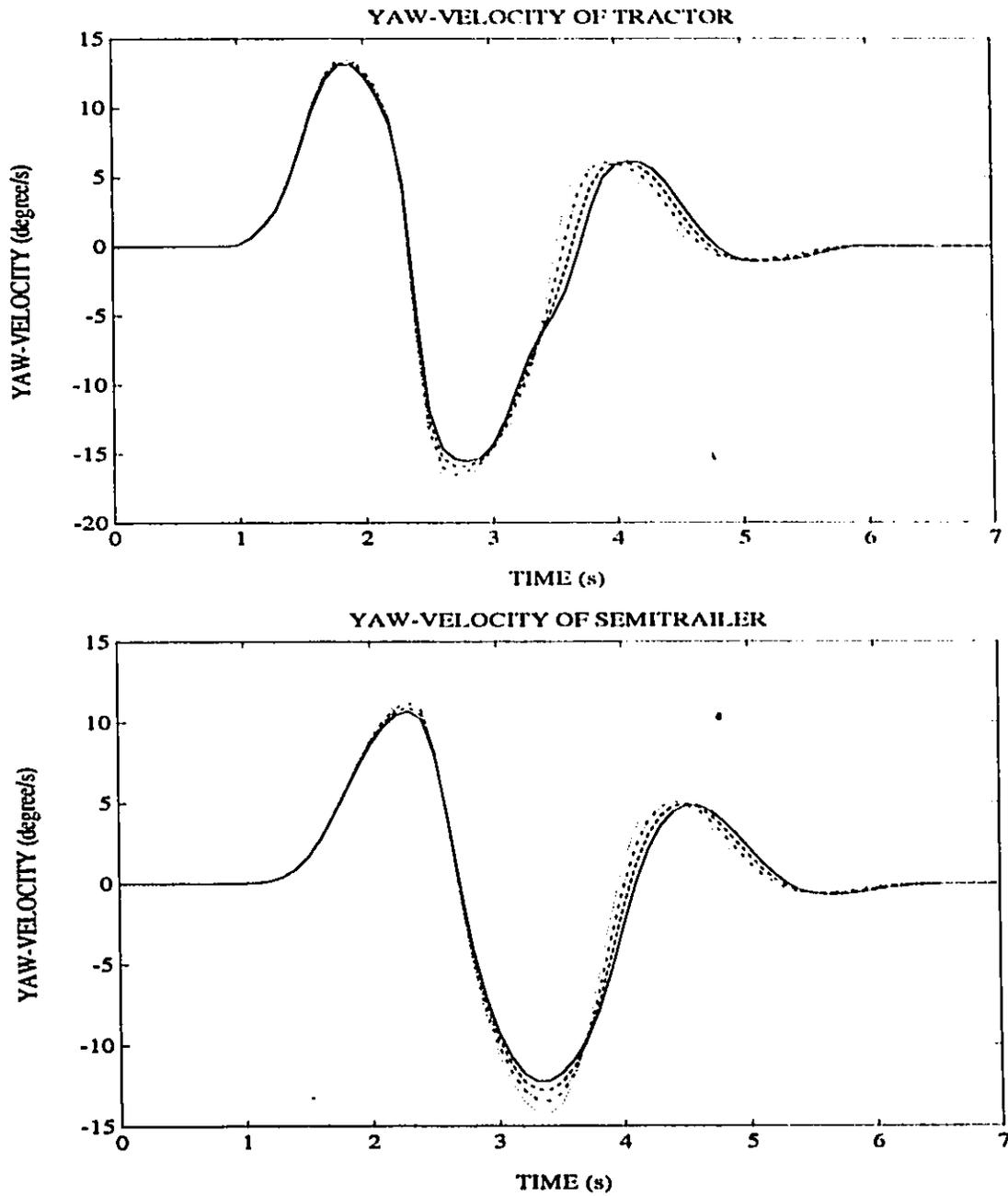
Figure 3.14: Yaw-Velocity Response of Tractor and Semitrailer for a Lane-Change Maneuver at 100 km/h
