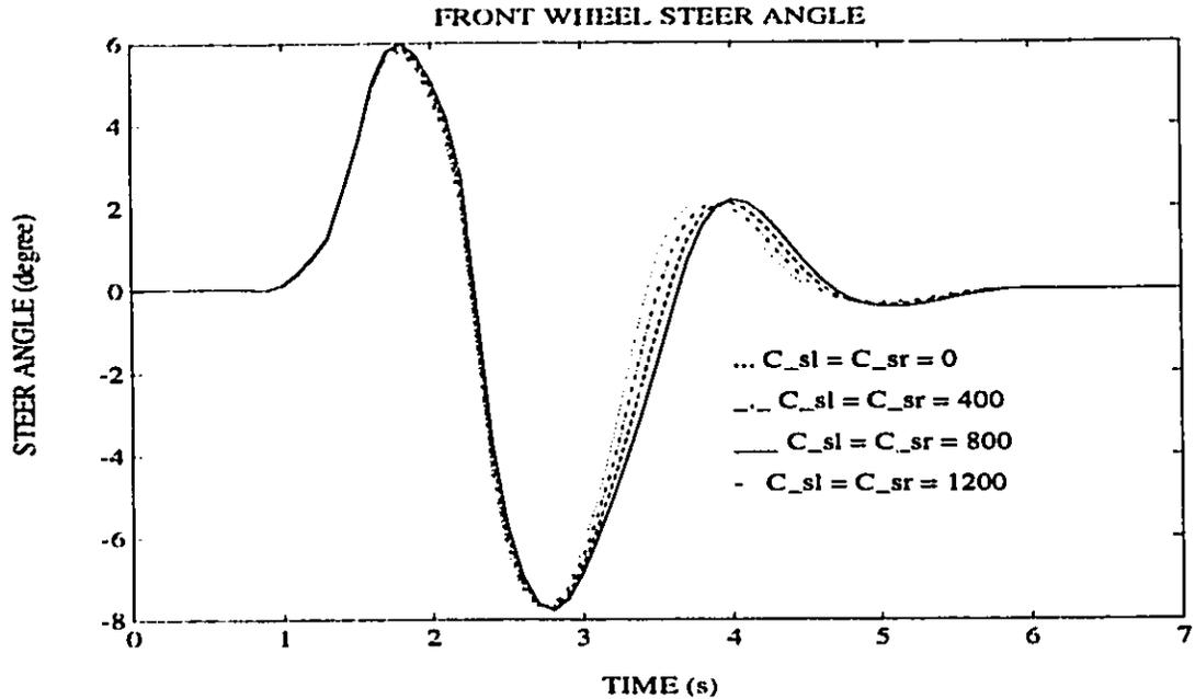
Figure 3.11: Front Wheel Steer Angle Required to negotiate a Lane-Change Maneuver at 100 km/h
