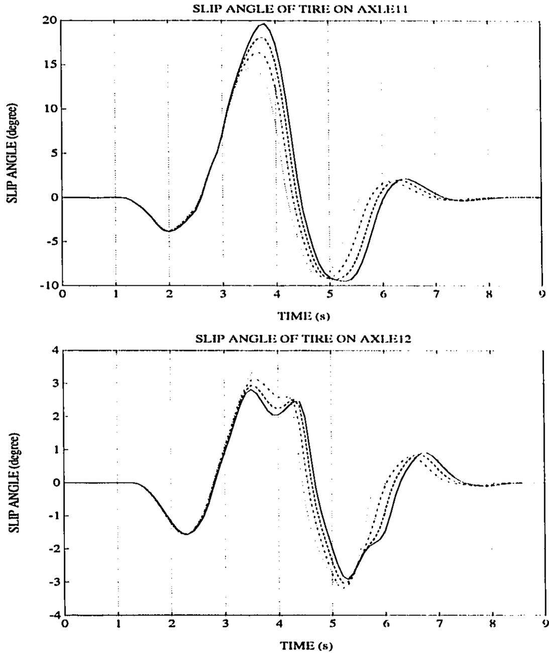
Figure 3.24: Side-Slip Angles of tires on Axles 11 and 12 of Articulated vehicle for an Evasive Maneuver at 100 km/h
