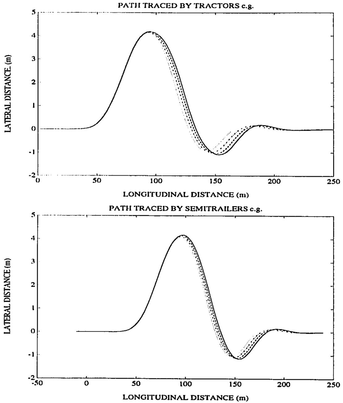
Figure 3.23: Path followed by the Tractor and Semitrailer for an Evasive Maneuver at 100 km/h
