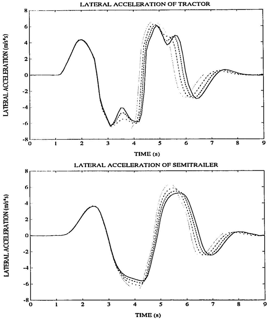
Figure 3.19: Lateral Acceleration Response of Tractor and Semitrailer for an Evasive Maneuver at 100 km/h
