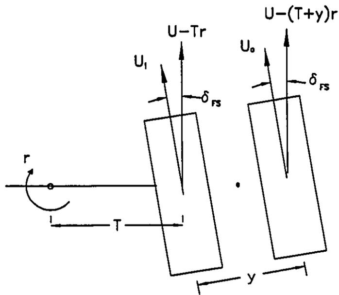
Figure 2.12: The forward velocities of the steered dual tire set
