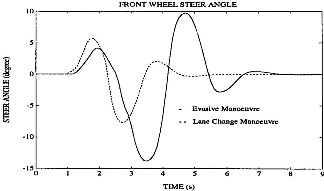
Figure 3.3: Front Wheel Steer Angle for Lane-change and Evasive Maneuvers at 100 km/h
