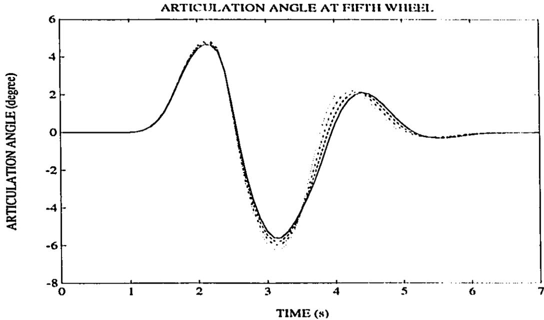
Figure 3.16: Articulation Angle Response of Vehicle for a Lane-Change Maneuver at 100 km/h
