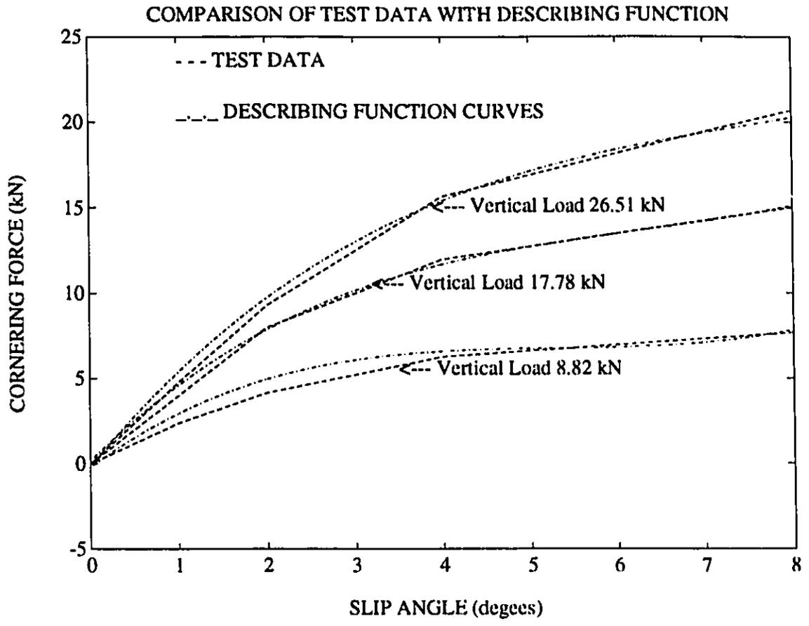
Figure 2.9: Cornering force of tire developed by Continuous Describing Function
