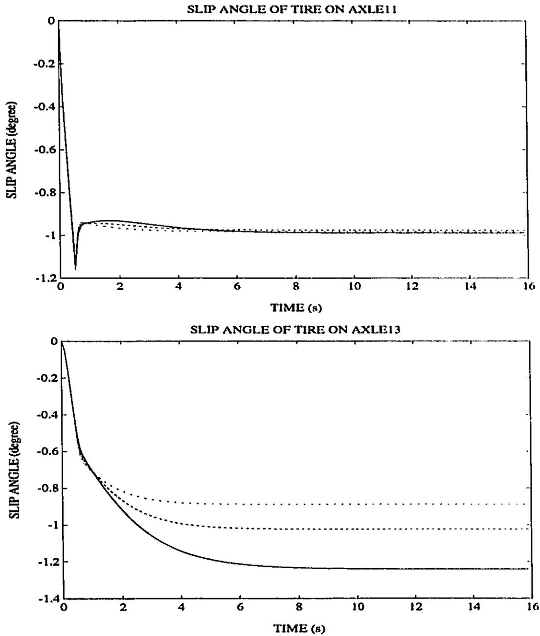
Figure 3.8: Side-Slip Angle response of axle 11 and 13 under a Constant Steer Maneuver at 50 km/h
