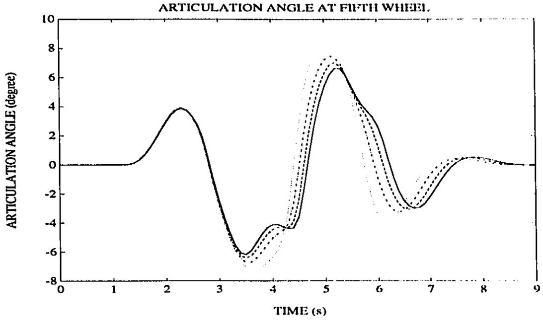
Figure 3.22: Articulation Angle Response of Vehicle for an Evasive Maneuver at 100 km/h
