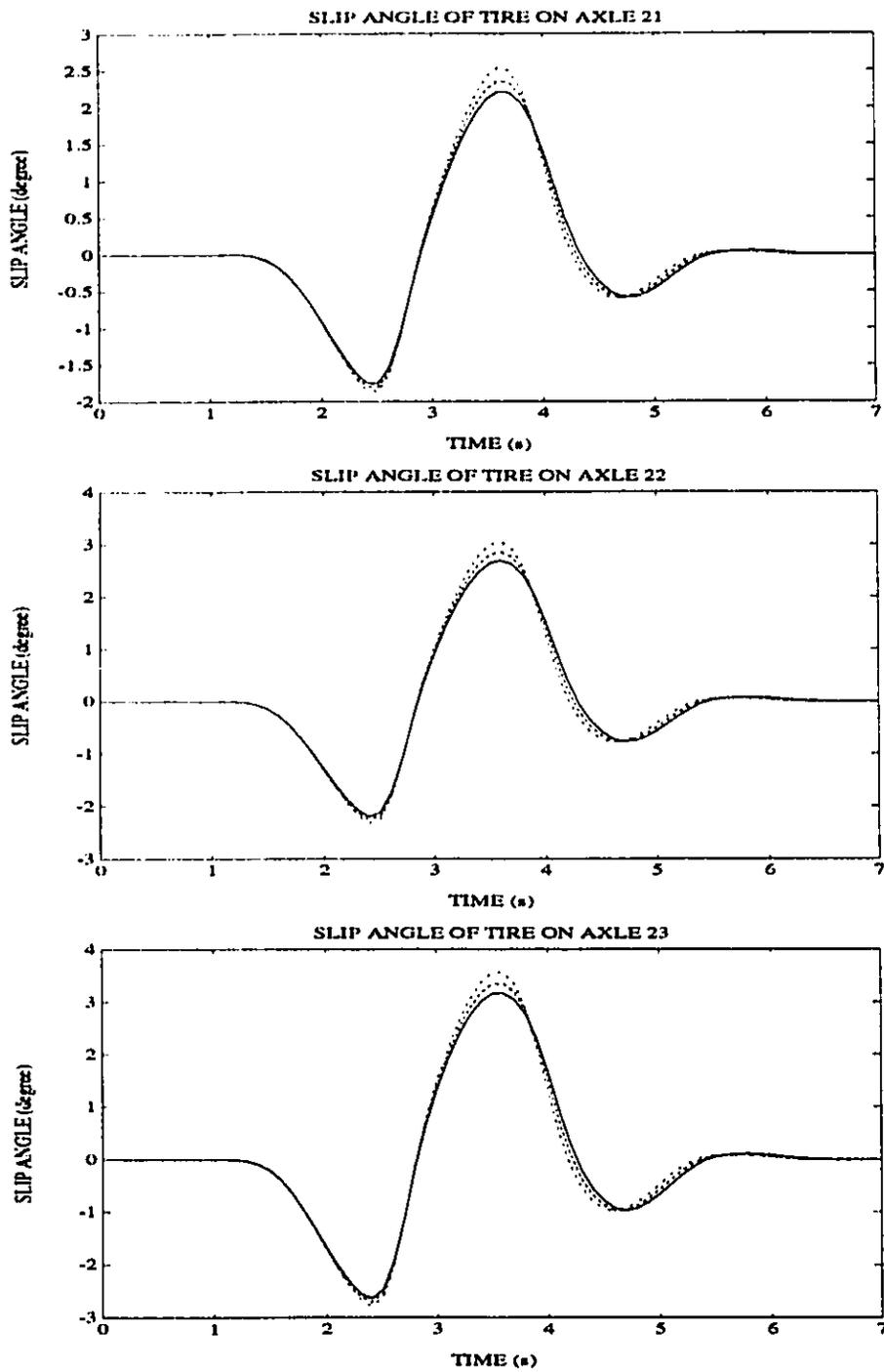
Figure 3.17: Side-Slip Angles of tires on Semitrailer during a Lane-Change Maneuver at 100 km/h
