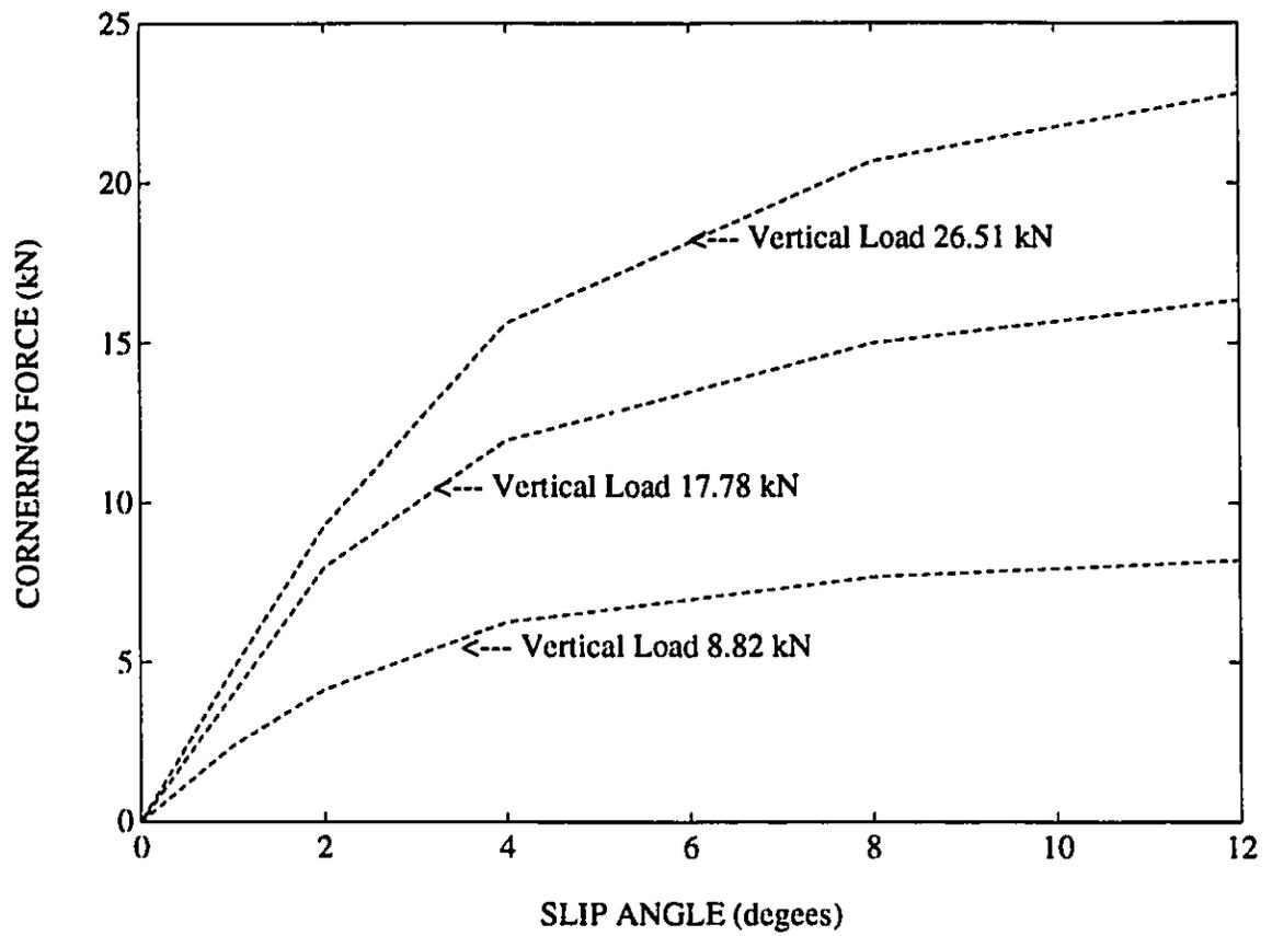
Figure 2.7: Cornering force characteristics of an 11R22.5 Radial tire
