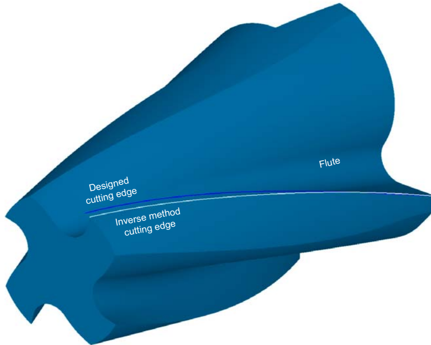
Figure 3.12: Ground tapered flat end-mill using the inverse method simulation.
