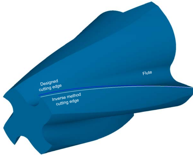
Figure 5.13: The simulation model of the tapered end-mill with the machined flutes by using the inverse method.
