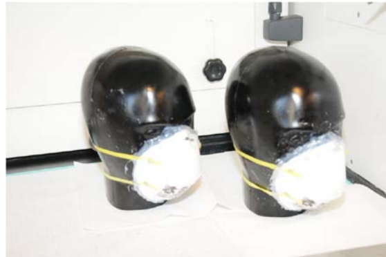
Figure 1. Sealed N95 FFR on the manikin head.
