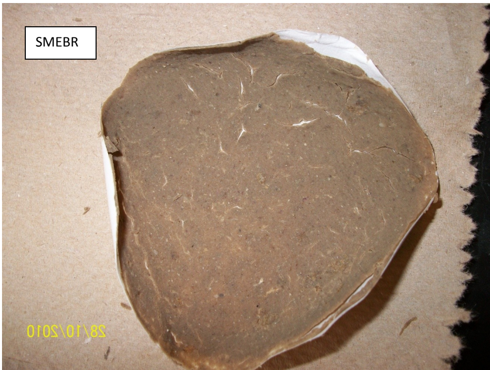
Figure 9.34: Photos of SMEBR and MBR sludge after vacuum filtration
