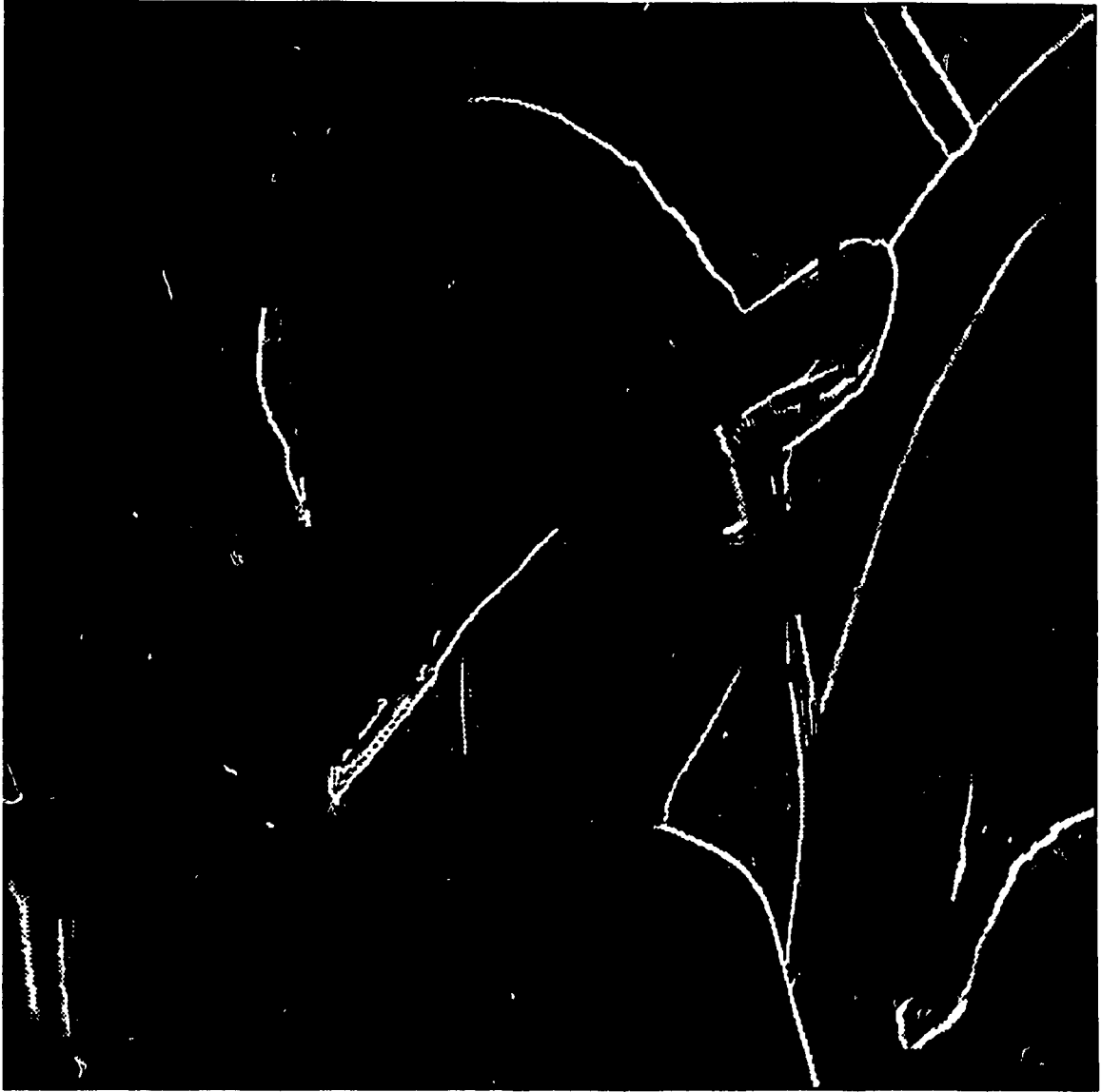
Figure 3.15: Sobel Masked Image of the Sharp Edge Blocks after the Continuity Test
