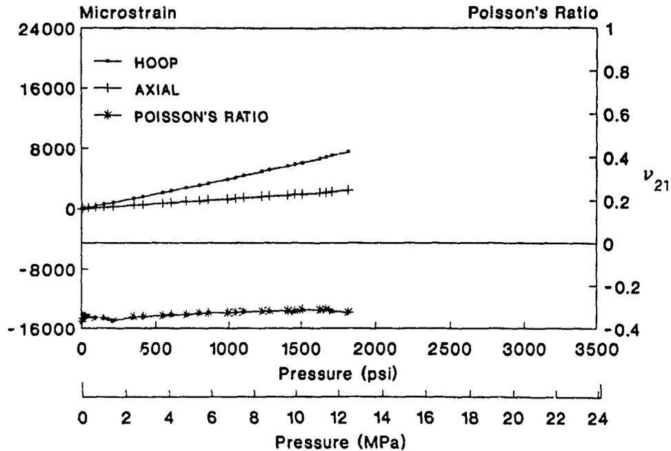
Fig. 6-32: Strain and Poisson's ratio versus pressure graph for veil lined tube 1E-2G.
