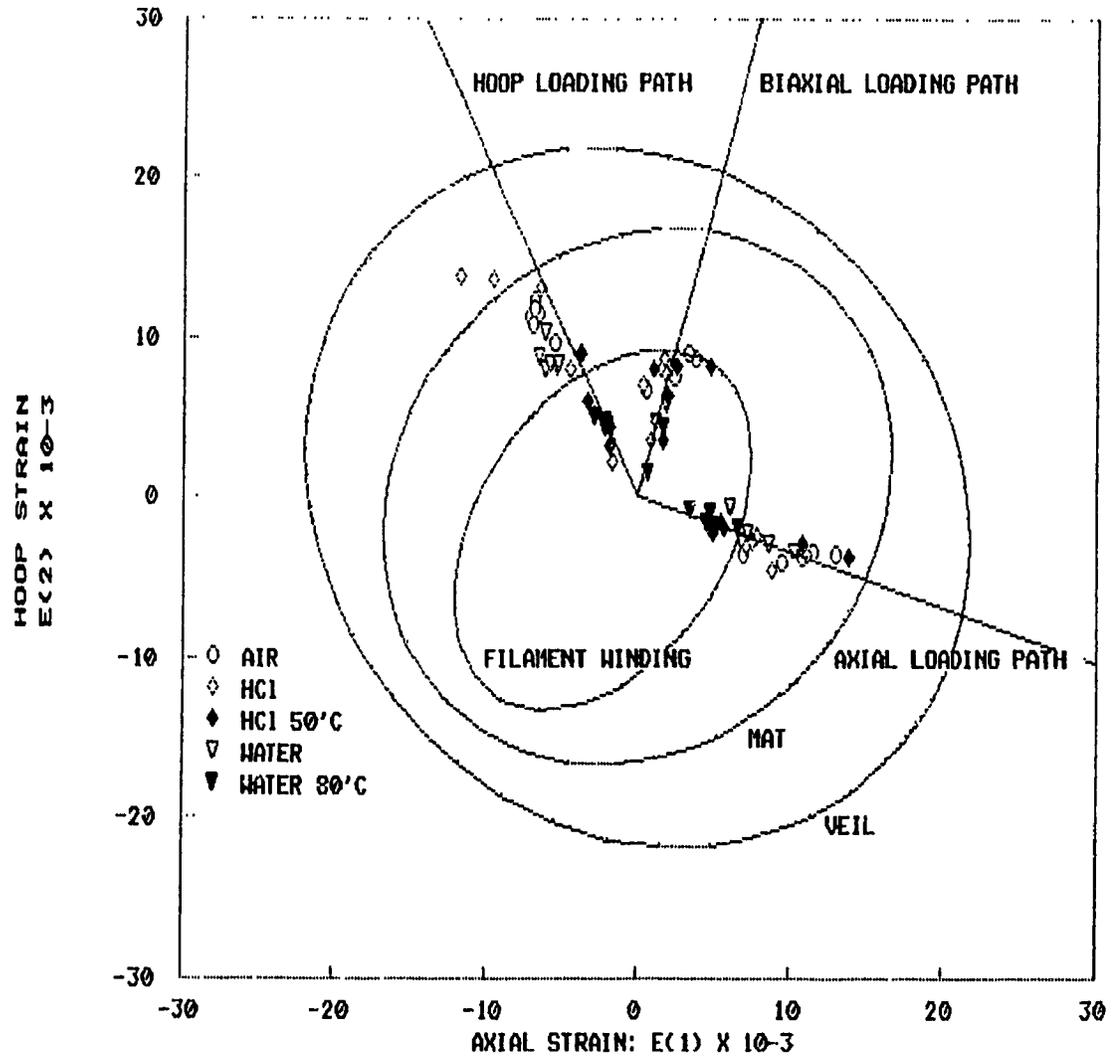
Fig. 7-25: Experimental results plotted onto the theoretical failure envelopes and loading paths in strain space, veil lined tubes.
