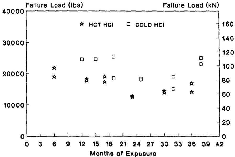
Fig. 7-9: Axial test failure load versus exposure time, veil lined tubes exposed to hot and cold HCl.
