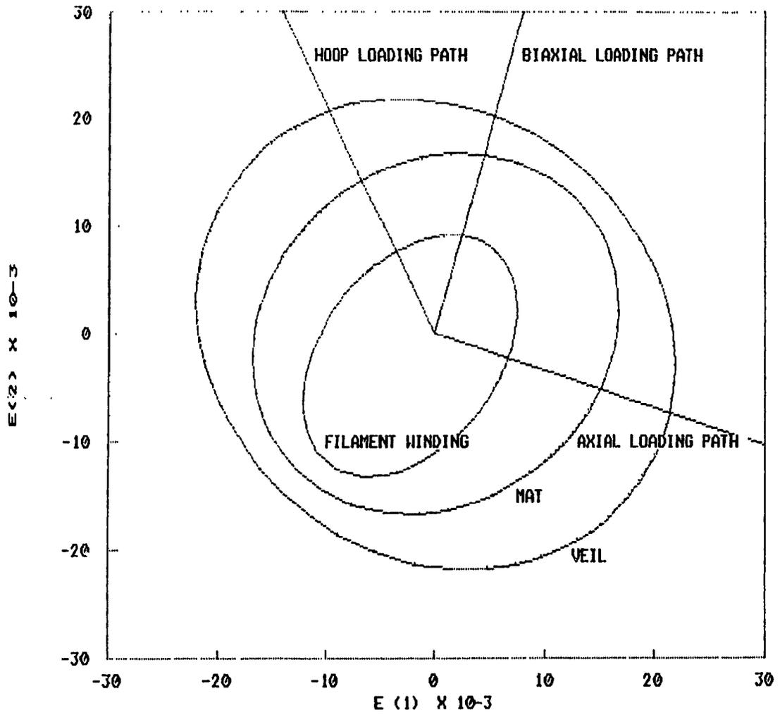
Fig. 4-11: Failure envelopes and loading paths in strain space.
