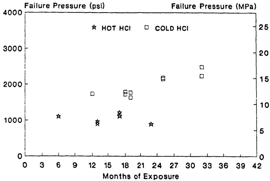
Fig. 7-17: Biaxial test failure pressure versus exposure time, PVC lined tubes exposed to hot and cold HCl.
