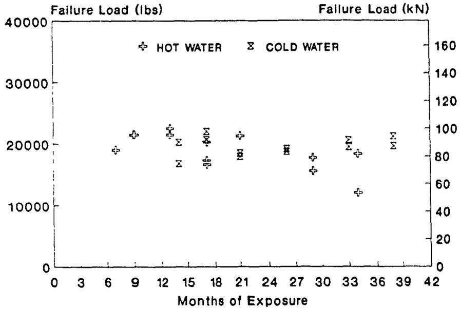
Fig. 7-15: Axial test failure load versus exposure time, PVC lined tubes exposed to hot and cold water.
