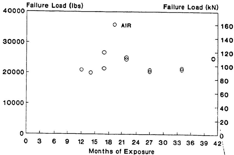
Fig. 7-3: Axial test failure load versus exposure time, veil lined tubes exposed to air.
