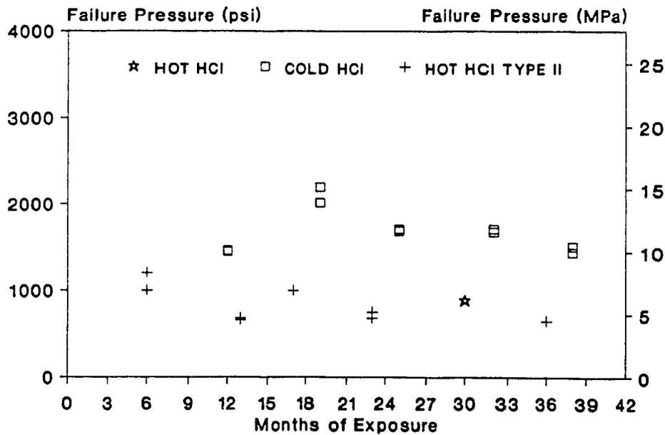
Fig. 7-7: Hoop test failure pressure versus exposure time, veil lined tubes exposed to hot and cold HCl.
