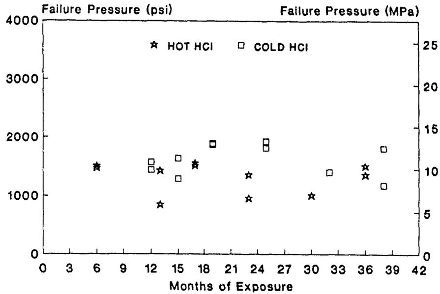
Fig. 7-8: Biaxial test failure pressure versus exposure time, veil lined tubes exposed to hot and cold HCl.
