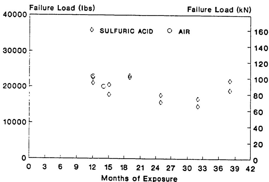
Fig. 7-21: Axial test failure load versus exposure time, PVC lined tubes exposed to sulfuric acid and air.
