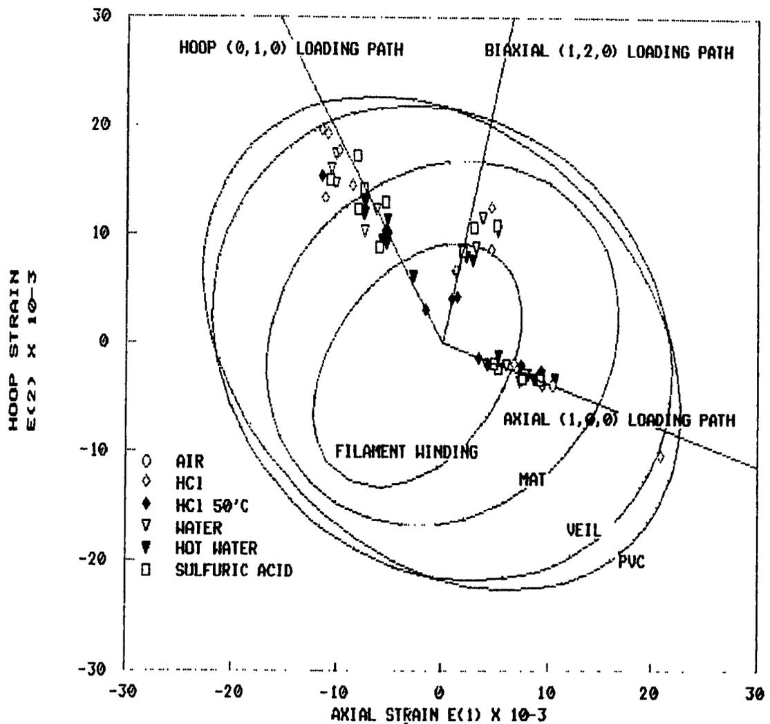
Fig. 7-29: Experimental results plotted onto the theoretical failure envelopes and loading paths in strain space, PVC lined tubes.
