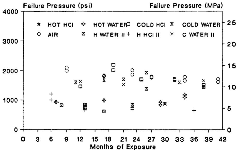
Fig. 7-10: Hoop test failure pressure versus exposure time, veil lined tubes, all environments.
