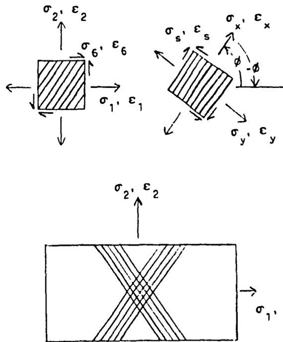
Fig. 4-1: Sign conventions for stress, strain and angle of transformation.
