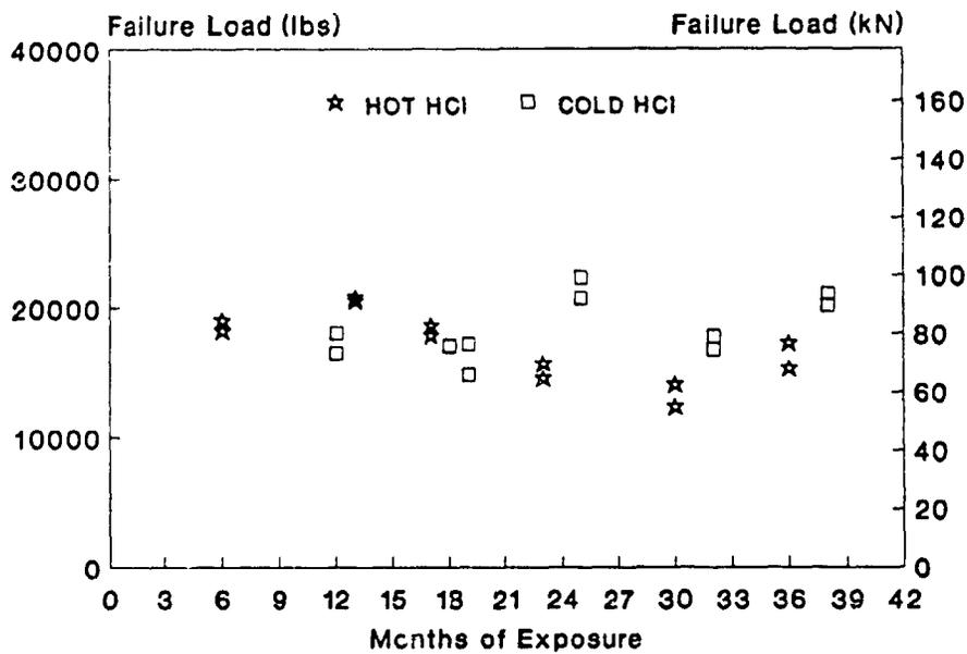
Fig. 7-18: Axial test failure load versus exposure time, PVC lined tubes exposed to hot and cold HCl.
