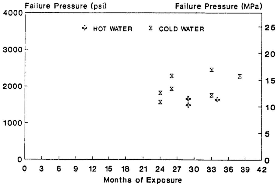
Fig. 7-14: Biaxial test failure pressure versus exposure time, PVC lined tubes exposed to hot and cold water.
