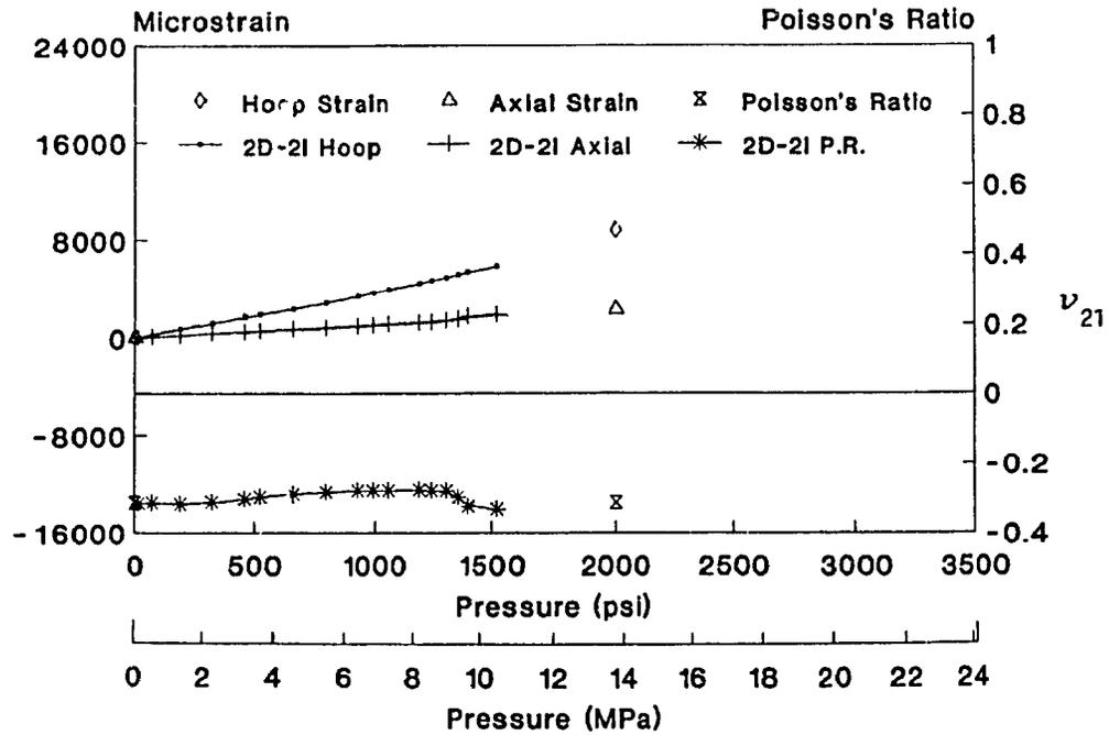
Fig. 7-34: Stress-strain graph, 2D-2I and theory. (Biaxial stress, veil lined tube)
