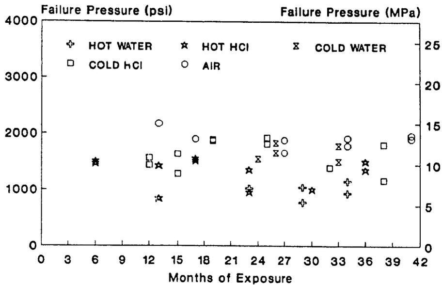
Fig. 7-11: Biaxial test failure pressure versus exposure time, veil lined tubes, all environments.
