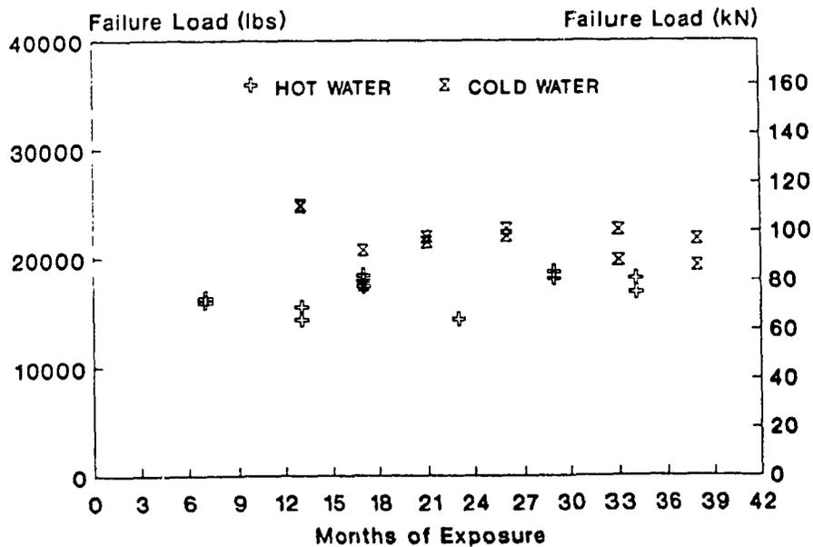
Fig. 7-6: Axial test failure load versus exposure time, veil lined tubes exposed to hot and cold water.
