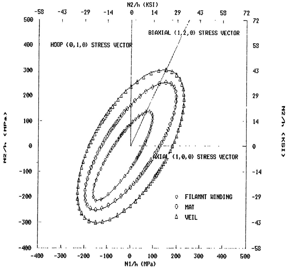
Fig. 4-9: Failure envelopes and stress vectors in stress space. Veil lined tube.
