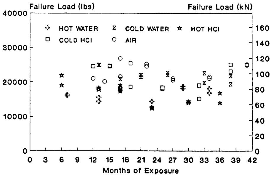
Fig. 7-12: Axial test failure load versus exposure time, veil lined tubes, all environments.
