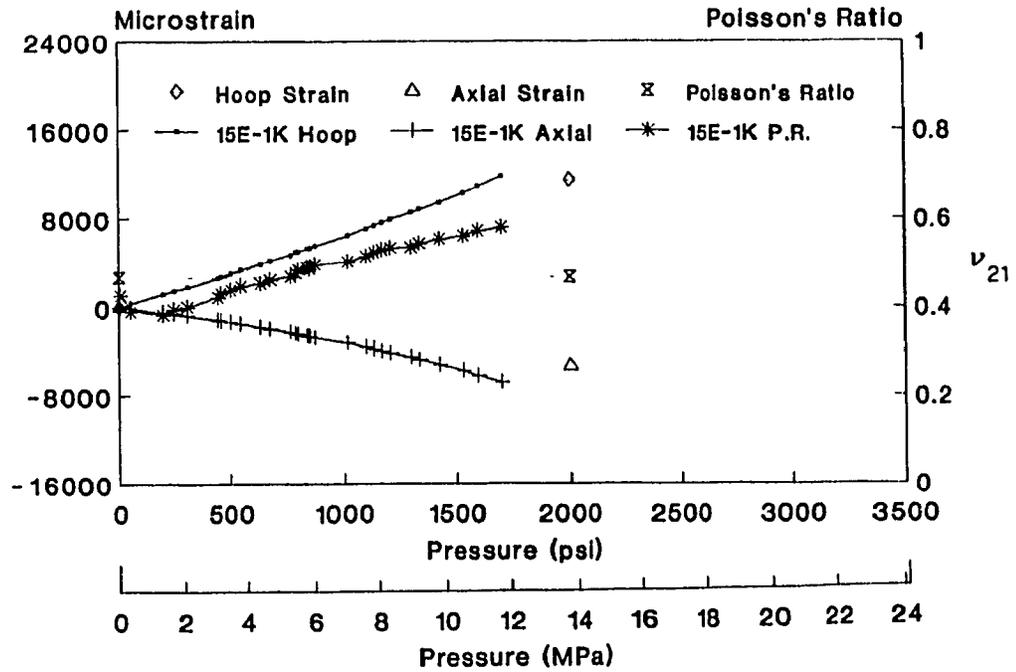
Fig. 7-33: Stress-strain graph, 15E-1K and theory (Hoop stress, veil lined tube).
