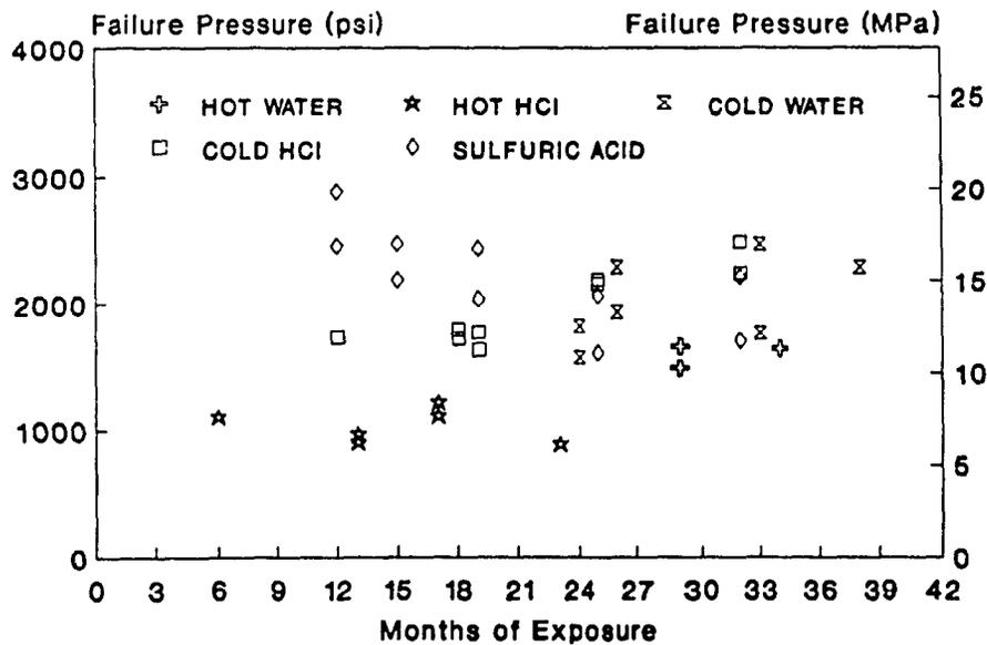
Fig. 7-23: Biaxial test failure pressure versus exposure time, PVC lined tubes, all environments.
