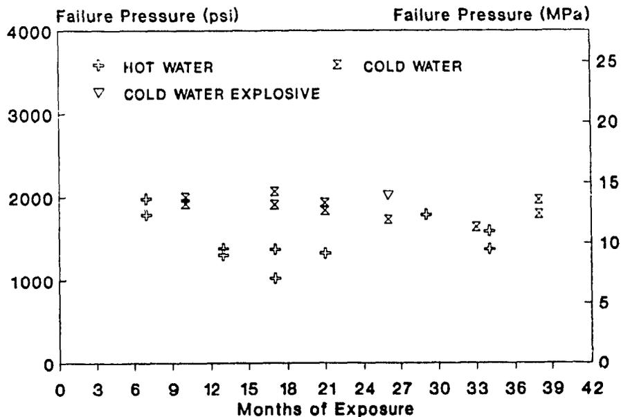
Fig. 7-13: Hoop test failure pressure versus exposure time, PVC lined tubes exposed to hot and cold water.
