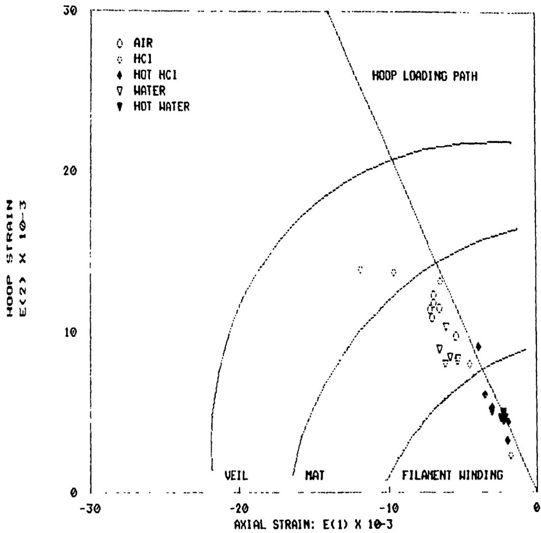
Fig. 7-26: Experimental results plotted onto the theoretical failure envelopes and loading paths in strain space, veil lined tubes, hoop test.
