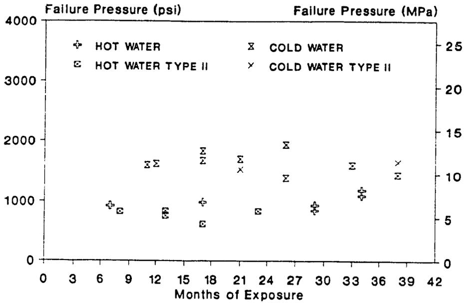
Fig. 7-4: Hoop test failure pressure versus exposure time, veil lined tubes exposed to hot and cold water.
