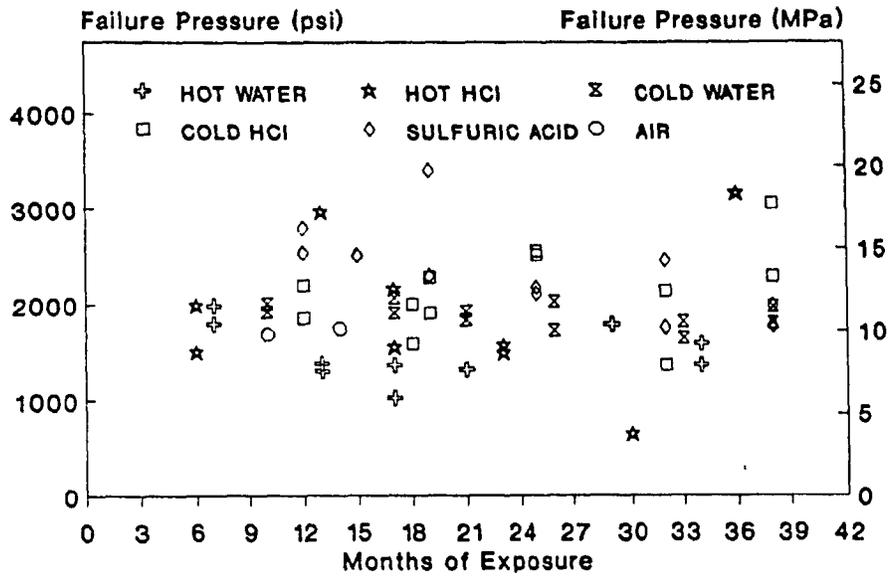
Fig. 7-22: Hoop test failure pressure versus exposure time, PVC lined tubes, all environments.
