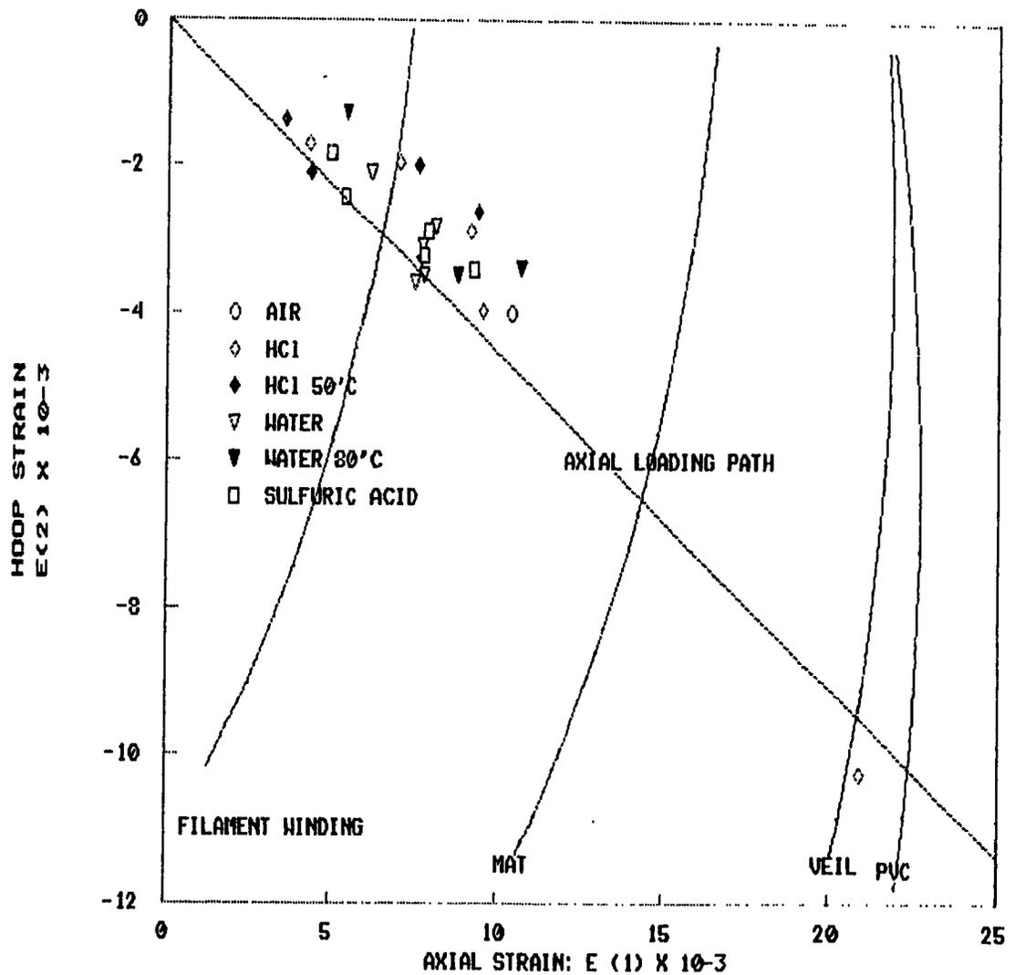
Fig. 7-32: Experimental results plotted onto the theoretical failure envelopes and loading paths in strain space. PVC lined tubes, axial test.
