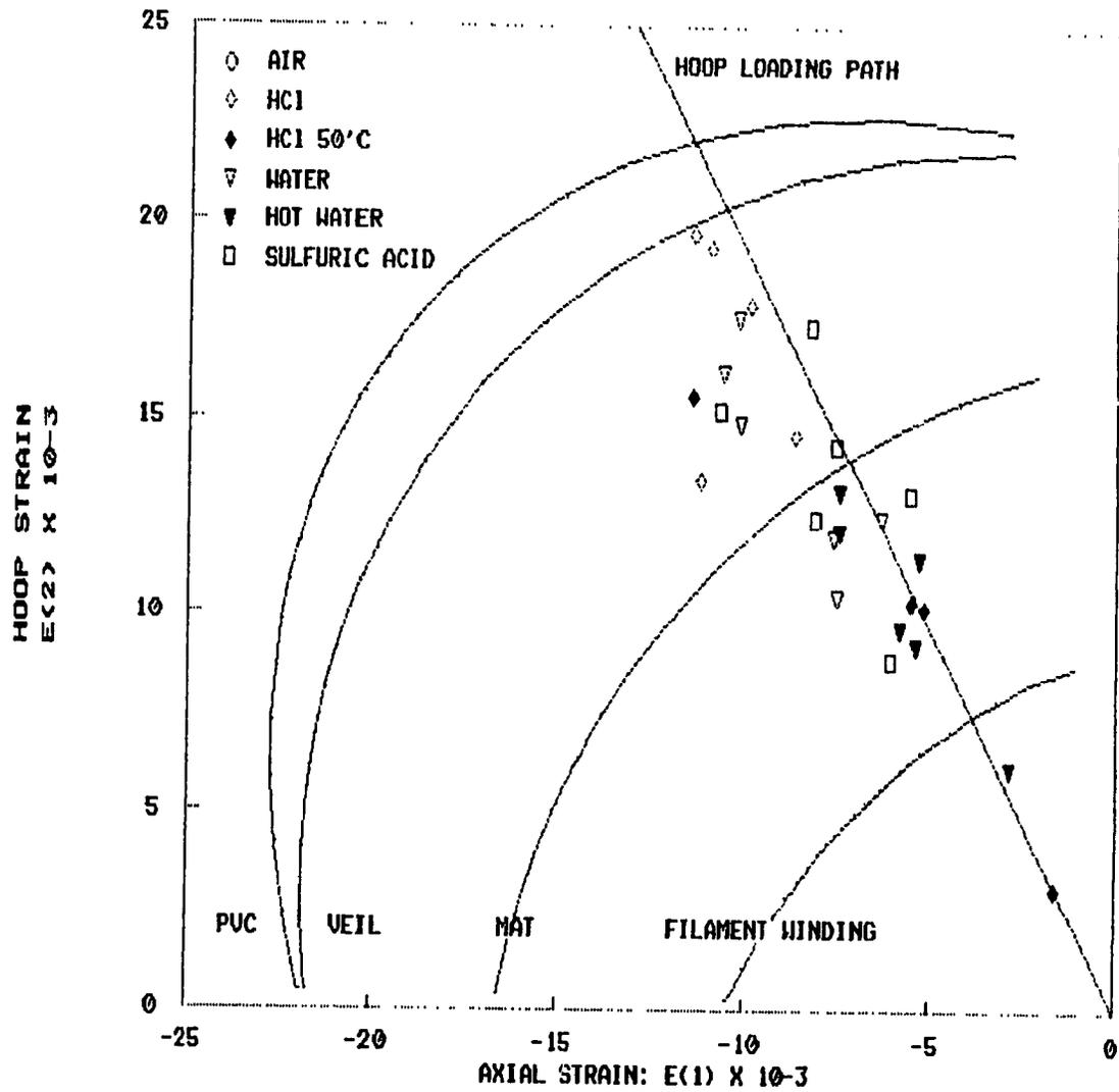
Fig. 7-30: Experimental results plotted onto the theoretical failure envelopes and loading paths in strain space. PVC lined tubes, hoop test.
