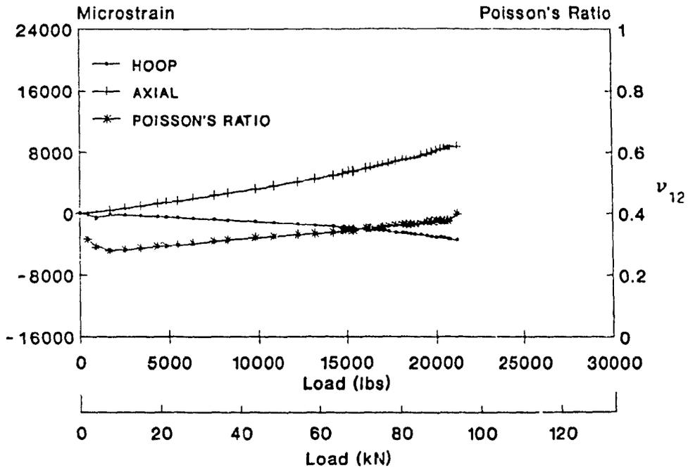
Fig 6-40: Strain and Poisson's ratio versus load graph for PVC lined tube 21A-3C
