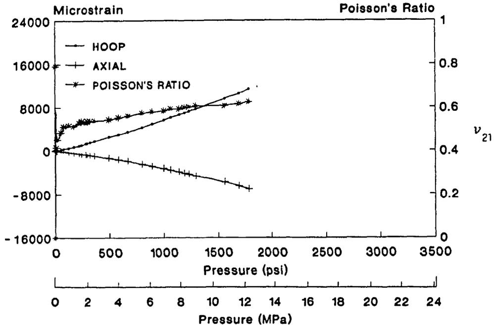
Fig. 6-24: Strain and Poisson's ratio versus pressure graph for veil lined tube 11E-1C.
