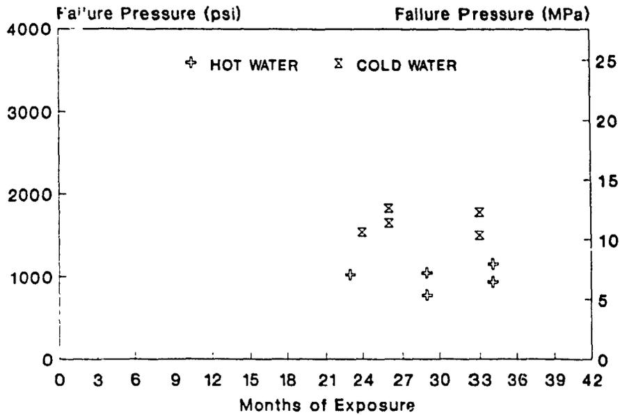
Fig. 7-5: Biaxial test failure pressure versus exposure time, veil lined tubes exposed to hot and cold water.
