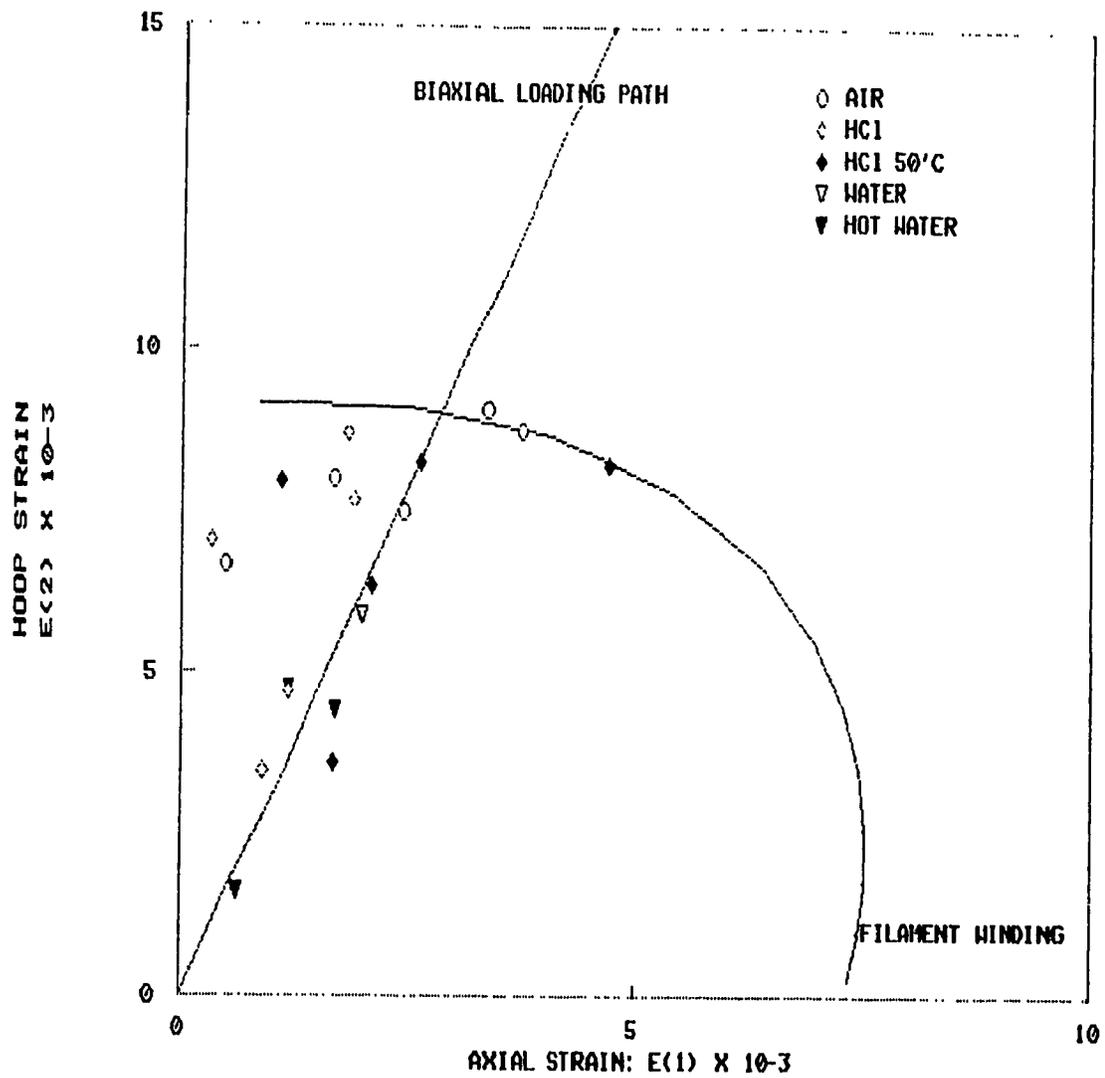
Fig. 7-27: Experimental results plotted onto the theoretical failure envelopes and loading paths in strain space, veil lined tubes, biaxial test.
