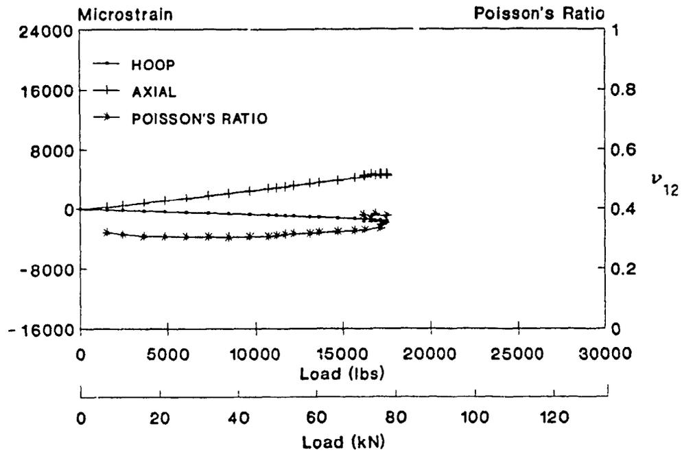
Fig. 6-41: Strain and Poisson's ratio versus load graph for veil lined tube 7C-3I.
