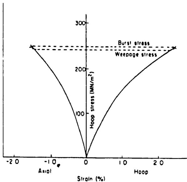
Fig. 2-3: Typical stress-strain response for a  $\pm 55^\circ$  filament wound E-glass/epoxy tube under hoop stress [31].
