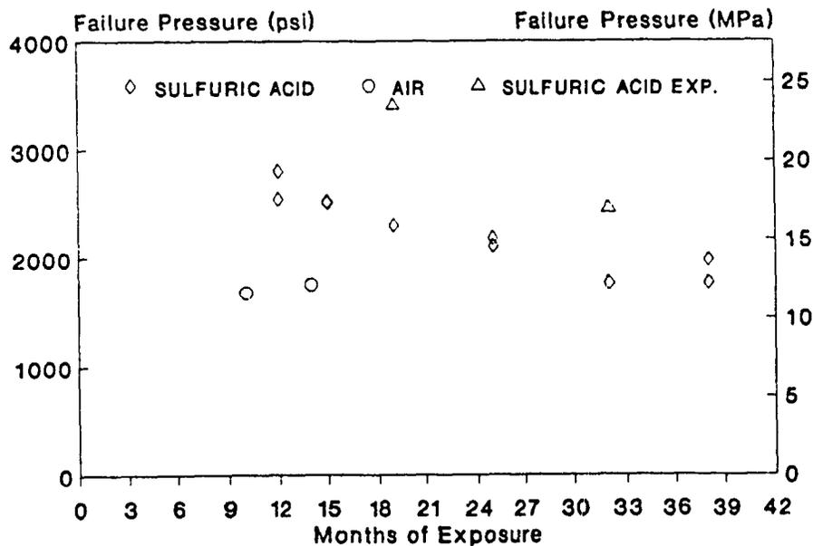
Fig. 7-19: Hoop test failure pressure versus exposure time, PVC lined tubes exposed to sulfuric acid and air.
