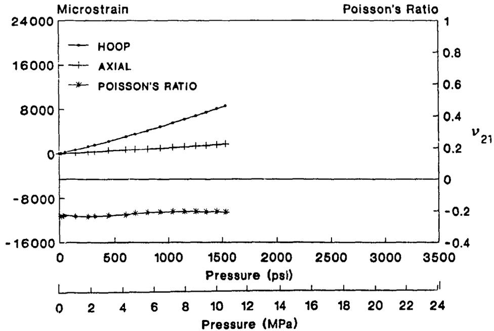
Fig. 6-31: Strain and Poisson's ratio versus pressure graph for PVC lined tube 31C-2A.
