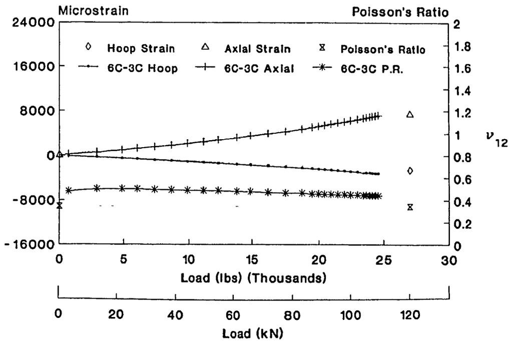
Fig. 7-35: Stress-strain graph, 6C-3C and theory. (Axial stress, veil lined tube)
