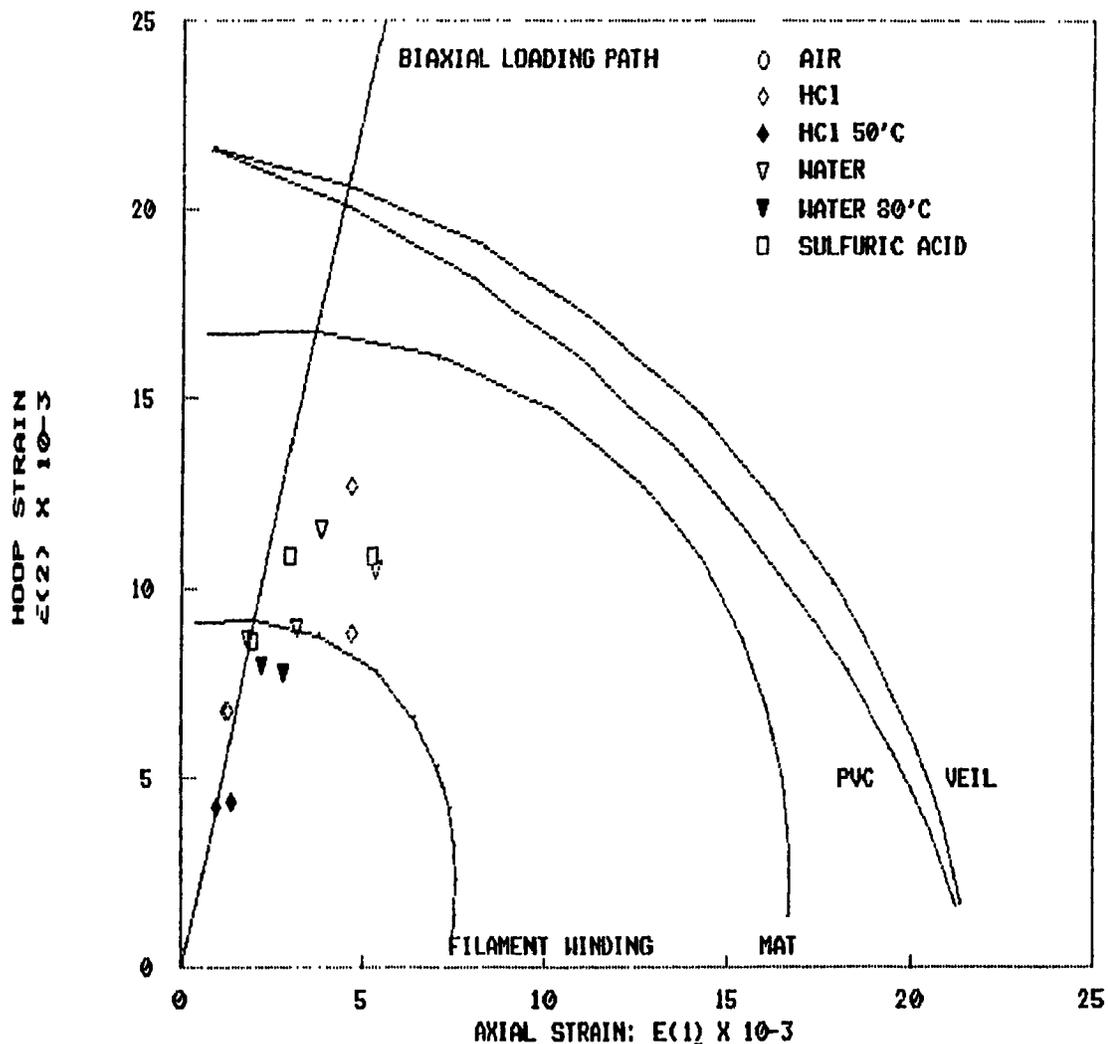
Fig. 7-31: Experimental results plotted onto the theoretical failure envelopes and loading paths in strain space. PVC lined tubes, biaxial test.
