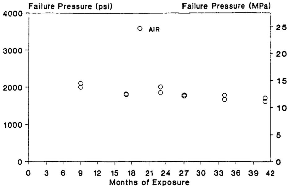
Fig. 7-1: Hoop test failure pressure versus exposure time, veil lined tubes exposed to air.
