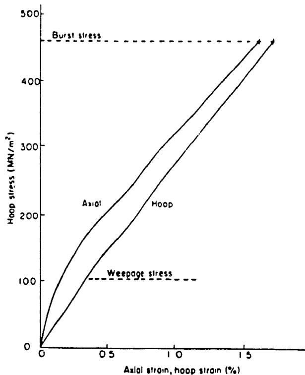
Fig. 2-2: Typical stress-strain behavior of a  $\pm 55^\circ$  filament wound E-glass/epoxy tube under biaxial stress [31].
