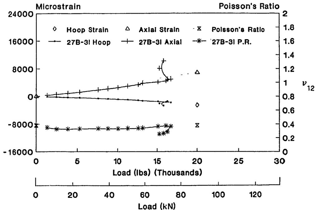
Fig. 7-38: Stress-strain graph, 27B-3I and theory. (Axial stress, PVC lined tube)
