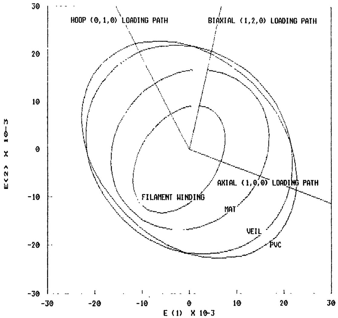
Fig. 4-10: Failure envelopes and loading paths in strain space. PVC lined tube.
