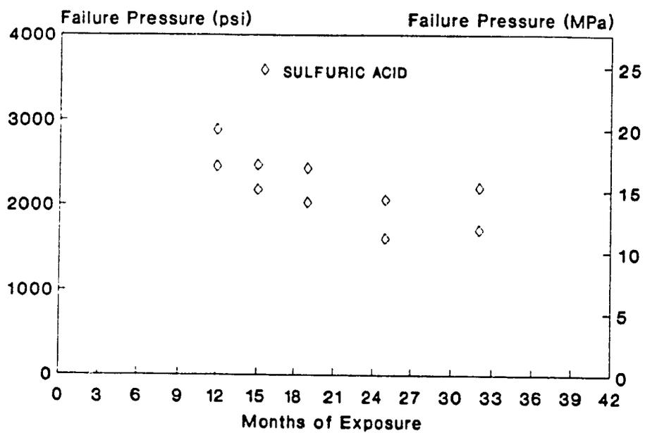
Fig. 7-20: Biaxial test failure pressure versus exposure time, PVC lined tubes exposed to sulfuric acid.
