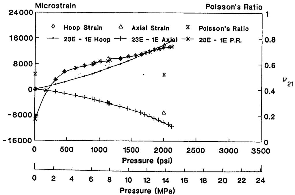
Fig. 7-36: Stress-strain graph, 23E-1E and theory (Hoop stress, PVC lined tube).
