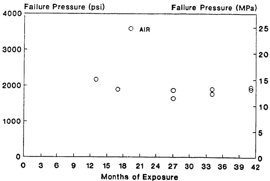
Fig. 7-2: Biaxial test failure pressure versus exposure time, veil lined tubes exposed to air.
