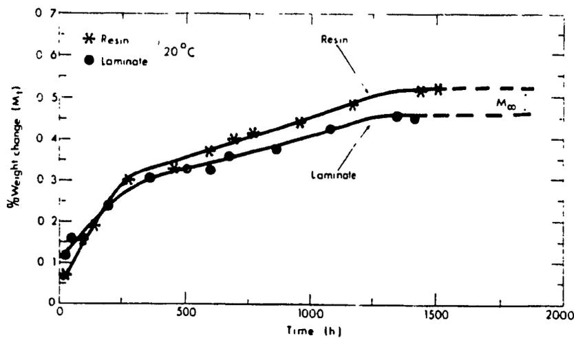
Fig. 2-1: Sorption data for vinyl ester resins and resin/glass laminates immersed in water at 20°C [40].
