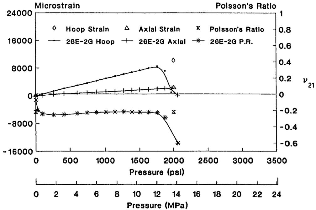
Fig. 7-37: Stress-strain graph, 26E-2G and theory. (Biaxial stress, PVC lined tube)
