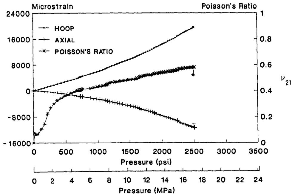
Fig. 6-23: Strain and Poisson's ratio versus pressure graph for PVC lined tube 29A-1G.
