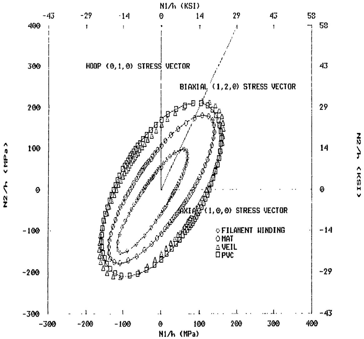
Fig. 4-8: Failure envelopes and stress vectors in stress space. PVC lined tube.
