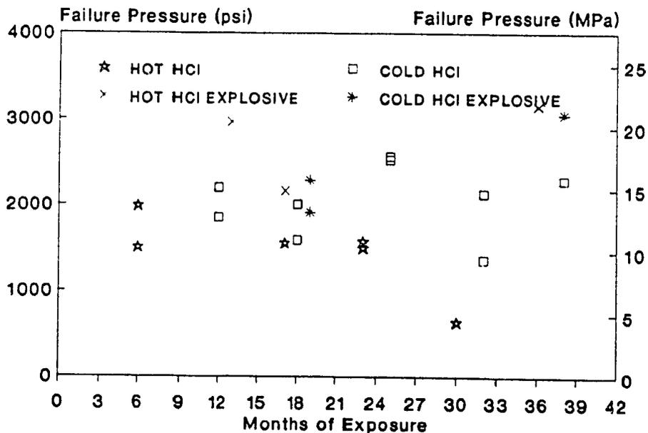
Fig. 7-16: Hoop test failure pressure versus exposure time, PVC lined tubes exposed to hot and cold HCl.
