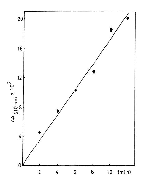
number of moles of  $Fe^{2+}$  ion calculated from the slope  $(2.8 \times 10^{-4})$  was  $9.6 \times 10^{-10}$  mole s<sup>-1</sup> and the corresponding light intensity was calculated to be  $1.9 \times 10^{-9}$  einstein s<sup>-1</sup> (eq.2.19).
