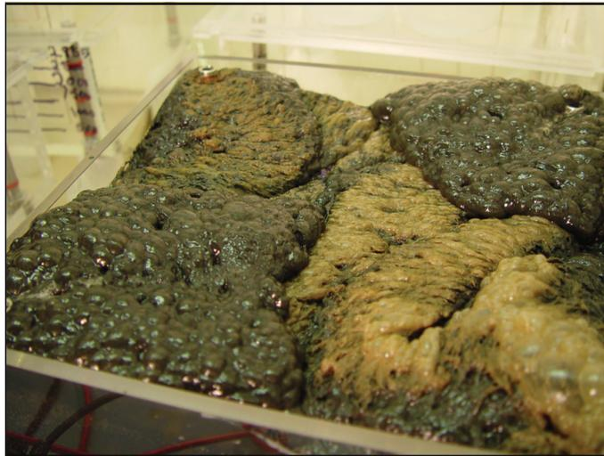
Figure 5.4: Bubble creation in BioElectro™ system
