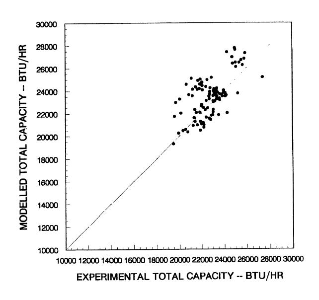
Figure 4.9. Total cooling capacity comparison of the air-conditioning system.
