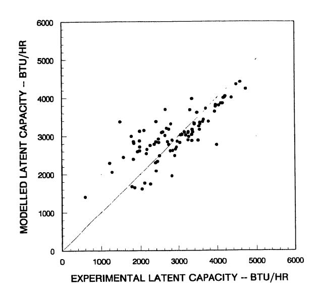
Figure 4.5. Latent cooling capacity comparison of the eight-row evaporator.
