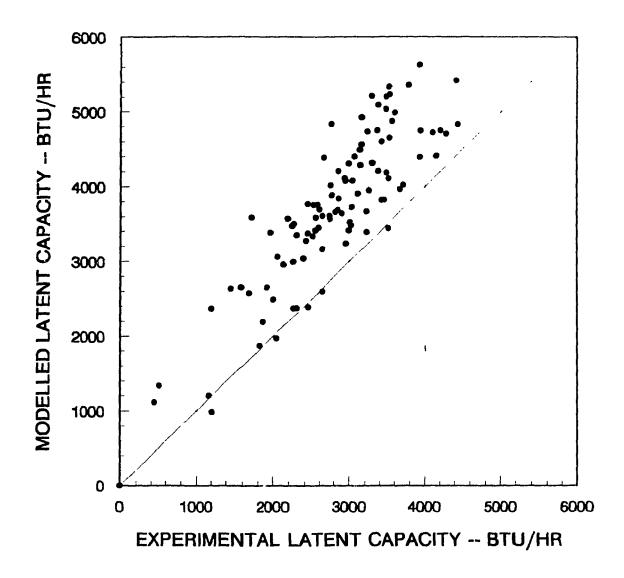
Figure 4.11. Latent cooling capacity comparison of the air-conditioning system.
