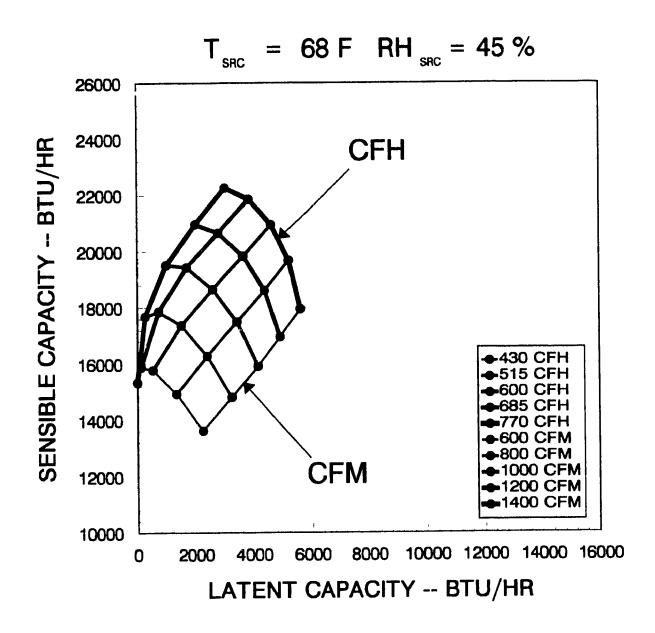
Figure 5.1. Experimental system capacities with a source temperature of 68°F and relative humidity of 45%.
