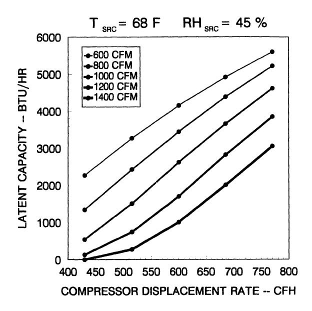
Figure 6.6. System latent capacity versus compressor volumetric displacement rate.
