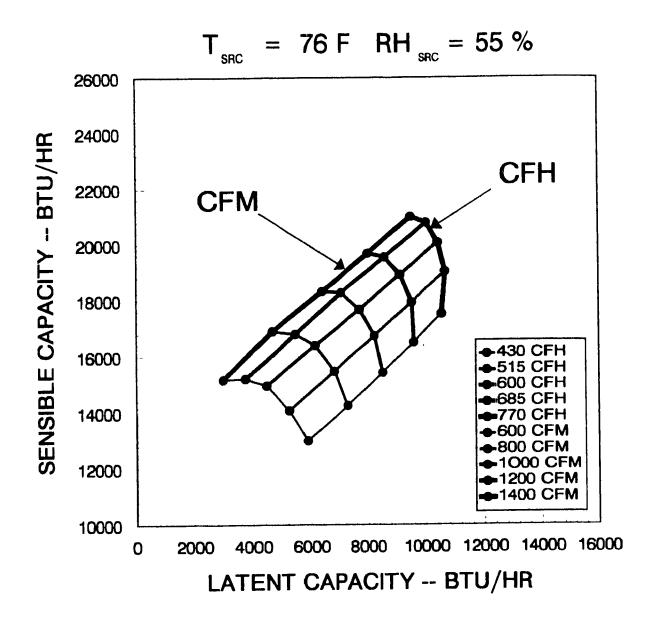
Figure 5.2. Experimental system capacities with a source temperature of 76°F and relative humidity of 55%.
