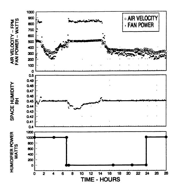
Figure 6.1. Experimental results--space relative humidity, humidifier power, space air velocity and fan power versus time.
