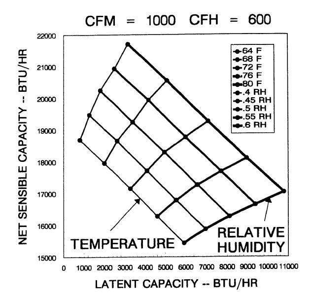
Figure 5.3. Experimental system capacities with a compressor volumetric displacement rate of 600 CFH and a evaporator air flow rate of 1000 CFM.
