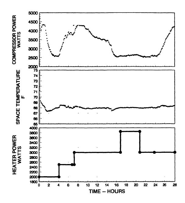
Figure 6.2. Experimental results--space temperature, compressor power and heater power versus time.
