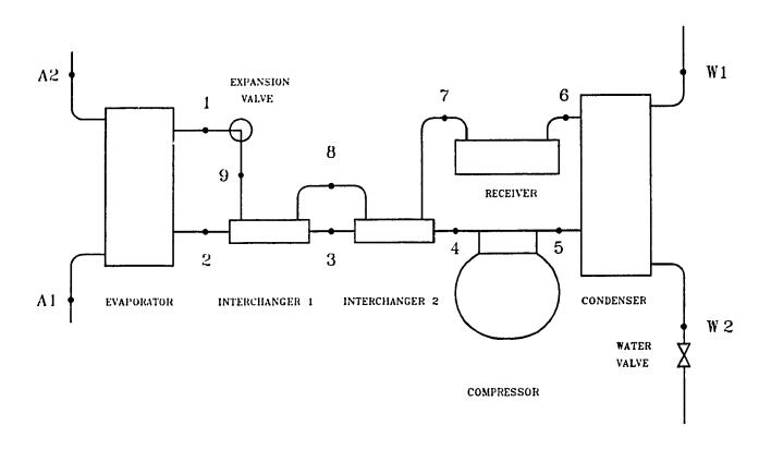
Figure 3.1. Air-conditioning system.
