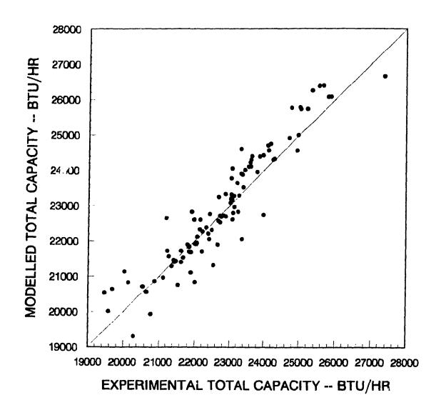
Figure 4.6. Total cooling capacity comparison of the four-row evaporator.
