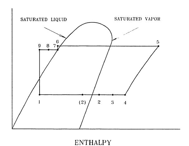
Figure 3.2. Pressure-enthalpy diagram of air-conditioning system.
