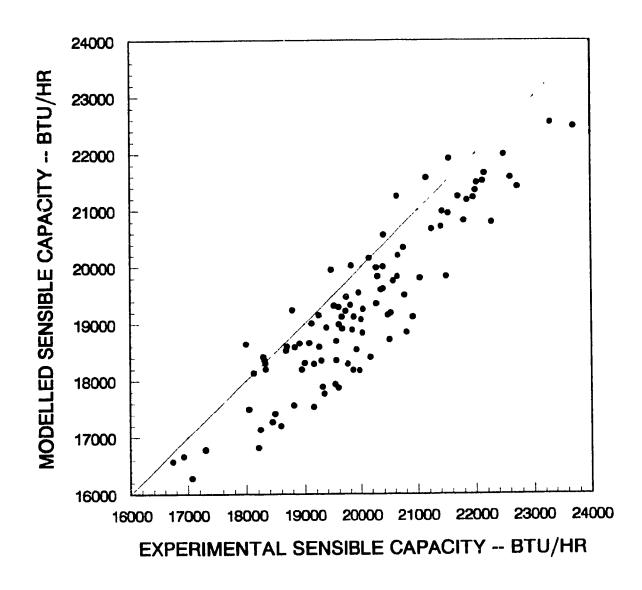
Figure 4.7. Sensible cooling capacity comparison of the four-row evaporator.
