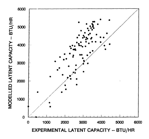
Figure 4.8. Latent cooling capacity comparison of the four-row evaporator.
