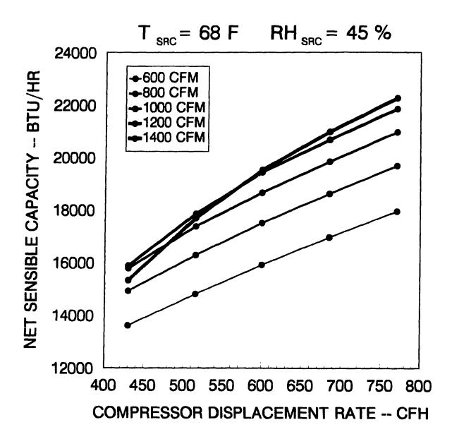
Figure 6.5. System net sensible capacity versus compressor volumetric displacement rate.
