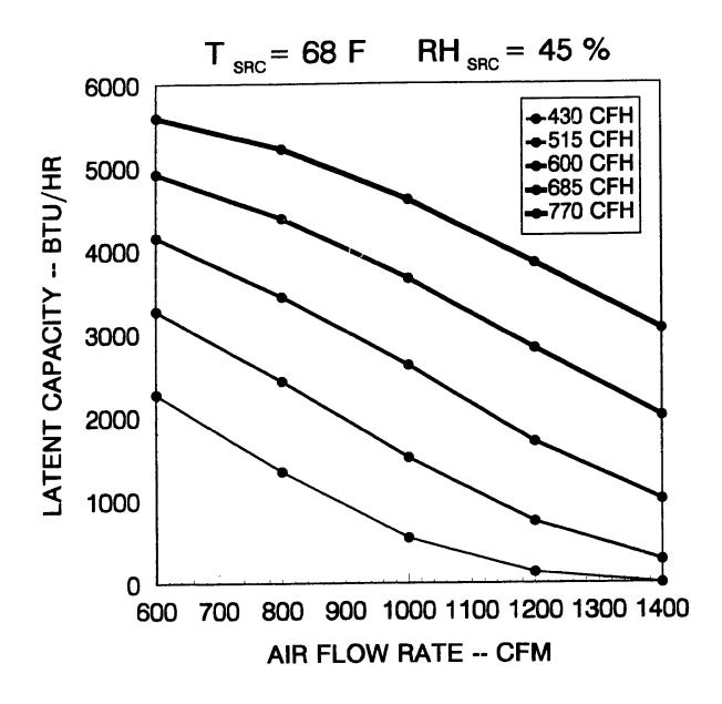
Figure 6.7. System latent capacity versus evaporator air flow rate.
