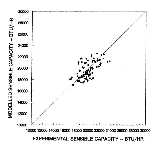
Figure 4.10. Sensible cooling capacity comparison of the air-conditioning system.
