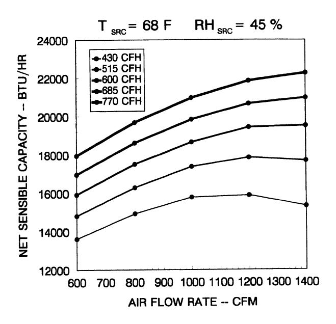
Figure 6.4. System net sensible capacity versus evaporator air flow rate.
