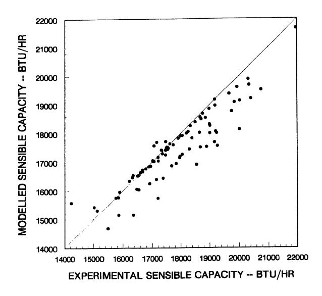
Figure 4.4. Sensible cooling capacity comparison of the eight-row evaporator.
