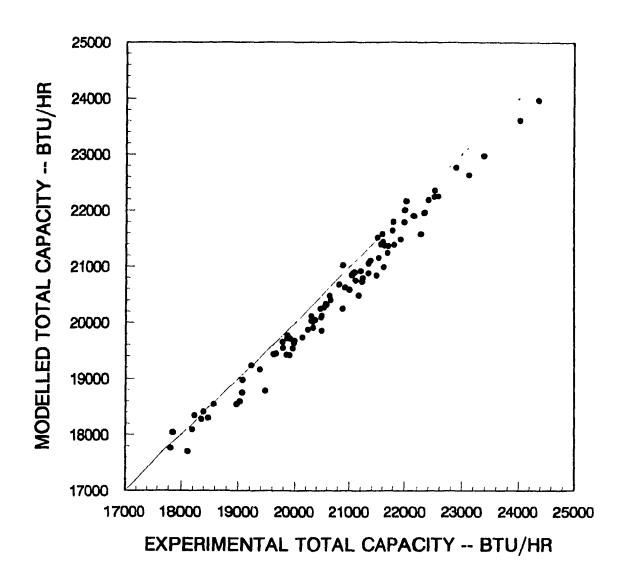
Figure 4.3. Total cooling capacity comparison of the eight-row evaporator.
