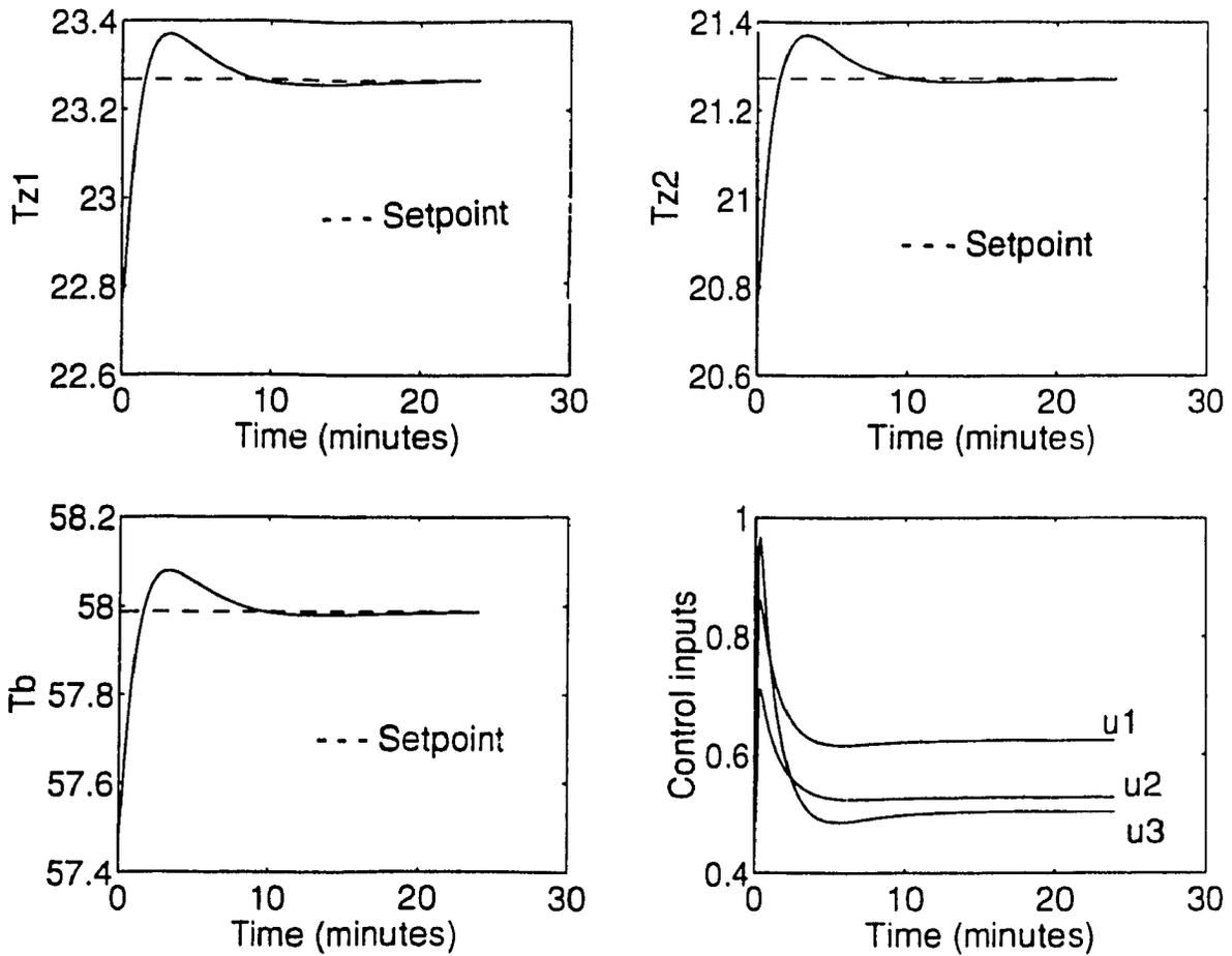
Figure 5.19: Closed-loop response showing the effect of adding extra valve dynamics when the controller is designed using pole placement.
