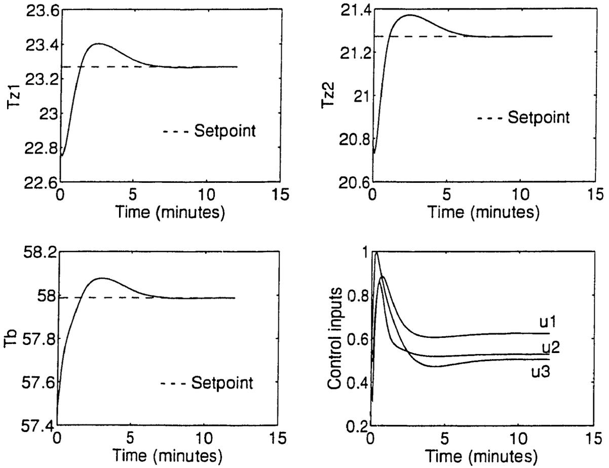
Figure 5.20: Closed-loop response showing the effect of adding extra valve dynamics when the controller is designed using LQR.
