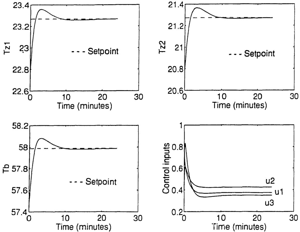
Figure 5.11: Closed-loop response showing the robustness properties when the controller is designed using pole placement theory:  $a_{z1}$  and  $a_{z2}$  are changed by 30 % each.
