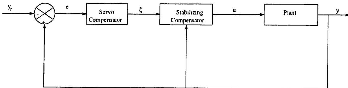
Figure 3.5: A robust controller for the servomechanism problem
