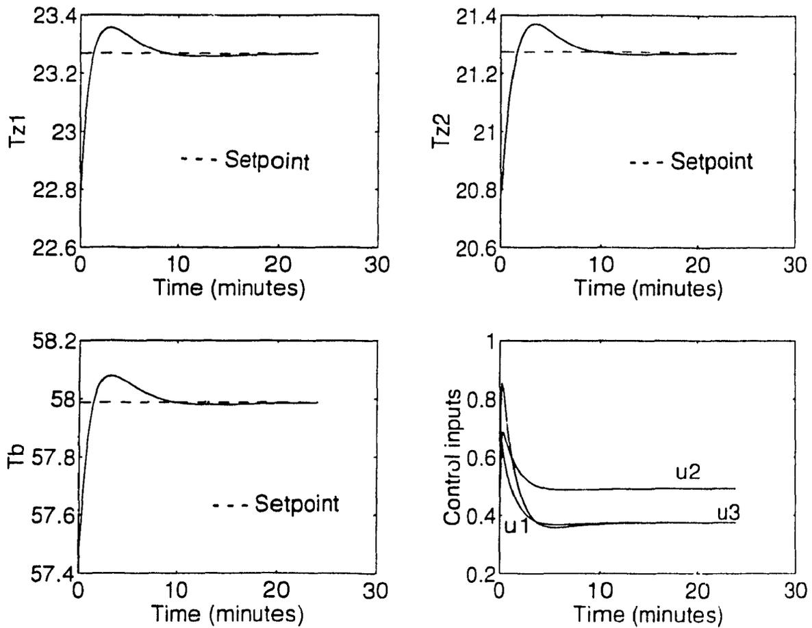
Figure 5.10: Closed-loop response showing the robustness properties when the controller is designed using pole placement theory:  $a_{21}$  is changed by 30 %
