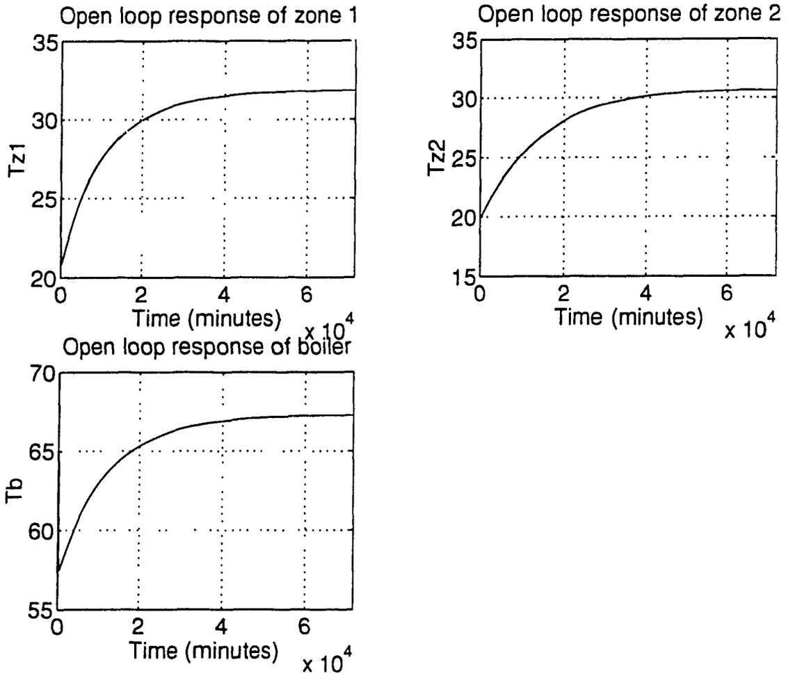
Figure 3.3: Effect of step changes in the control input on the open-loop response of the MFCH system.
