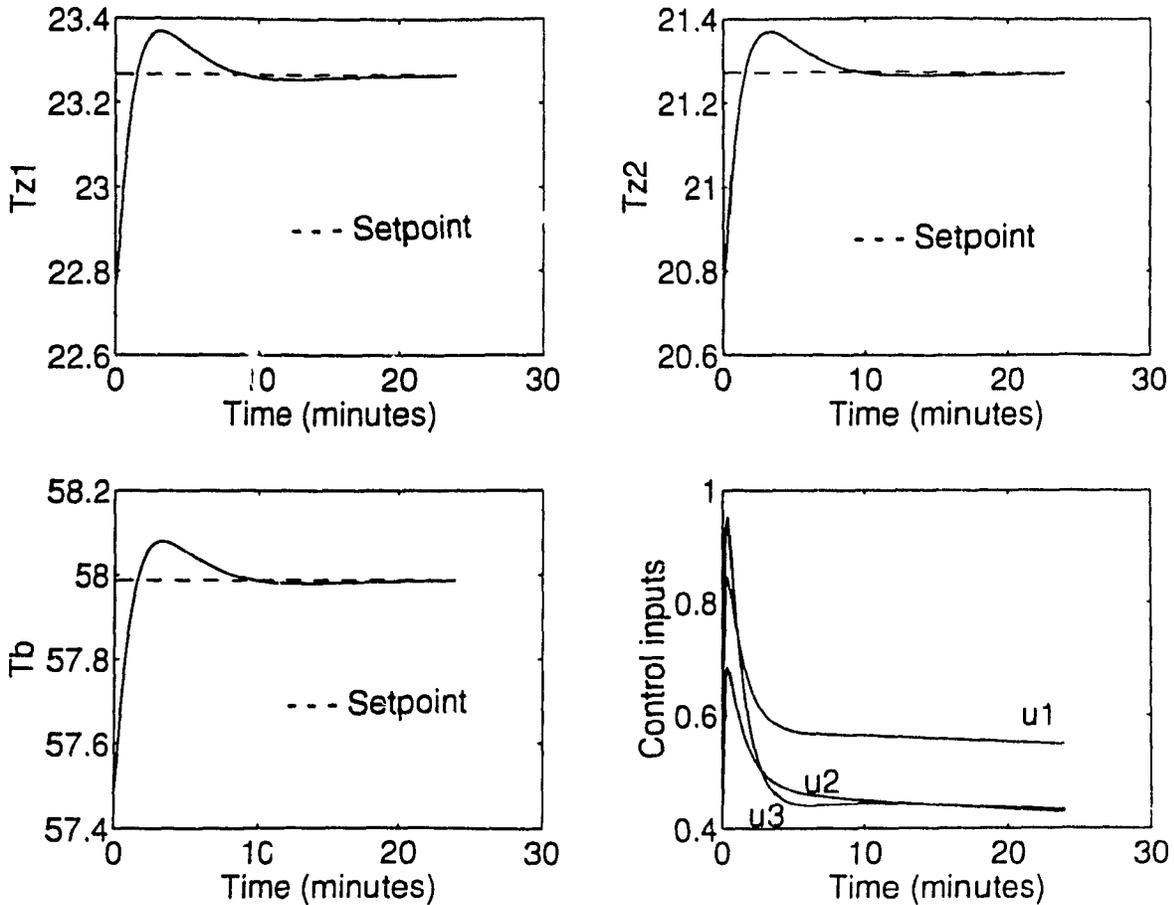
Figure 5.6: Closed-loop response showing the effect of perturbation in initial conditions, static, and dynamic disturbances for the controller designed using pole placement theory
