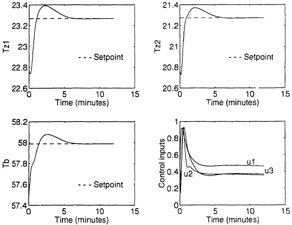
Figure 5.9: Closed-loop response showing the effect of perturbations in initial conditions and dynamic disturbance for the controller designed using LQR theory
