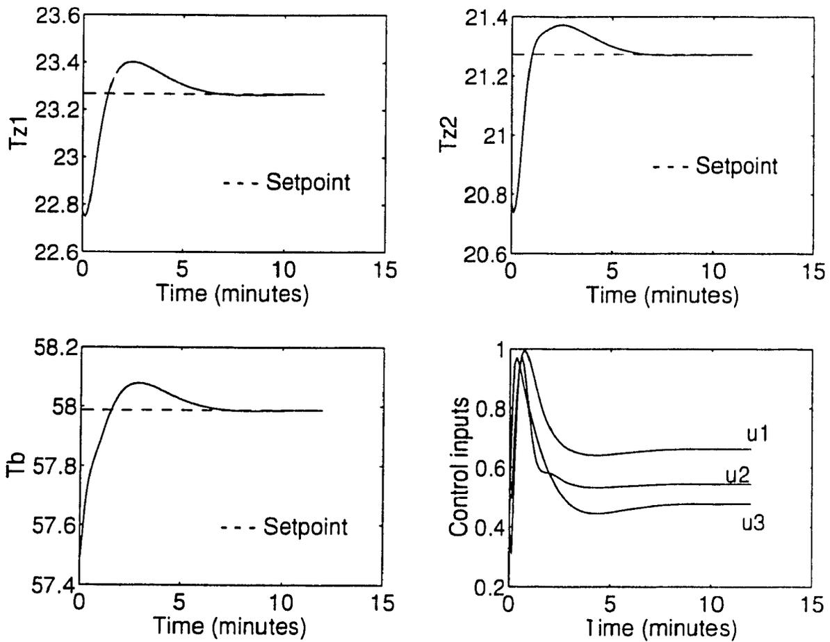
Figure 5.16: Closed-loop response showing the robustness properties when the controller is designed using LQR theory:  $\xi_z$  is changed by 20 %.
