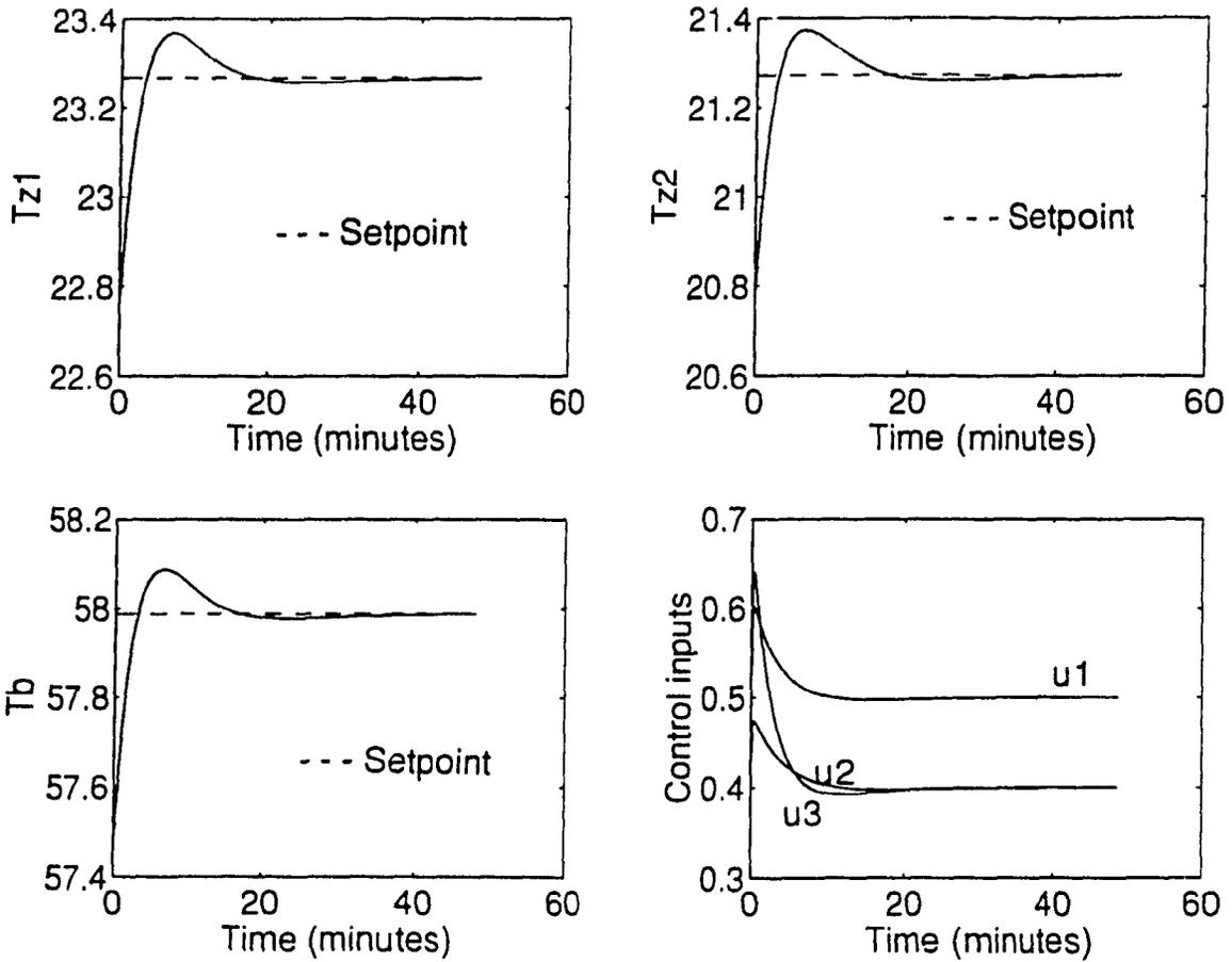
Figure 5.1: Closed-loop response showing the effect of perturbations in the initial conditions for the controller designed using pole placement theory
