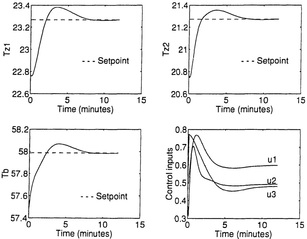
Figure 5.18: Closed-loop response when there is no estimation-error feedback to the controller.
