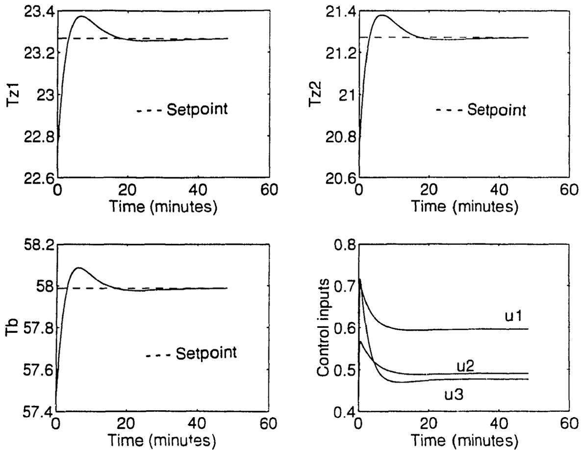
Figure 5.3: Closed-loop response showing the effect of perturbations in initial conditions and static disturbance for the controller designed using pole placement theory
