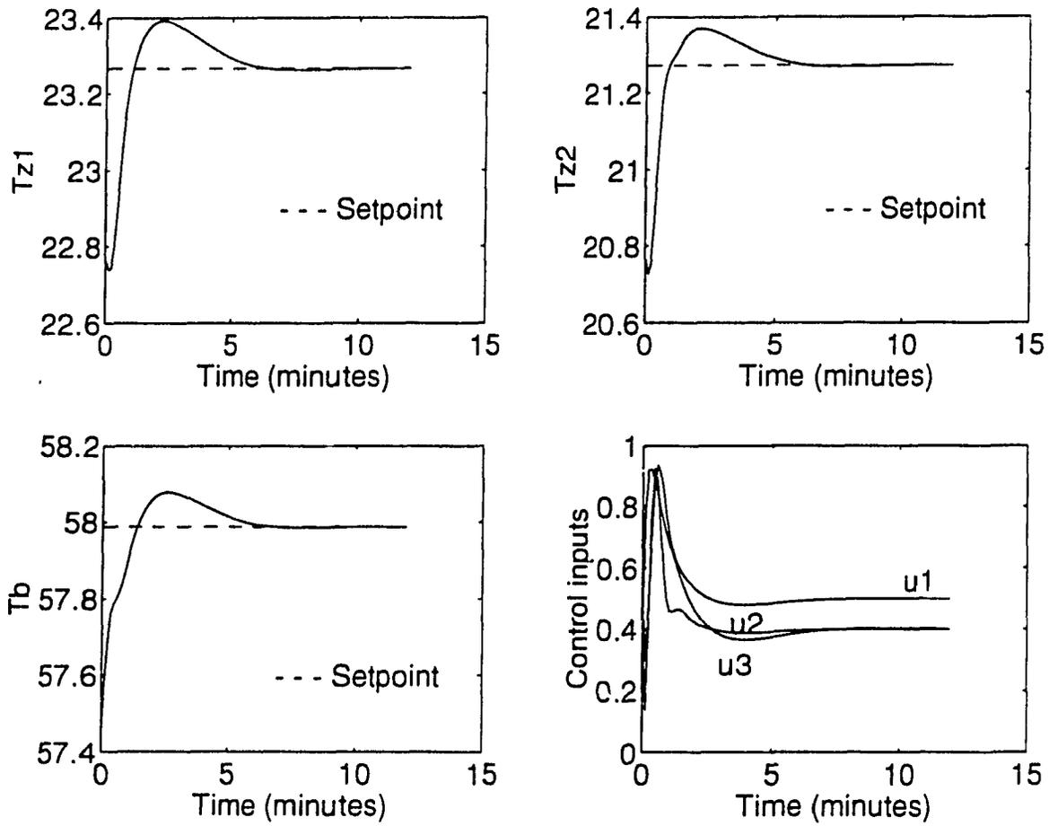
Figure 5.2: Closed-loop response showing the effect of perturbations in the initial conditions for the controller designed using LQR theory.
