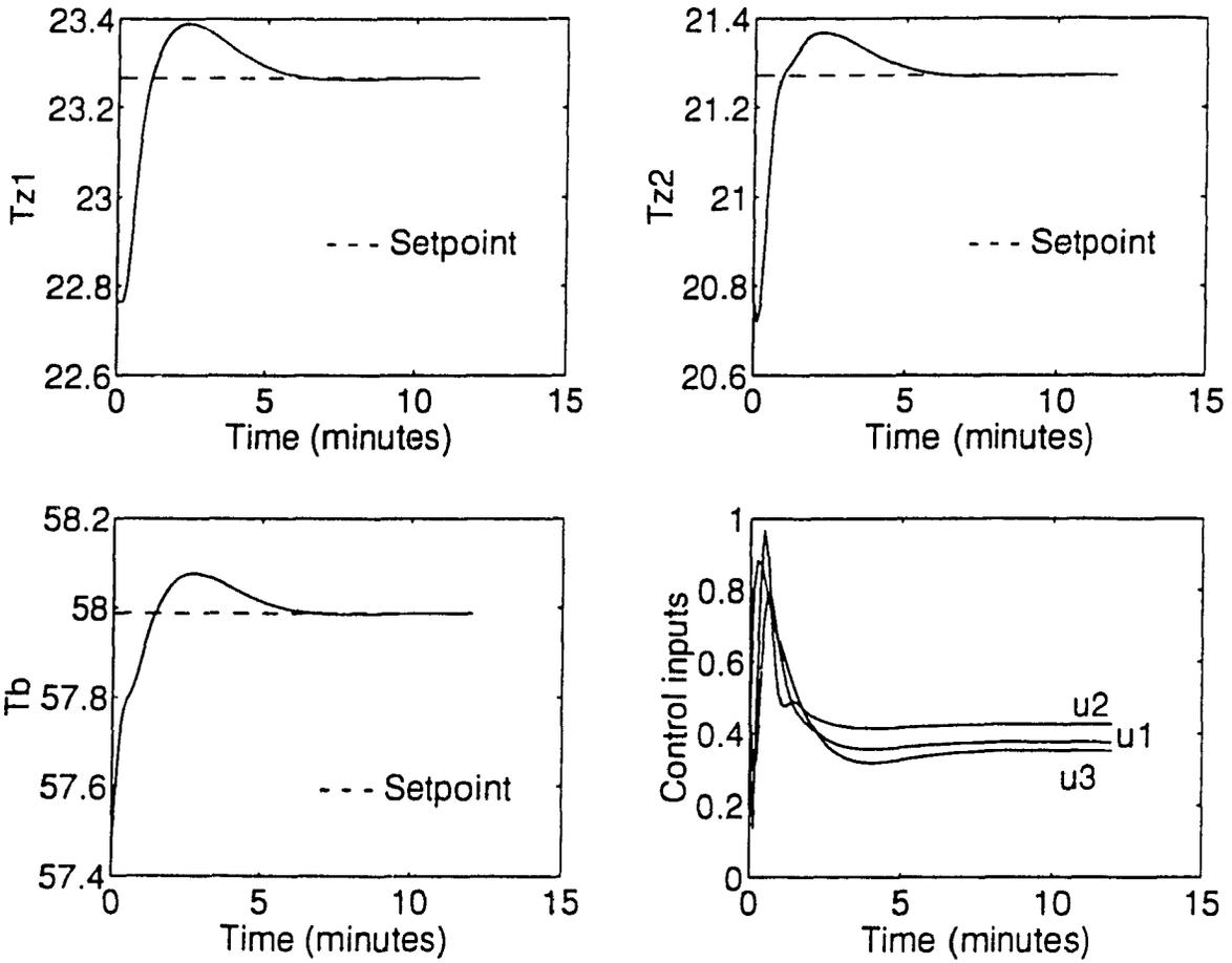
Figure 5.15: Closed-loop response showing the robustness properties when the controller is designed using LQR theory:  $a_{z1}$  and  $a_{z2}$  are changed by 30 % each.
