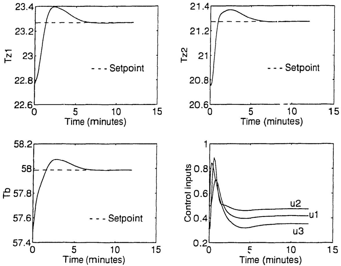
Figure 5.17: Closed-loop response showing the robustness properties when the controller is designed using LQR theory:  $a_{z1}$ ,  $a_{z2}$ , and  $\xi_z$  are changed by 30 %, 30 %, and 20 % respectively.
