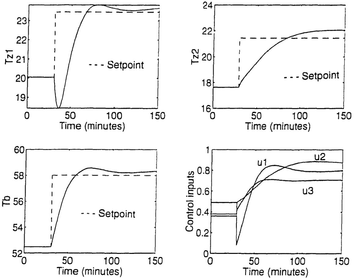
Figure 5.22: Closed-loop response showing the effect of step changes in the operating point with fixed-gain controller.
