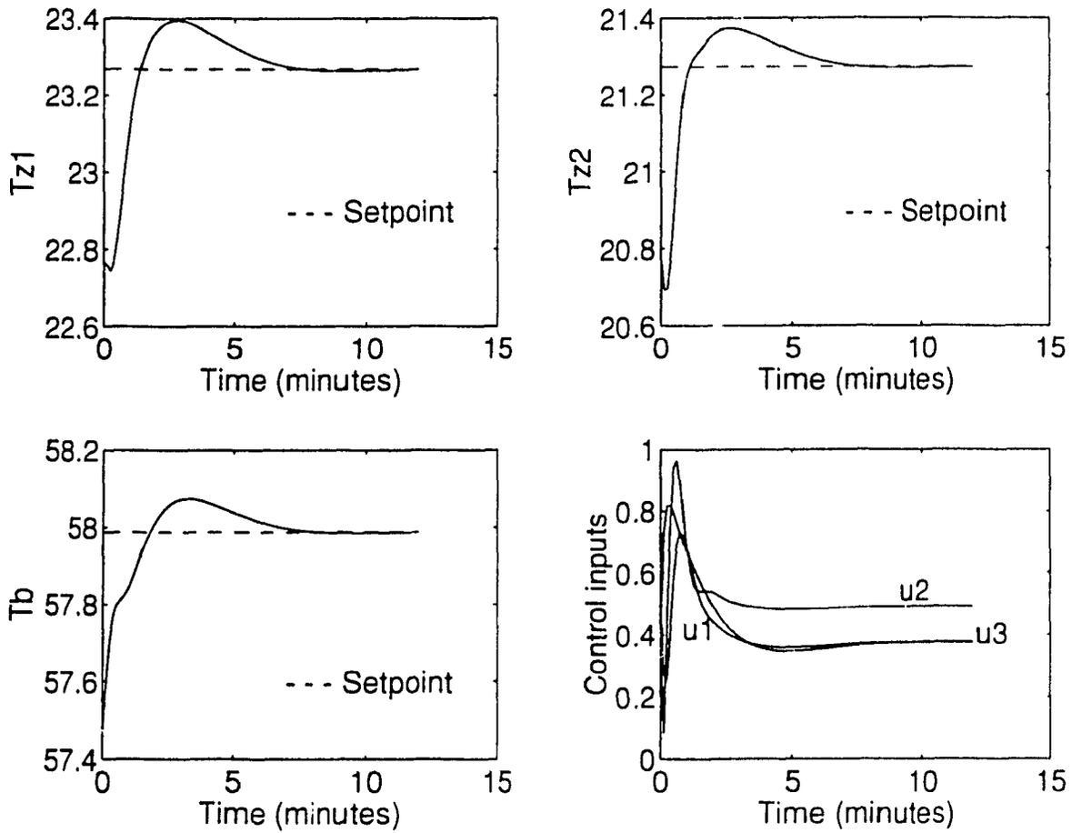
Figure 5.14: Closed-loop response showing the robustness properties when the controller is designed using LQR theory:  $a_{z1}$  is changed by 30 %
