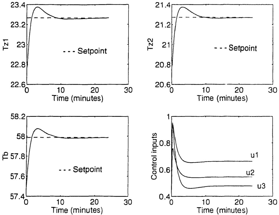
Figure 5.12: Closed-loop response showing the robustness properties when the controller is designed using pole placement theory:  $\xi_c$  is changed by 20 %
