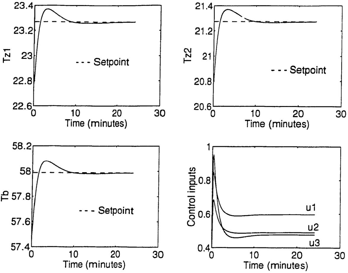
Figure 5.5: Closed-loop response showing the effect of perturbations in initial conditions and static disturbances for the controller designed using pole placement theory: Improved response.
