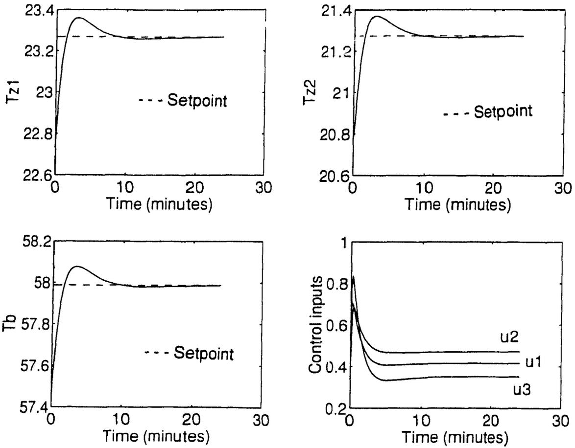
Figure 5.13: Closed-loop response showing the robustness properties when the controller is designed using pole placement theory:  $a_{z1}$ ,  $a_{z2}$ , and  $\xi_z$  are changed by 30 %, 30 %, and 20 % respectively.
