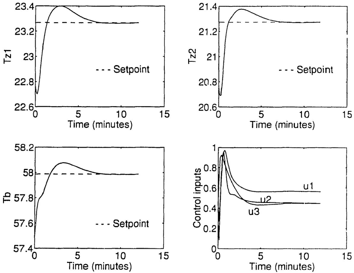
Figure 5.7: Closed-loop response showing the effect of perturbations in initial conditions, static, and dynamic disturbances for the controller designed using LQR theory.
