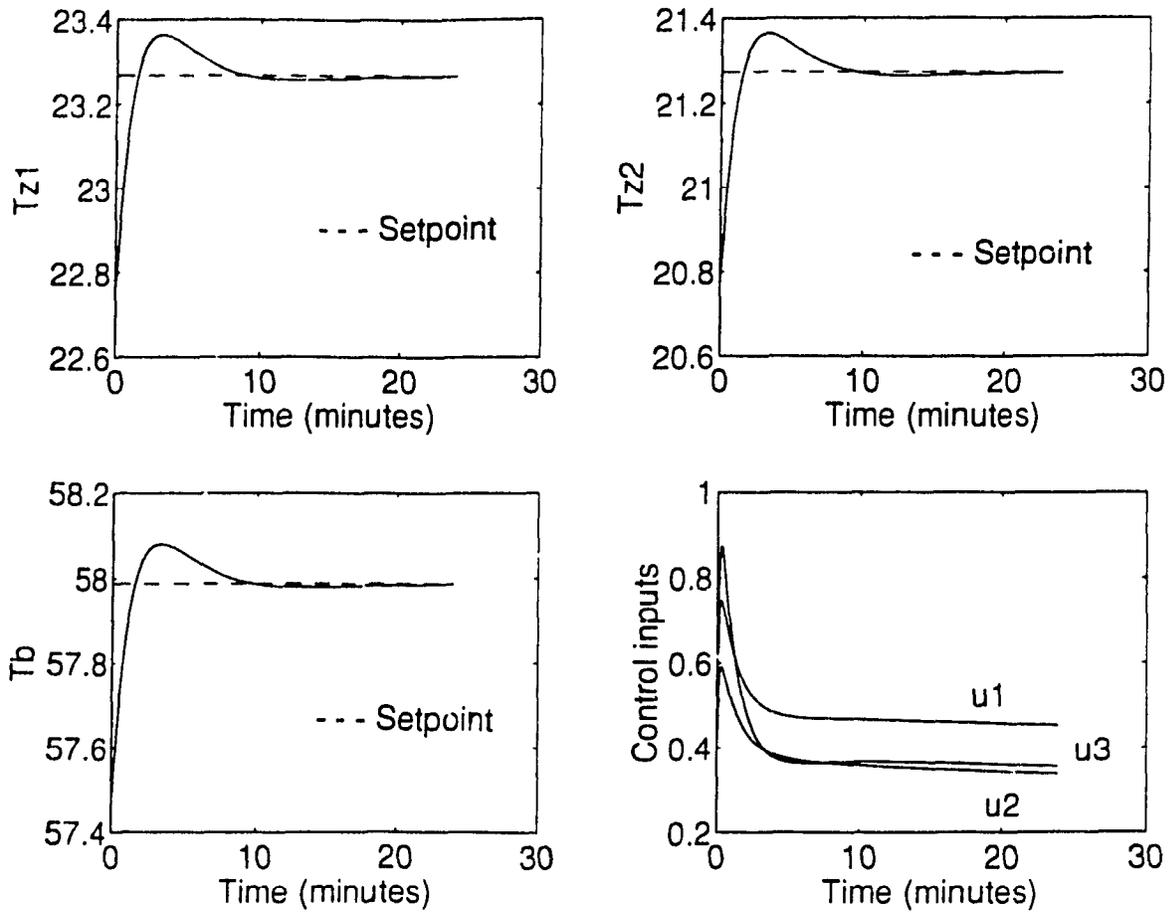
Figure 5.8: Closed-loop response showing the effect of perturbation in initial conditions and dynamic disturbance for the controller designed using pole placement theory
