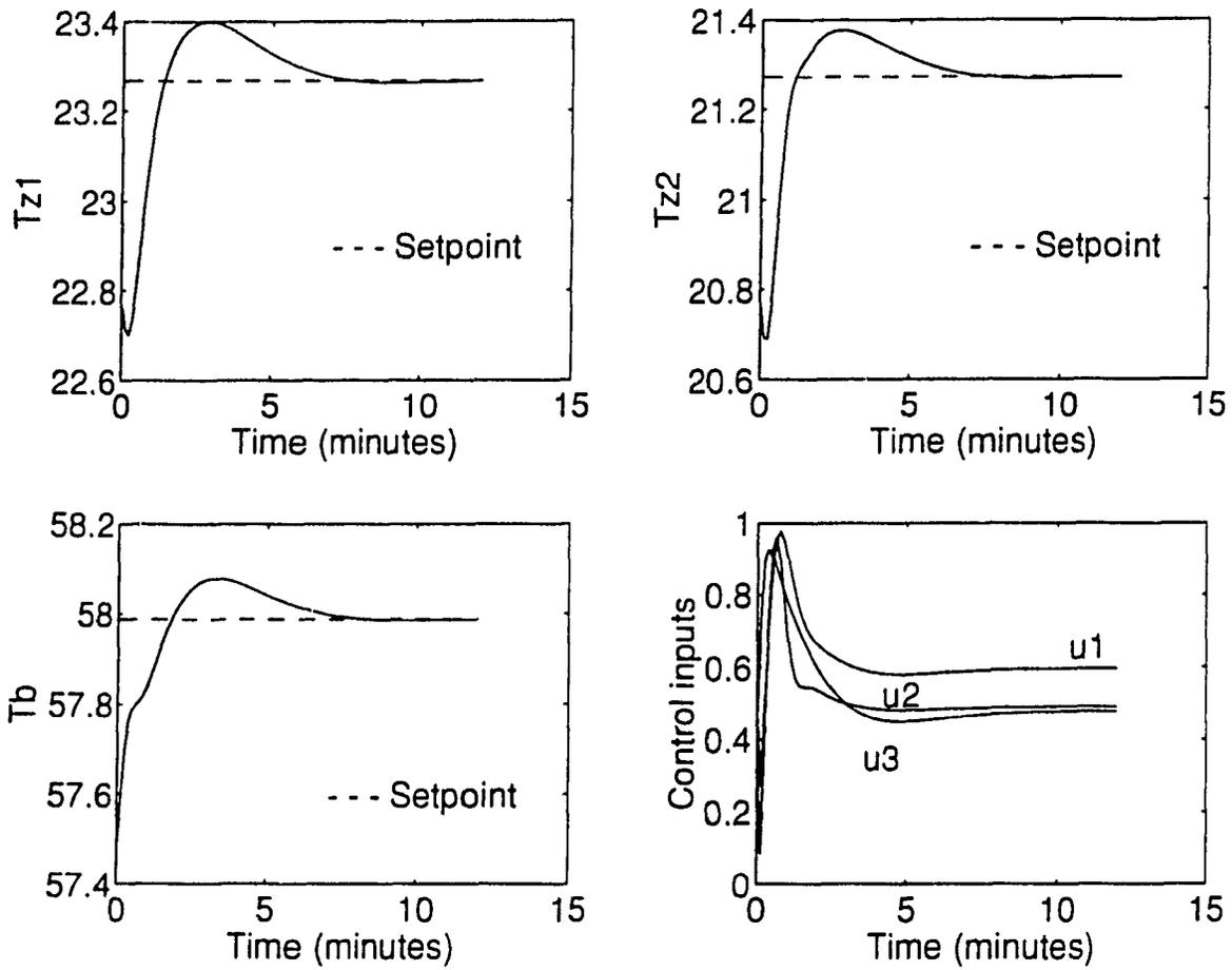
Figure 5.4: Closed-loop response showing the effect of perturbations in initial conditions and static disturbance for the controller designed using LQR theory.
