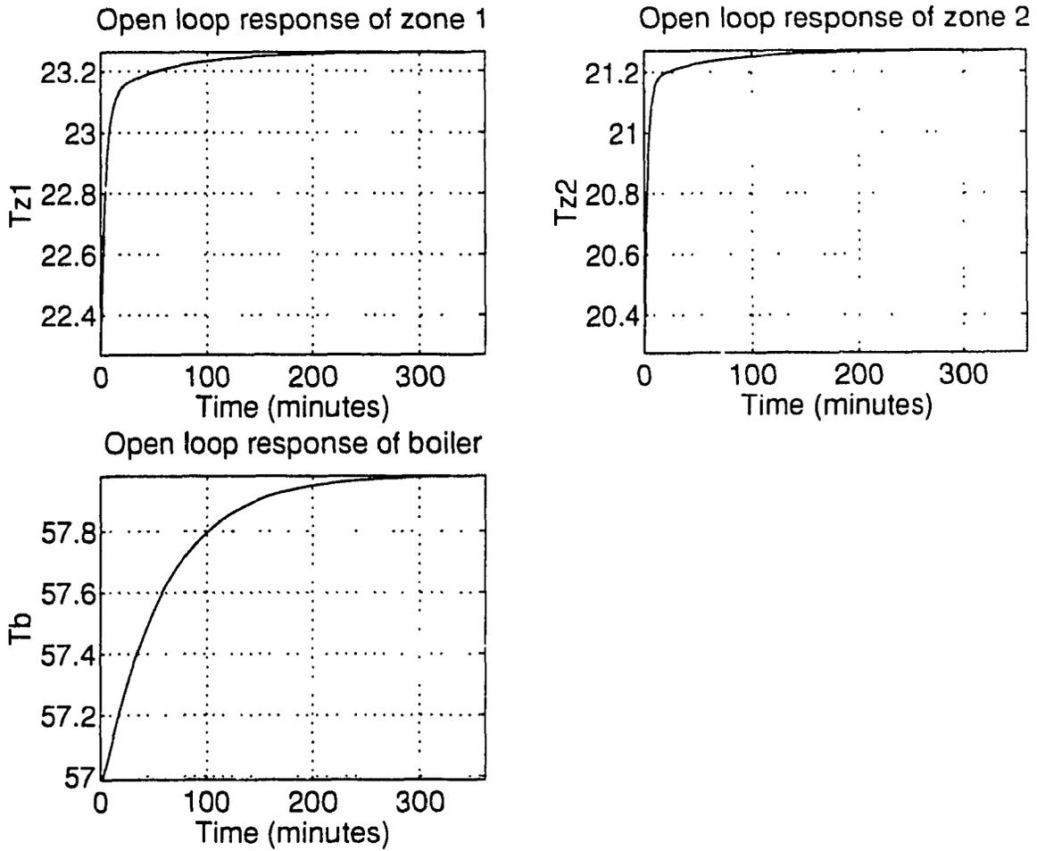
Figure 3.4: Open-loop response of the system when the initial conditions are perturbed by 1.0 deg C.
