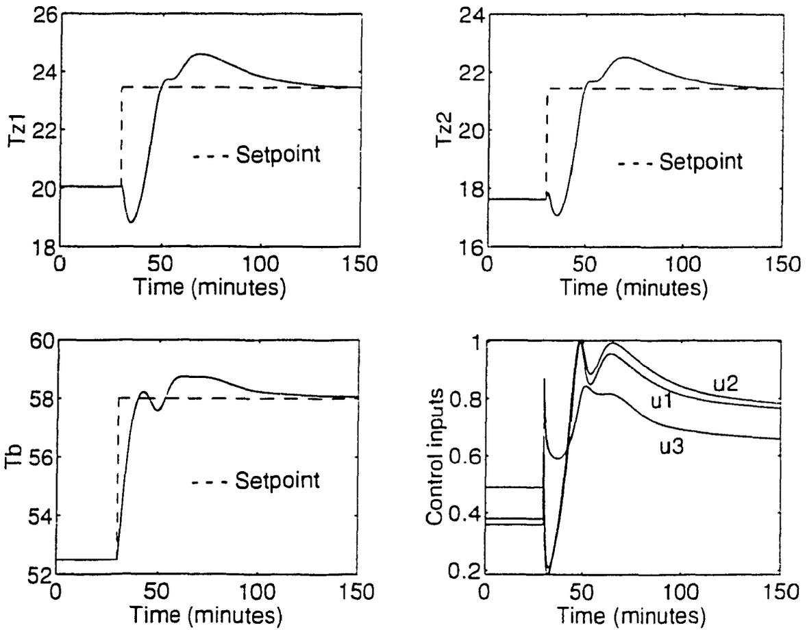
Figure 5.21: Closed-loop response showing the effect of step changes in the operating point with adaptive controller.
