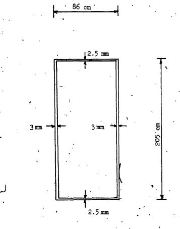
Fig. 4.4 — Maximum Gaps Between Frame and Door Specimen.
