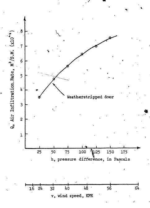
Fig. 6.1 — Door Air Infiltration Characteristics.
