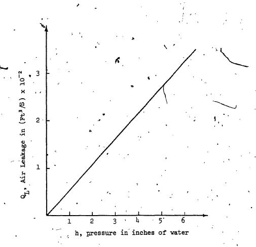
Fig. 3.4 — Air Leakage-Pressure Variation.
