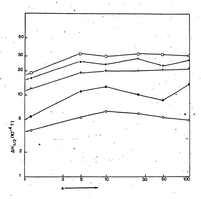
Figure 12: Log  $\Delta H_{1/2}$  vs.  $\log \alpha$ , for  $\alpha \leq 100$  in  $Yb_{0.5}Y_{0.5}$ CH. A: $\Box$ , B:0. C:a. D:\*. Sum:+.
