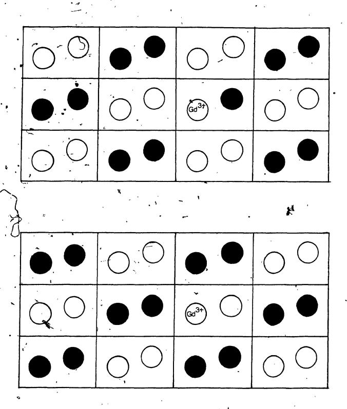
Figure 7: Two possible configurations A (top) and B (bottom) in the case of alternating unit cells. O: Yb3+.
