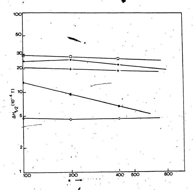
Figure 13: Log  $\Delta H_{1/2}$  vs.  $\log \alpha$ , for  $\alpha \ge 100$  in Yb  $_{0.5}^{\text{Y}}_{0.5}^{\text{CH.A:D}}$ , B:0. C:0. D:+. Sum:+.
