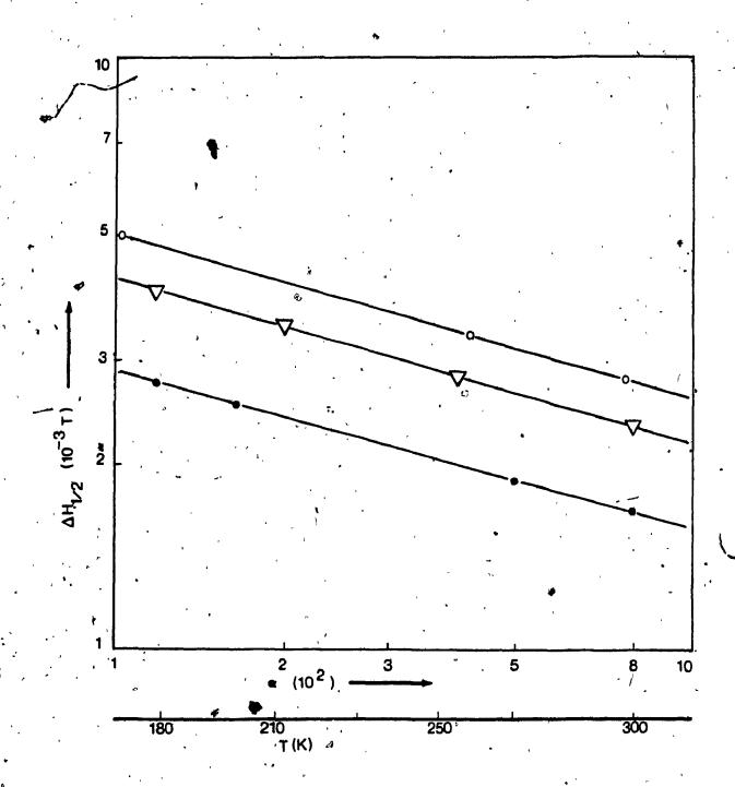
Figure 14: Log of both the experimental and simulated linewidths vs.  $\log \alpha$  and temperature. •: Misra and Sharp<sup>1</sup>, o: Malhotra et al.<sup>2</sup>,  $\nabla$ : Simulated
