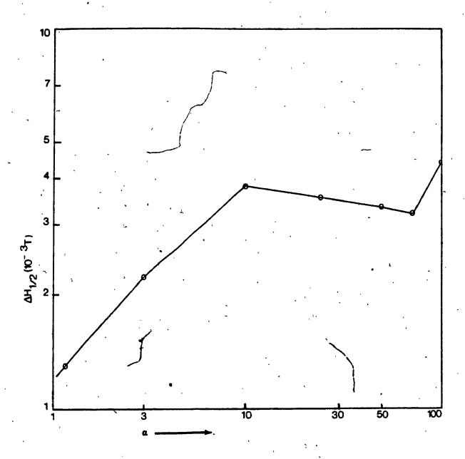
Figure 11: Log-log plot of linewidth vs. relaxation time ratio ∞≤100 in YbCH.
