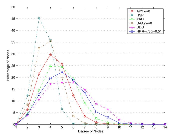
Figure 4.20: Histogram of degrees of nodes for different spanning subgraphs
