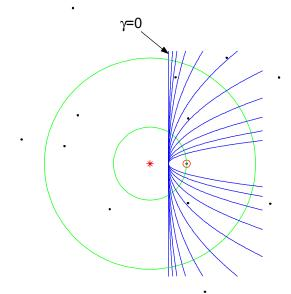
Figure 3.3: Definition of parabola when  $\alpha = 0.5$ . This picture shows  $x = \gamma a_m y^2 + b$  family of parabolas with  $\alpha = 0.5$  and  $\gamma = 0, 1, 2, 4, ..., 512$ . At the beginning the value of a is 0 and parabola starts as a line, then as the value of  $\gamma$  increases parabola gets narrower.
