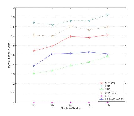
Figure 4.19: Power Stretch Factor for graphs with various numbers of nodes
