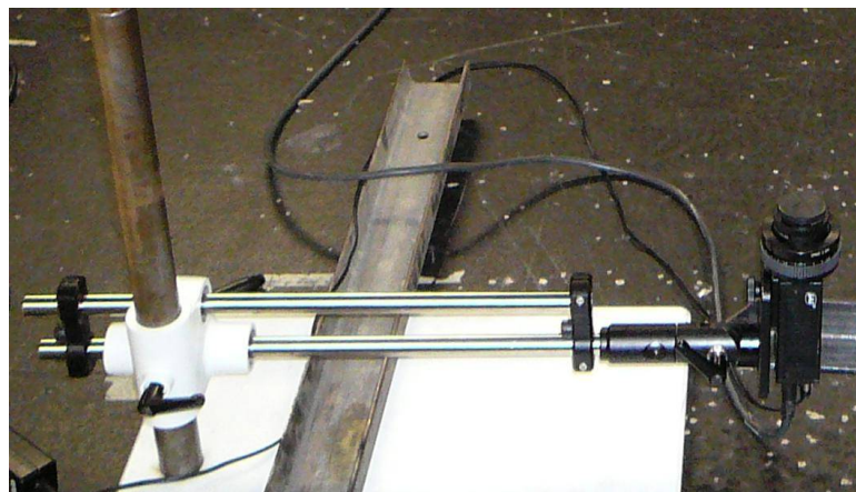
Figure 2.10: CCD camera positioning structure.
