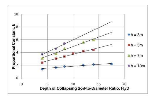
Figure 5.1: Proportional constant (k) vs. H<sub>s</sub>/D ratio for different radius of wetting front (h)
