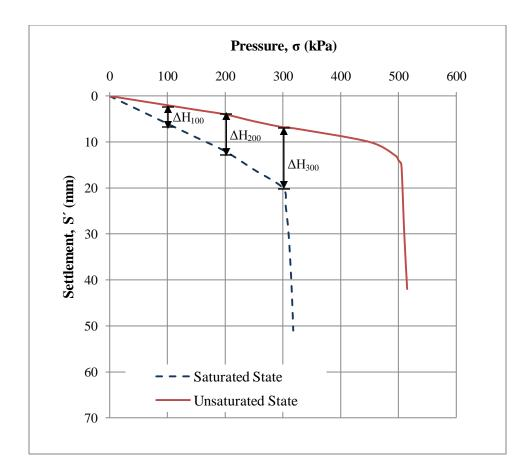
Figure 2.10: Typical load settlement curves of a bearing plate in collapsible soils (saturated and unsaturated) (Grigoryan, 1997)
