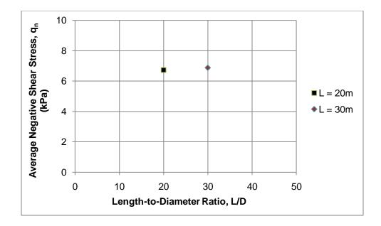
Figure 4.22: Average negative shear stress  $(q_n)$  vs length-to-diameter ratio (L/D), when h = 3 m,  $H_s/D = 4$ , and  $C_p = 5\%$
