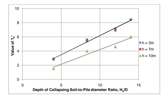
Figure 5.11: Value of  $I_a$  for different H<sub>s</sub>/D and h, when  $C_p = 5-10\%$
