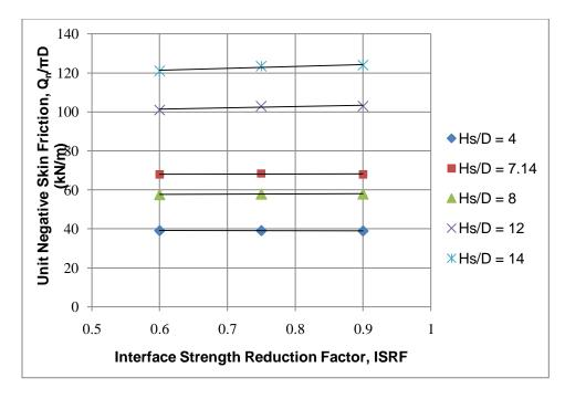
Figure 4.40: Effect of Interface Strength Reduction Factor (ISRF) on unit negative skin friction ( $Q_n/\pi D$ ), where h = 3 m and  $C_p = 5\%$
