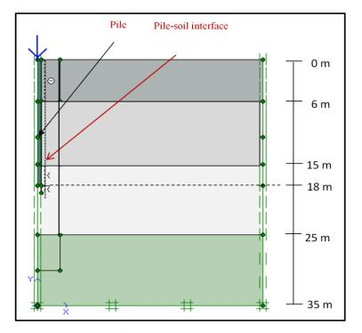
Figure 3.9: Numerical model of pile load test in Voldogon Experimental Region-2
