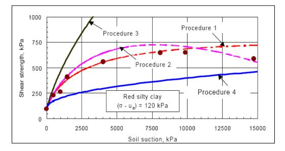
Figure 2.24: Comparison of the measured and the predicted shear strength values for red silty clay using four different procedures (Vanapalli and Fredlund 2000)
