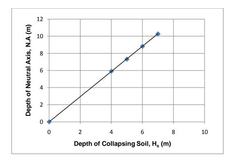
Figure 4.36: Depth of Neutral Axis (N.A) vs.  $H_s$ , when h = 3 m, and  $C_p = 5\%$
