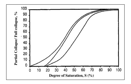
Figure 2.13: Partial collapse curves for three collapsible silts (Mahmoud, 1991)
