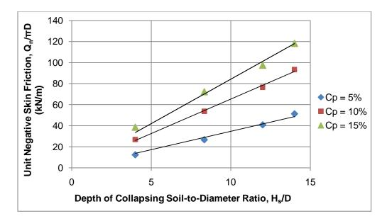
Figure 4.48: Unit negative skin friction  $(Q_n/\pi D)$  vs. H<sub>s</sub>/D ratio, when h = 3 m
