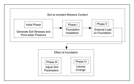
Figure 3.14: Principle/framework of the proposed staged construction
