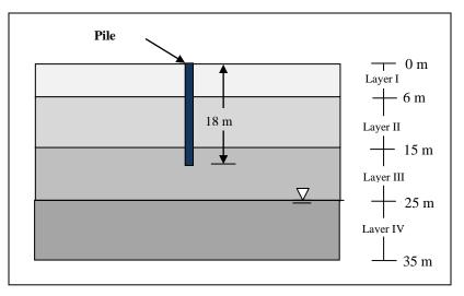
Figure 3.8: Soil profile at Volgodon Experimental Region-2
