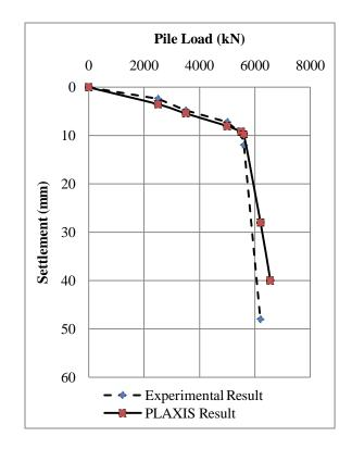
Figure 3.10: Pile load displacement curves at Volgodon Experimental Region-1
