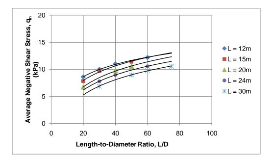
Figure 4.21: Average negative shear stress  $(q_n)$  vs. length-to-diameter ratio (L/D), when h = 3m,  $H_s = 4m$  and  $C_p = 5\%$
