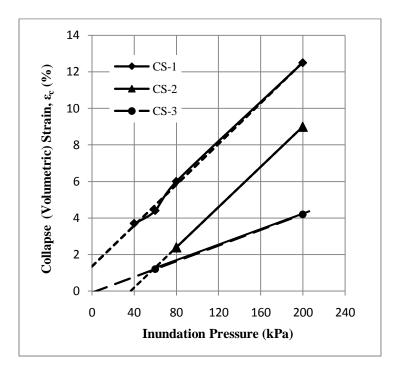
Figure 3.18: Effect of inundation pressure on collapse (volumetric) strain (after Mashhour, 2009)
