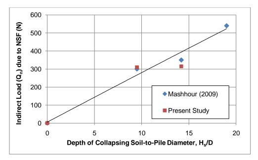
Figure 3.21: Effect of depth of collapsing soil-to-diameter ratio  $(H_s/D)$  on indirect load  $(Q_n)$  due to NSF (Test – 3 in Table 3.17)
