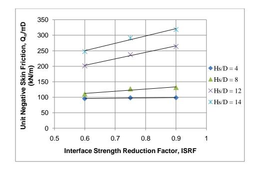
Figure 4.42: Effect of Interface Strength Reduction Factor (ISRF) on unit negative skin friction ( $Q_n/\pi D$ ), where h = 7 m and  $C_p = 5\%$
