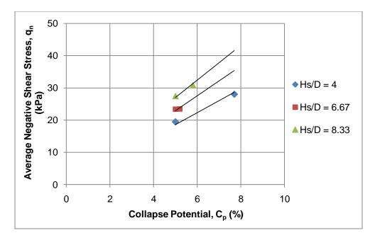
Figure 4.47: Average negative shear stress  $(q_n)$  vs. collapse potential  $(C_p)$ , when h = 10 m
