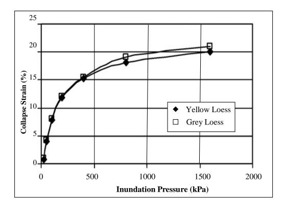
Figure 2.12: Effect of inundation pressure on collapse strain (Nouaouria et al., 2008)
