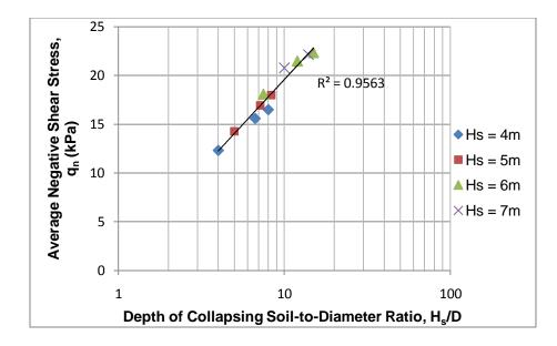
Figure 4.33: Average negative shear stress  $(q_n)$  vs.  $H_s/D$  ratio, when h = 5 m, and  $C_p = 5\%$
