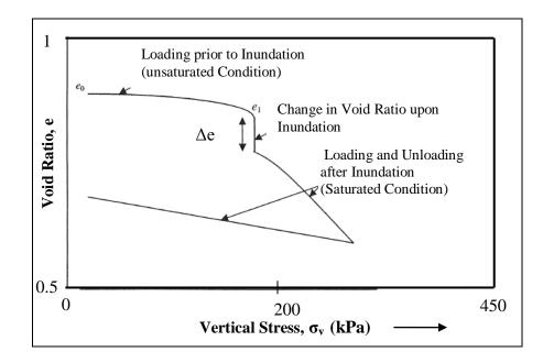
Figure 2.14: Single curve oedometer test to evaluate collapse potential (C<sub>p</sub>)
