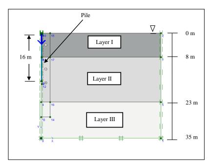
Figure 3.12: Numerical model of pile load test in wetted collapsible loess
