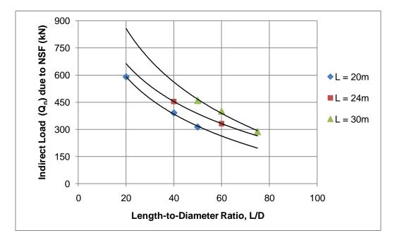
Figure 4.19: Indirect load (Q<sub>n</sub>) due to NSF vs. length-to-diameter ratio (L/D), when h = 3 m,  $H_s = 7$  m and  $C_p = 10\%$
