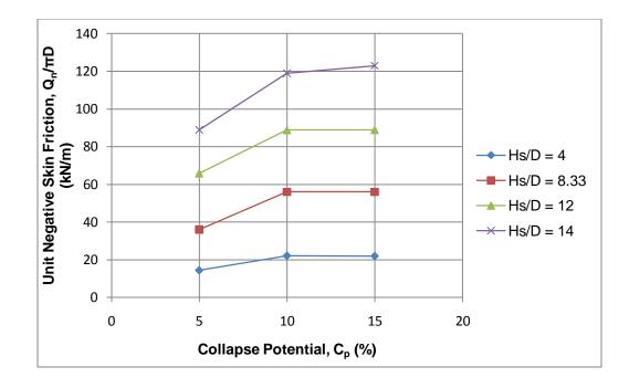
Figure 4.56: Effect of collapse potential (C<sub>p</sub>) on unit negative skin friction (Q<sub>n</sub>/ $\pi$ D), when h = 10 m
