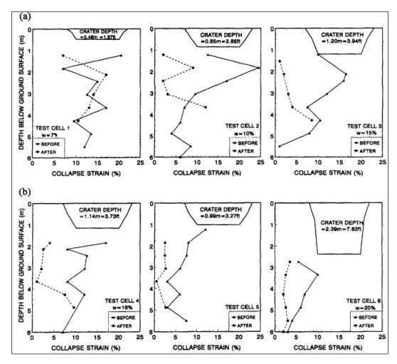
Figure 2.9: Collapse strain profiles before and after dynamic compaction (Rollins et al., 1998)
