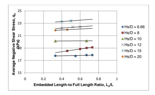
Figure 4.29: Average negative shear stress  $(q_n)$  vs  $(L_e/L)$  Ratio, when h = 3 m, and  $C_p = 10\%$
