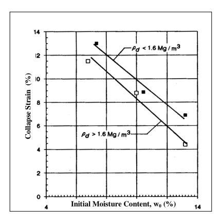
Figure 2.5: Effect of initial water content on collapse strain (Fredlund and Gan, 1995)
