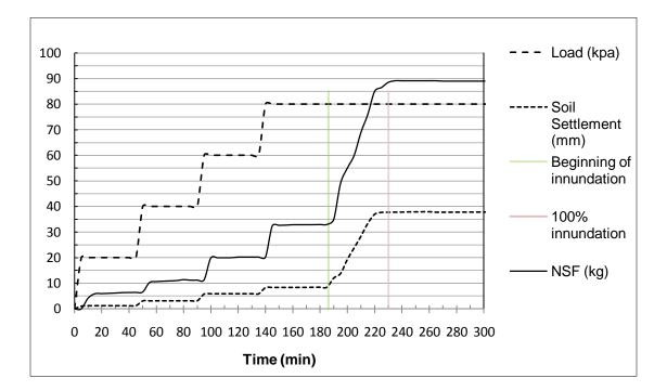
Figure 2.31: Surcharge, soil settlement and negative skin friction versus time for  $C_P = 12.5\%$  (Mashhour, 2009)
