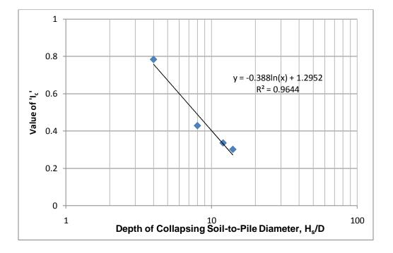
Figure 5.10: Value of  $I_c$  for different depth of collapsing soil-to-pile diameter ratio  $(H_s\!/D)$
