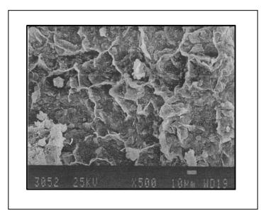
Figure 2.2: Honeycomb type of microstructure of loess like sediments (Klukanova and Frankovska, 1995)
