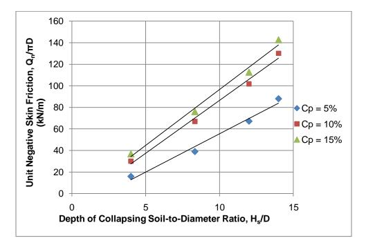
Figure 4.49: Unit negative skin friction  $(Q_n/\pi D)$  vs.  $H_s/D$  ratio, when h = 7 m
