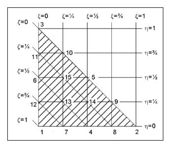
Figure 3.2: Numbering of nodes in a 15-node triangular element
