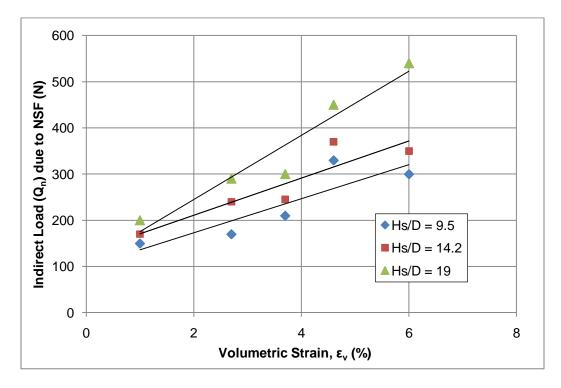
Figure 4.5: Effect of volumetric strain  $(\varepsilon_v)$  on negative skin friction
