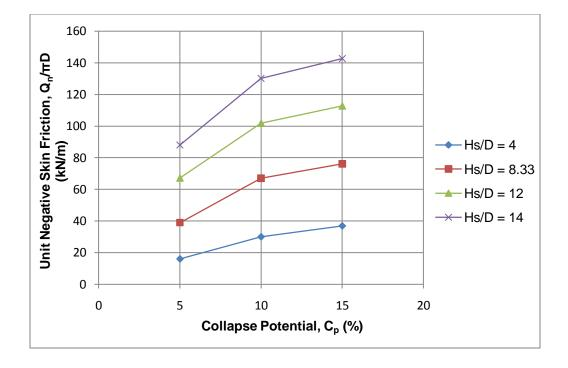
Figure 4.55: Effect of collapse potential (C<sub>p</sub>) on unit negative skin friction (Q<sub>n</sub>/ $\pi$ D), when h = 7 m
