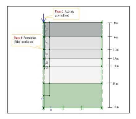
Figure 3.15: Staged Construction: Soil at Constant Moisture Content
