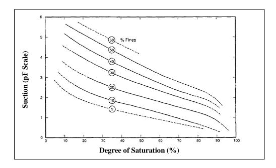
Figure 2.21: Soil Water Characteristic Curve for soils having different percent fines (Kenneth et al., 1993)
