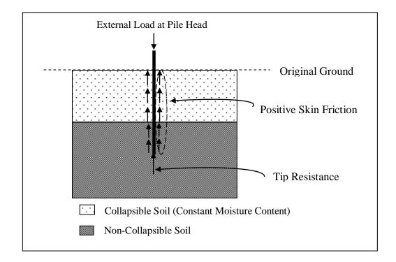
Figure 1.1: Load transfer mechanism of a single pile in unsaturated collapsible soil at constant moisture content
