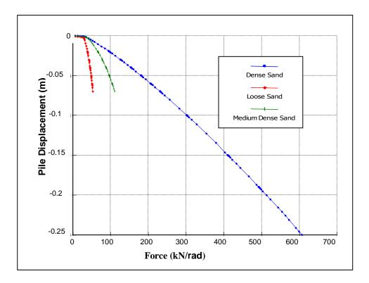
Figure 3.6: Present study - Load displacement curves for a 10 m long pile with 0.5 m diameter in dense, medium dense and loose sands
