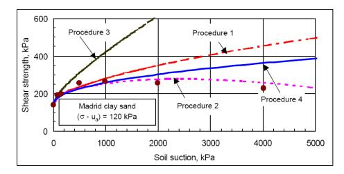
Figure 2.25: Comparison of the measured and the predicted shear strength values for Madrid clay sand using four different procedure (Vanapalli and Fredlund 2000)
