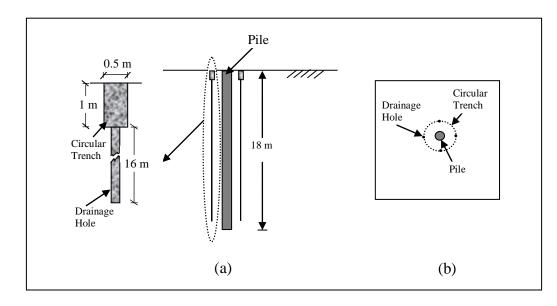
Figure 3.26: Method of local wetting of collapsible soil using circular trench and drainage holes at Volgodon-2; (a) Profile of the test setup, (b) Plan view of the test setup
