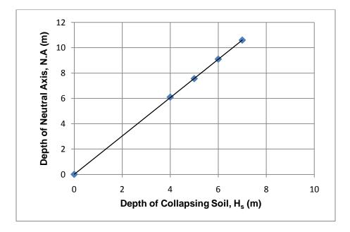
Figure 4.37: Depth of Neutral Axis (N.A) vs.  $H_s$ , when h = 3 m, and  $C_p = 10\%$
