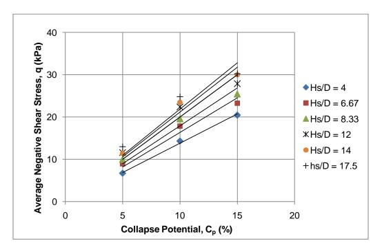
Figure 4.44: Average negative shear stress  $(q_n)$  vs. collapse potential  $(C_p)$ , when h = 3 m
