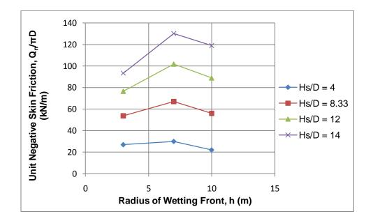
Figure 4.52: Effect of radius of wetting front (h) on Unit negative skin friction  $(Q_n/\pi D)$ , when  $C_p = 10\%$
