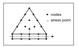
Figure 3.3: Connection between a 15 node triangular element and an interface element
