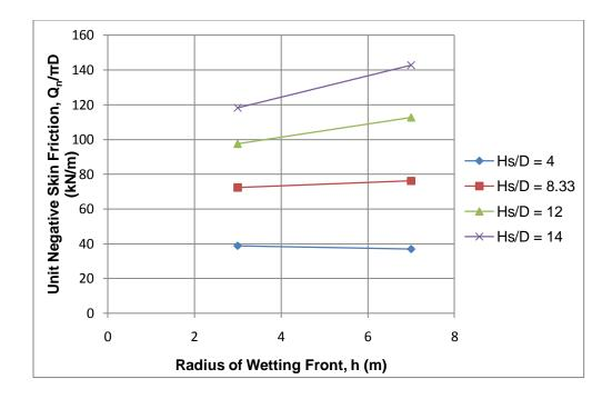
Figure 4.53: Effect of radius of wetting front (h) on unit negative skin friction  $(Q_n/\pi D)$ , when  $C_p = 15\%$
