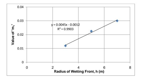
Figure 5.6: Effect of radius of wetting (h) on the value of 'm<sub>1</sub>'
