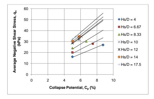
Figure 4.46: Average Negative Shear Stress  $(q_n)$  vs. Collapse Potential  $(C_p)$ , when h = 7 m
