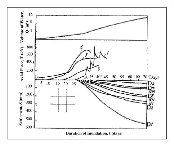
Figure 2.29: Experimental results: the amount of water discharge (Q), the axial forces (T) at different pile sections (1, 4, 5 & 6), and the settlements (S) of piles (NI and NII) & depth markers (D1 through D6) with time (Grigoryan and Grigoryan 1975)
