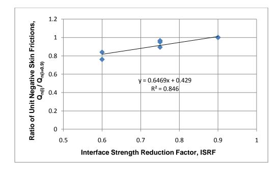
Figure 5.8: Effect of Interface Strength Reduction Factor (ISRF) on unit negative skin friction ( $Q_n/\pi D$ ), when  $H_s/D = 8$
