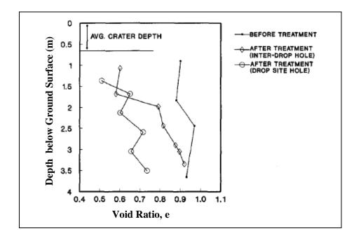
Figure 2.8: Void ratio before and after dynamic compaction (Rollins et al., 1994)
