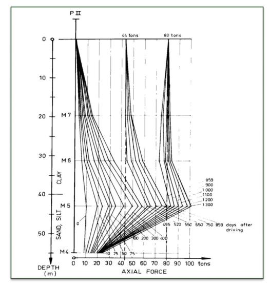
Figure 2.26 Vertical load distribution in piles PI at various times after the driving (Fellenius 1972)
