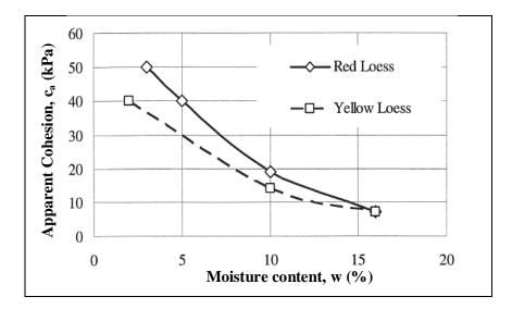
Figure 2.4: The effect of moisture content on apparent cohesion of Khon Kaen loess (Udomchoke, 1991)
