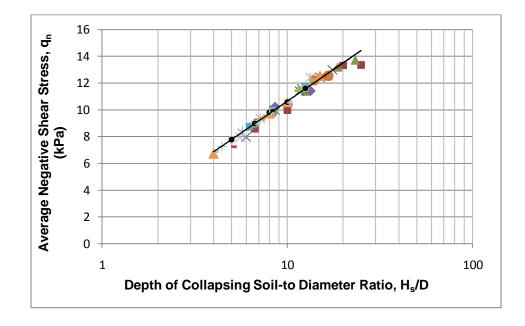
Figure 4.30: Average negative shear stress  $(q_n)$  vs.  $H_s/D$  ratio, for different Embedded Length-to-Full Length ratio  $(L_e/L)$ , when h = 3 m, and  $C_p = 5\%$
