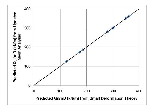
Figure 3.27: Comparison between unit negative skin friction  $(Q_n/\pi D)$  values predicted from small deformation theory and updated mesh analysis
