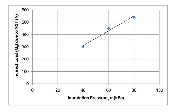
Figure 4.1: Effect of inundation pressure ( $\sigma$ ) on indirect load (Q<sub>n</sub>) due to negative skin friction (NSF), when H<sub>s</sub>/D = 19.8
