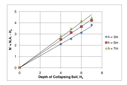
Figure 5.4: Effect of depth of collapsing soil (H<sub>s</sub>) on N', when  $C_p = 10\%$
