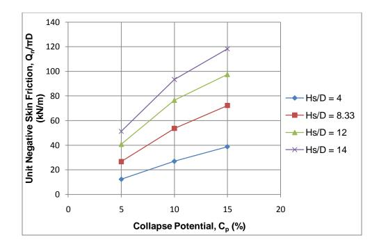
Figure 4.54: Effect of collapse potential (C<sub>p</sub>) on unit negative skin friction (Q<sub>n</sub>/ $\pi$ D), when h = 3 m
