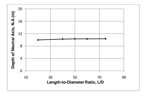
Figure 4.27: Depth of neutral axis (N.A) vs length-to-diameter ratio (L/D), when h = 3 m,  $H_s = 7 \text{m}$  and  $C_p = 5\%$
