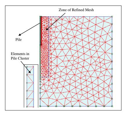
Figure 3.4: Generated Mesh in an axi-symmetric model
