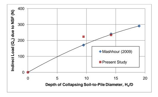
Figure 3.22: Effect of depth of collapsing soil-to-diameter ratio  $(H_s/D)$  on indirect load  $(Q_n)$  due to NSF (Test – 4 in Table 3.17)
