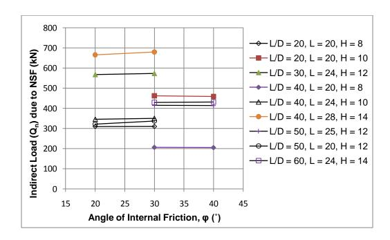
Figure 4.14: Indirect load (Q<sub>n</sub>) due to NSF vs. angle of internal friction ( $\phi$ ), when h=7m, and C<sub>p</sub> = 5%
