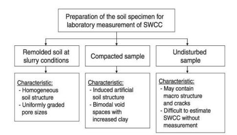
Figure 2.19: Effect of initial conditions of the soil specimens on the SWCC (Fredlund and Houston, 2009)
