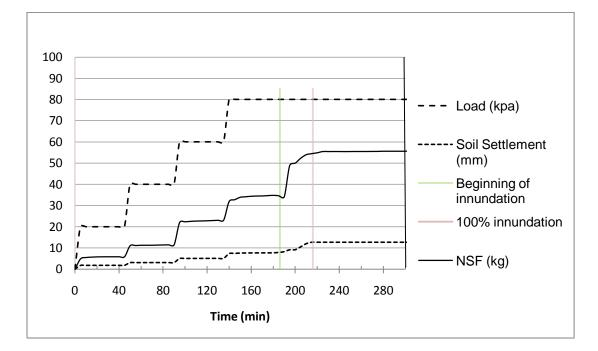
Figure 2.30: Surcharge, soil settlement and negative skin friction with time for  $C_p = 4.2\%$  (Mashhour, 2009)
