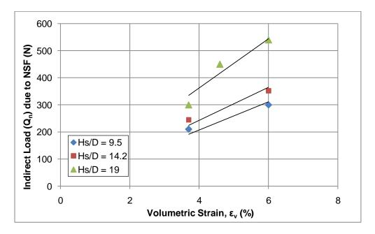
Figure 4.4: Effect of volumetric strain  $(\epsilon_v)$  on indirect load  $(Q_n)$  due to NSF
