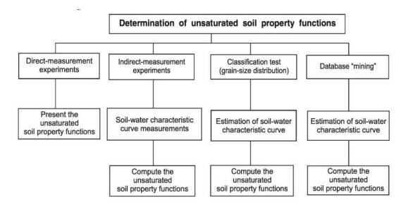
Figure 2.20: Different approaches in Determining Unsaturated Soil Property Functions (Fredlund and Houston, 2009)
