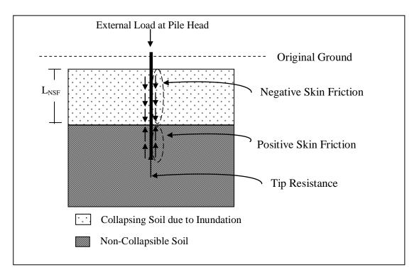
Figure 1.2: Load transfer mechanism of a single pile in collapsible soil (near the ground surface) during inundation
