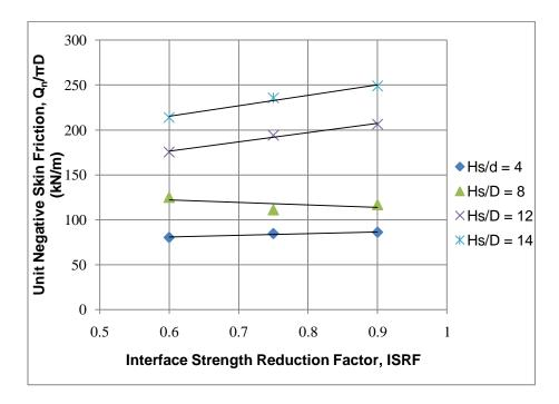
Figure 4.41: Effect of Interface Strength Reduction Factor (ISRF) on unit negative skin friction ( $Q_n/\pi D$ ), where h = 3 m and  $C_p = 10\%$
