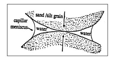
Figure 2.3: Bond in unsaturated soil by capillary action (Dudley, 1970)
