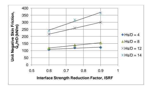
Figure 4.43: Effect of Interface Strength Reduction Factor (ISRF) on unit negative skin friction ( $Q_n/\pi D$ ), where h = 10 m and  $C_p = 5\%$
