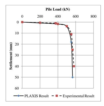
Figure 3.13: Pile load displacement curve at Nikopol Experimental Region
