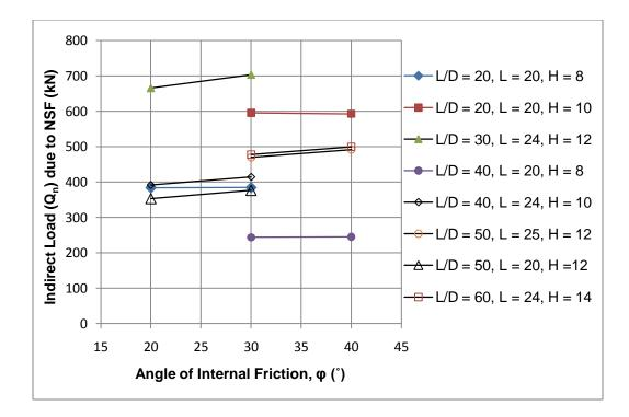
Figure 4.15: Indirect load (Q<sub>n</sub>) due to NSF vs. angle of internal friction ( $\phi$ ), when h=10m, and C<sub>p</sub> = 5%
