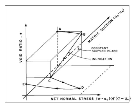
Figure 2.15: Typical compression curve for collapsible soil (Tadepalli and Fredlund, 1991)
