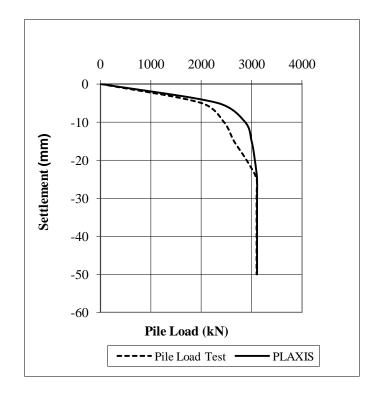
Figure 3.7: Load displacement curves of a pile in overconsolidated stiff clay (OCR = 6.25)
