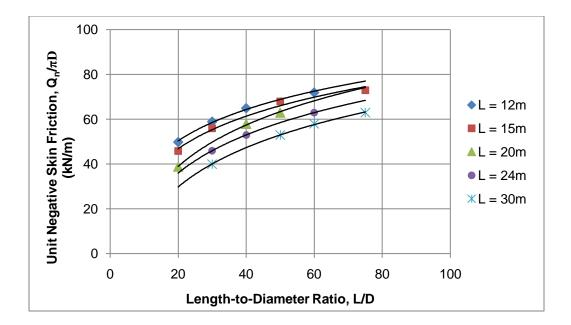
Figure 4.20: Unit negative skin friction  $(Q_n/\pi D)$  vs length-to-diameter ratio (L/D), when h = 3 m, H<sub>s</sub> = 4 m and C<sub>p</sub> = 5%
