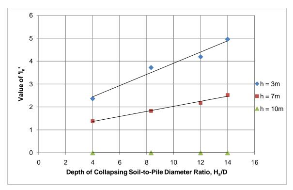
Figure 5.12: Value of  $I_a$  for different  $H_s/D$  and h, when  $C_p$  = 10–15%
