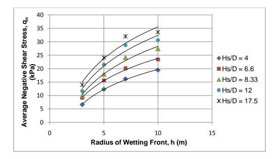
Figure 4.39: Average negative shear stress (qn) vs. radius of wetting front (h) when Cp = 5%
