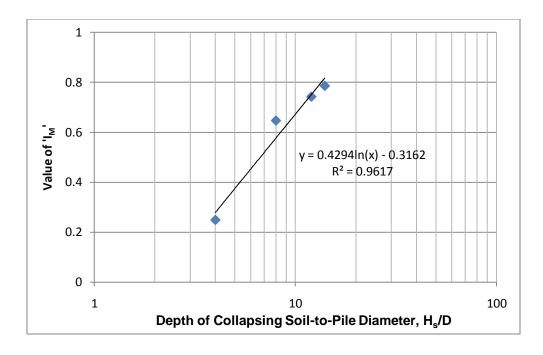
Figure 5.9: Value of  $I_{\rm M}$  for different depth of collapsing soil-to-pile diameter ratio  $(H_{s}\!/D)$
