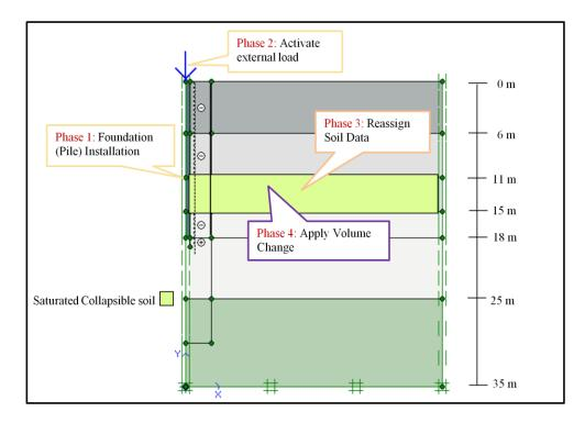
Figure 3.16: Staged construction: collapsible soil subjected to inundation
