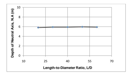
Figure 4.26: Depth of neutral axis (N.A) vs length-to-diameter ratio (L/D), when h = 3 m,  $H_s = 4m$  and  $C_p = 5\%$
