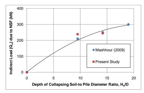
Figure 3.19: Effect of depth of collapsing soil-to-diameter  $(H_s/D)$  on indirect load  $(Q_n)$  due to NSF (Test -1 in table 3.17)
