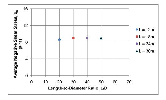
Figure 4.23: Average negative shear stress (q<sub>n</sub>) vs length-to-diameter ratio (L/D), when h = 3 m,  $H_s/D = 6.6$ , and  $C_p = 5\%$
