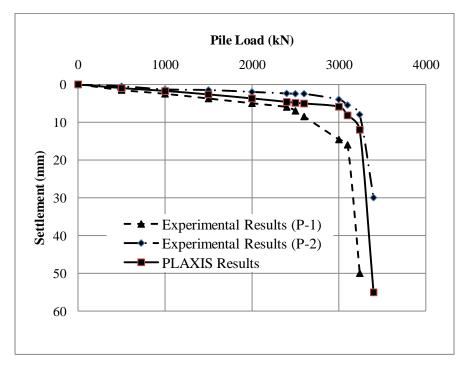
Figure 3.11: Pile load displacement curves at Volgodon Experimental Region-2
