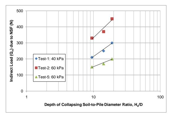
Figure 4.2: Effect of H<sub>s</sub>/D ratio on indirect load (Q<sub>n</sub>) due to NSF
