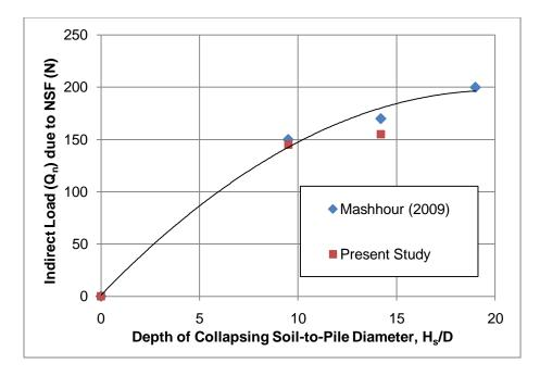
Figure 3.23: Effect of depth of collapsing soil-to-diameter ratio  $(H_s/D)$  on indirect load  $(Q_n)$  due to NSF (Test – 5 in Table 3.17)
