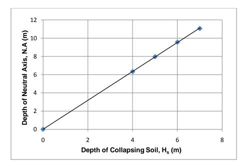
Figure 4.38: Depth of Neutral Axis (N.A) vs.  $H_s$ , when h = 3 m, and  $C_p = 15\%$
