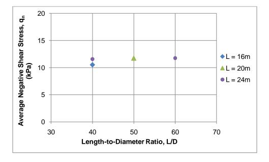
Figure 4.25: Average negative shear stress (q<sub>n</sub>) vs length-to-diameter ratio (L/D), when h = 3 m,  $H_s/D = 12.5$ , and  $C_p = 5\%$
