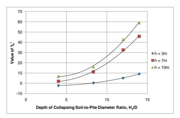
Figure 5.13: Value of  $I_b$  for different  $H_s/D$  and h, when  $C_p$  = 5–10%
