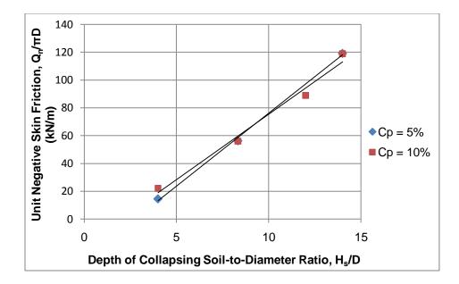
Figure 4.50: Unit negative skin friction  $(Q_n/\pi D)$  vs. H<sub>s</sub>/D ratio, when h = 10 m
