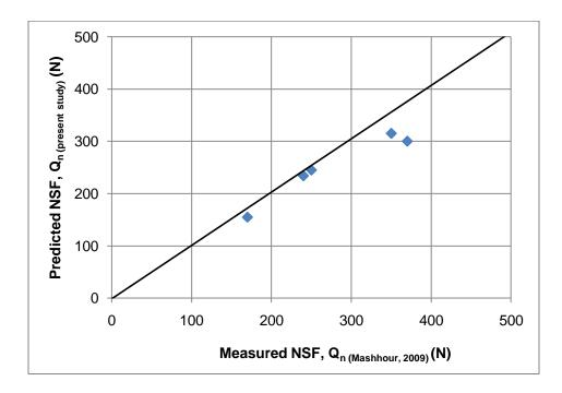
Figure 3.25: Comparison of numerical and experimental results (collapse of three-quarter depth from bottom of the collapsible soil)
