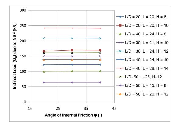
Figure 4.12: Indirect load (Q<sub>n</sub>) due to NSF vs. angle of internal friction ( $\phi$ ), when h=3m, and C<sub>p</sub> = 5%
