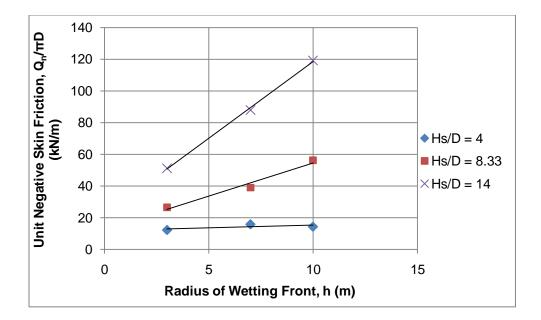
Figure 4.51: Effect of radius of wetting front (h) on unit negative skin friction  $(Q_n/\pi D)$ , when  $C_p = 5\%$
