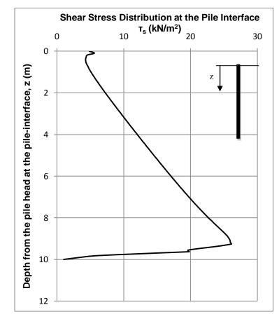
Figure 3.5: Present study - Typical shear stress distribution on pile-soil interface
