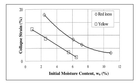
Figure 2.6: Effect of initial water content on collapse strain (Udommchoke, 1991)
