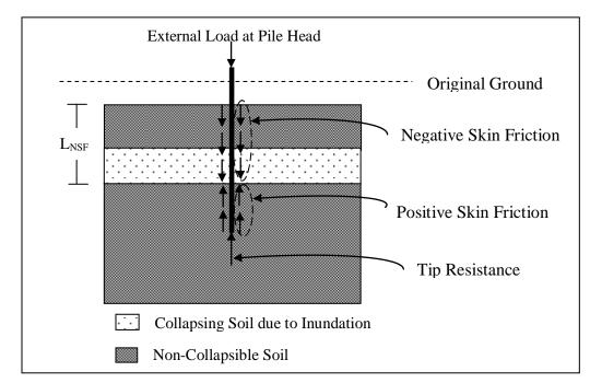
Figure 1.3: Load transfer mechanism of a single pile in collapsible soil (at depth) during inundation
