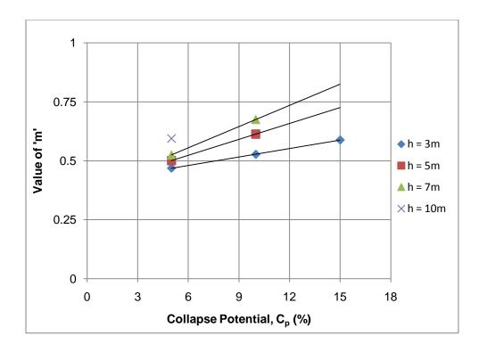
Figure 5.5: Effect of collapse potential (C<sub>p</sub>) on the value of 'm'
