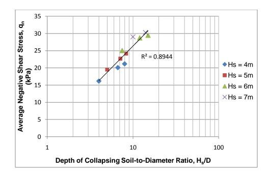
Figure 4.34: Average negative shear stress (q<sub>n</sub>) vs.  $H_s/D$  ratio, when h = 7 m, and  $C_p = 5\%$
