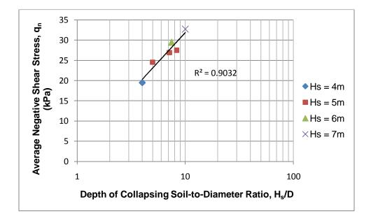
Figure 4.35: Average negative shear stress ( $q_n$ ) vs. H<sub>s</sub>/D ratio, when h = 10 m, and  $C_p = 5\%$
