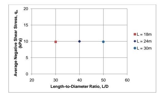
Figure 4.24: Average negative shear stress (q<sub>n</sub>) vs length-to-diameter ratio (L/D), when h = 3 m,  $H_s/D = 8.33$ , and  $C_p = 5\%$
