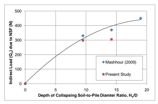
Figure 3.20: Effect of depth of collapsing soil-to-diameter ratio (H<sub>s</sub>/D) on indirect load (Q<sub>n</sub>) due to NSF (Test-2 in Table 3.17)
