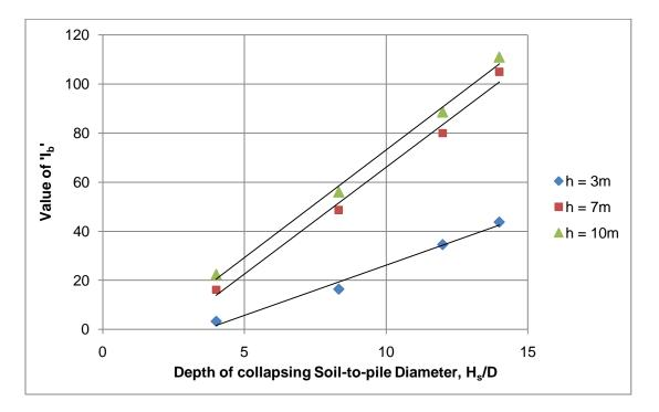
Figure 5.14: Value of  $I_b$  for different  $H_s/D$  and h, when  $C_p = 10-15\%$
