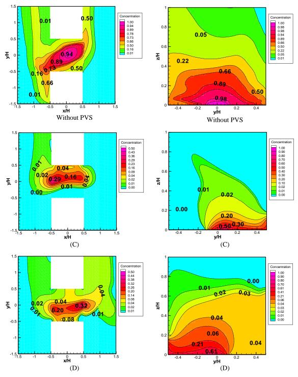
**Figure 4.30** Normalized pollution concentration: AR = 2, wind direction = 0 (degree), wind velocity = 1 (m/s), and fan pressure = 100 (Pa) for various PVS strategies (Left) Horizontal section 1.5 above the ground (Right) Vertical section in middle of the studied street canyon
