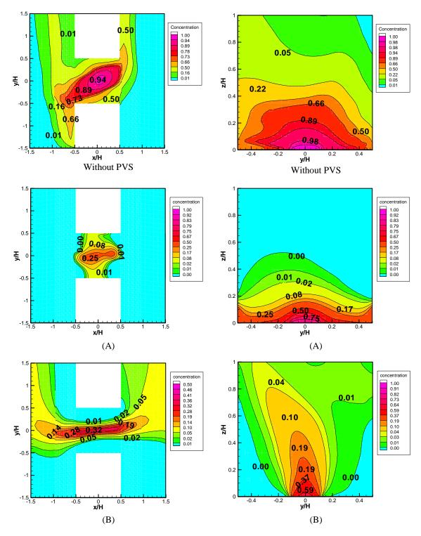
**Figure 4.29** Normalized pollution concentration: AR = 2, wind direction = 0 (degree), wind velocity = 1 (m/s), and fan pressure = 100 (Pa) for various PVS strategies (Left) Horizontal section 1.5 above the ground (Right) Vertical section in middle of the studied street canyon
