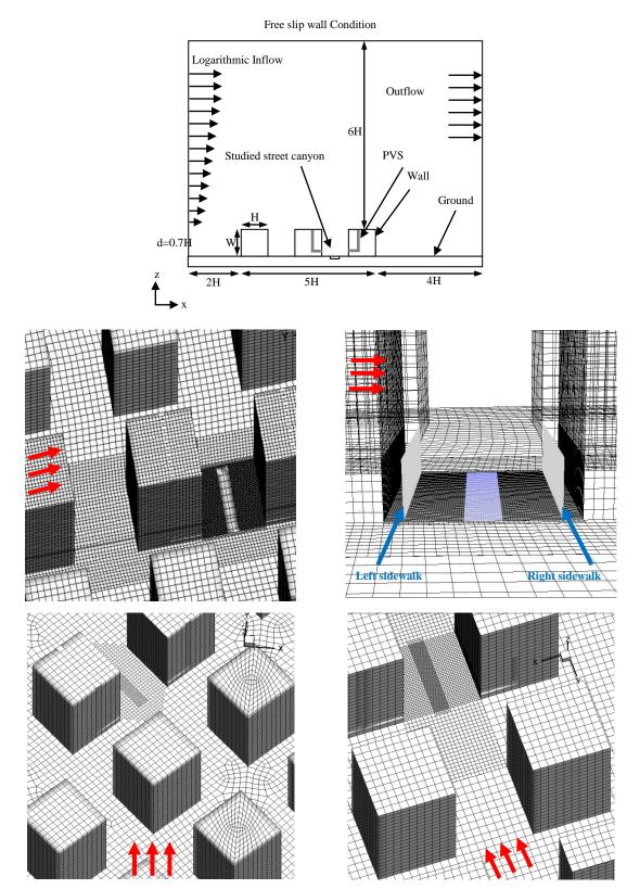
Figure 3.9 Simulation study domains (direction of prevailing wind is presented with red arrows)
