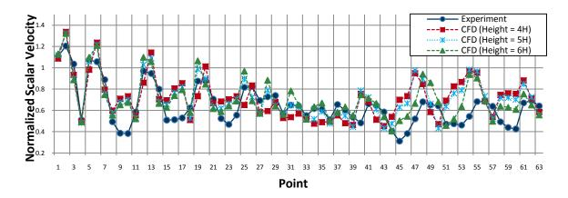
Figure 4.4 Comparison between measurement and CFD with different domain height
