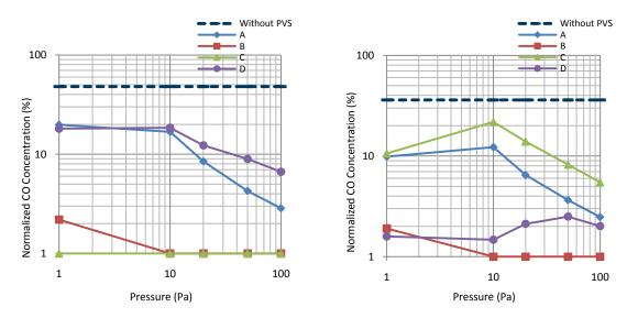
Figure 4.25 Normalized CO concentration within pedestrian plane for various PVS combinations (Left) left sidewalk (Right) right sidewalk
