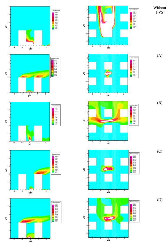
Figure 4.31 Normalized pollution concentration in (Left) a vertical section (Right) a horizontal section 1.5 above the ground for various PVS strategies
