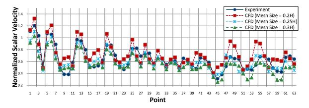
Figure 4.2 Comparison between measurement and CFD with different mesh size
