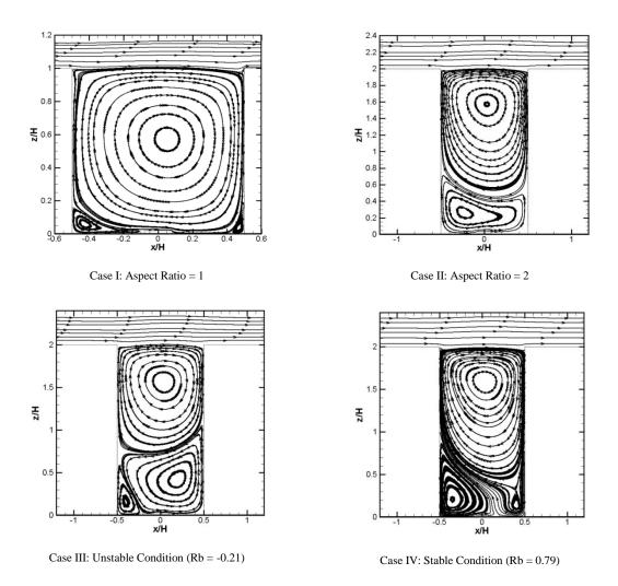
Figure 3.11 Streamline through street canyons with different characteristics
