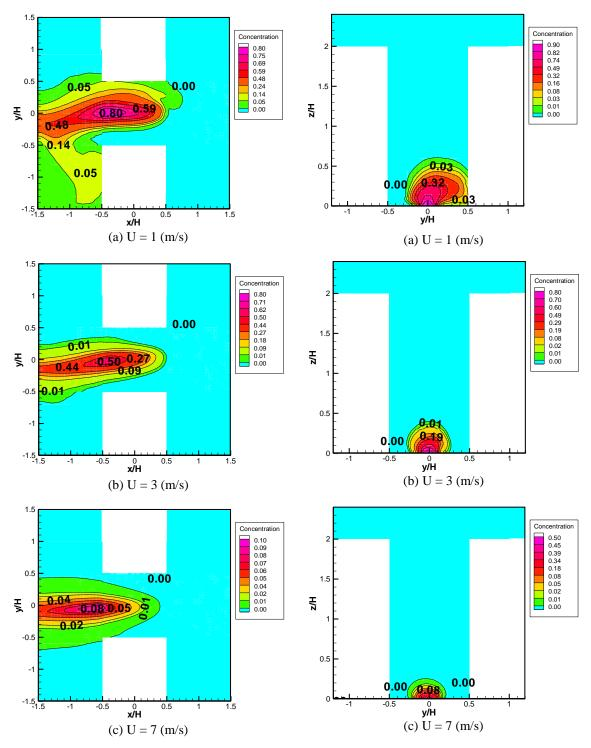
**Figure 4.21** Normalized pollution concentration: wind direction = 0 (degree) and AR = 2 (Left) Horizontal section 1.5 above the ground (Right) Vertical section in middle of the studied street canyon
