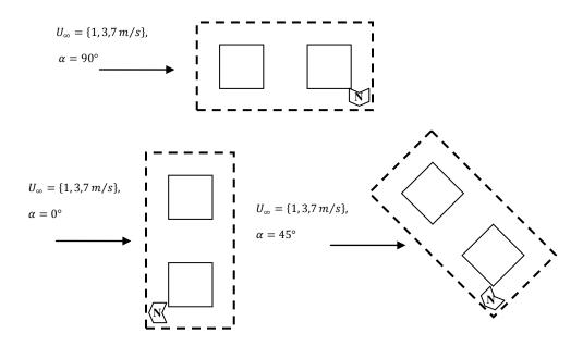
**Figure 3.10** Top view of various wind velocities ( $U_{\infty} = 1, 3, 7 m/s$ ) and directions ( $\alpha = 0, 45, 90^{\circ}$ ) around the target street canyon (north -south)
