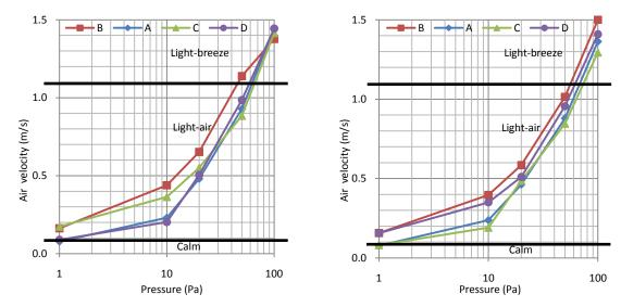
**Figure 4.27** WCI within pedestrian plane for various PVS combinations (Left) left sidewalk (Right) right sidewalk
