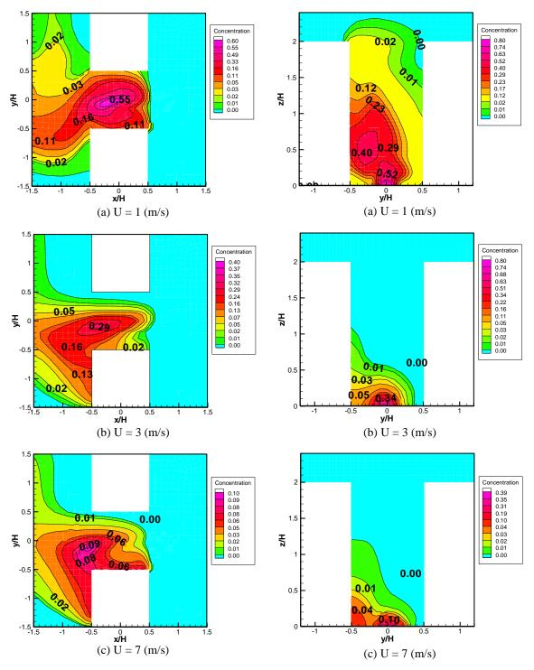
**Figure 4.23** Normalized pollution concentration: wind direction = 45 (degree) and AR = 2 (Left) Horizontal section 1.5 above the ground (Right) Vertical section in middle of the studied street canyon
