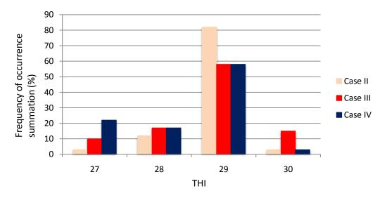
**Figure 4.15** Temperature-humidity index (THI) frequency of occurrence summation for AR=2 (case II) albedo of buildings' surface (case III) and changing albedo of road and pavement (case IV)
