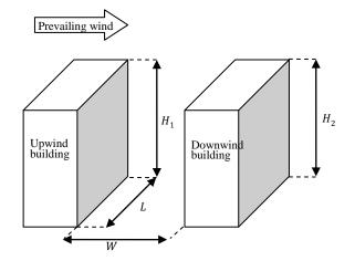
**Figure 2.1** Street canyon characteristic; Step-down  $(H_1 > H_2)$  - Step-up  $(H_2 > H_1)$  -Symmetric  $(H_1 = H_2)$
