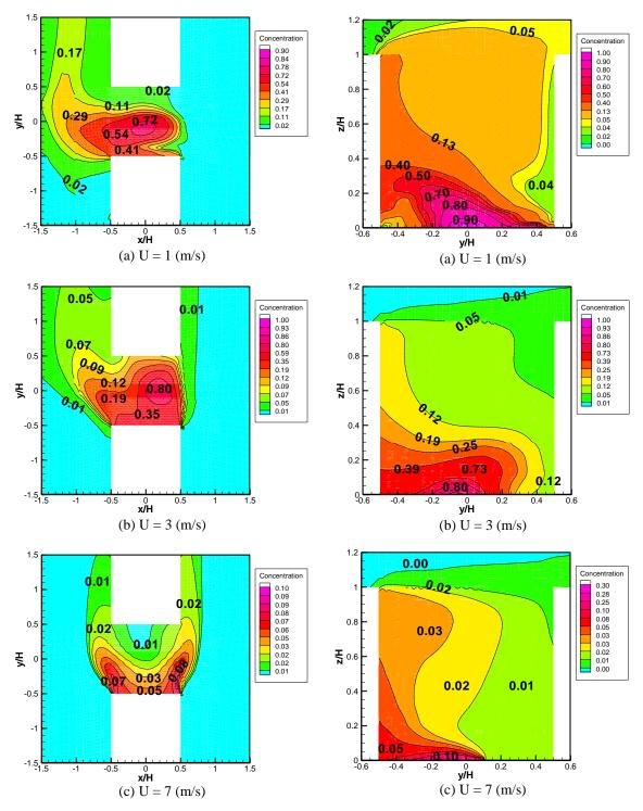
**Figure 4.18** Normalized pollution concentration: wind direction = 90 (degree) and AR = 1 (Left) Horizontal section 1.5 above the ground (Right) Vertical section in middle of the studied street canyon
