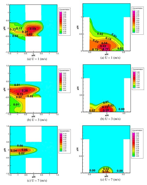
**Figure 4.20** Normalized pollution concentration: wind direction = 0 (degree) and AR = 1 (Left) Horizontal section 1.5 above the ground (Right) Vertical section in middle of the studied street canyon
