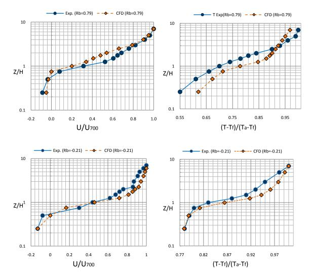
Figure 4.7 Comparison between measurement and CFD (Left) Velocity (Right) Temperature
