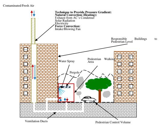
Figure 3.2 New design approach: Pedestrian Ventilation System (PVS)
