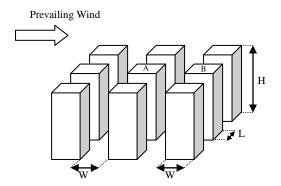
Figure 3.7 Layout of a 3 × 3 array of homogeneous buildings
