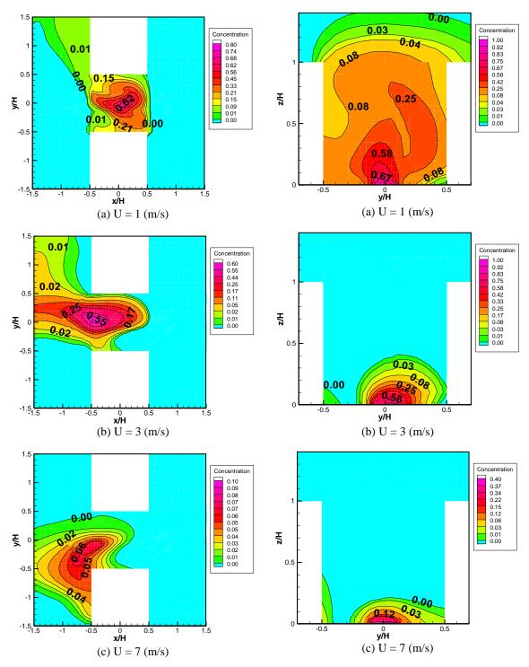
**Figure 4.22** Normalized pollution concentration: wind direction = 45 (degree) and AR = 1 (Left) Horizontal section 1.5 above the ground (Right) Vertical section in middle of the studied street canyon
