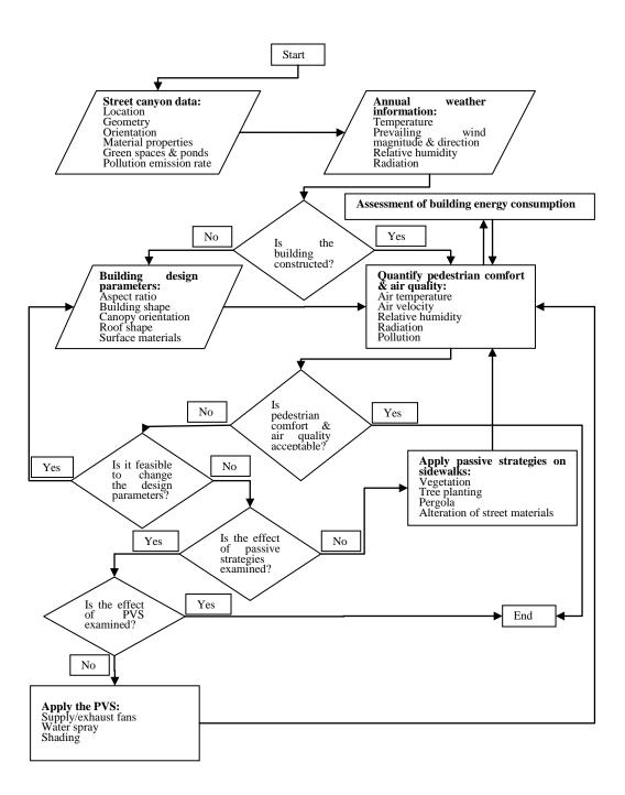
Figure 3.1 PCE-algorithm; a systematic model to evaluate and control PCE around the buildings
