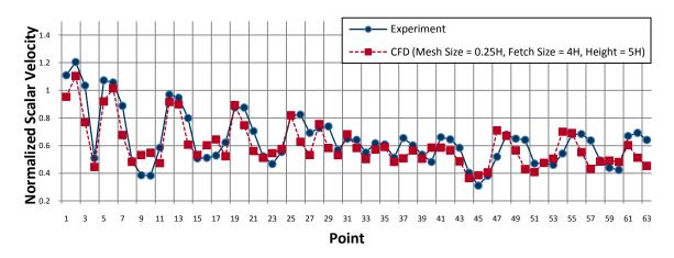
Figure 4.5 Comparison between measurement and CFD with suggested mesh size, domain height and fetch length
