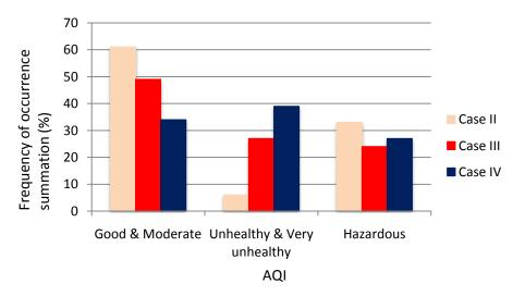
**Figure 4.14** Air quality index (AQI) frequency of occurrence summation for AR=2 (case II) changing albedo of buildings' surface (case III) and changing albedo of road and pavement (case IV)
