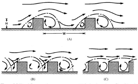
**Figure 2.2** The airflow over long street canyons (A) isolated roughness flow (B) wake interference flow (C) skimming flow (Oke, 1988)
