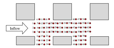
Figure 4.1 Half-domain measured points located 2mm above the ground (Top view) (Tominaga et al. 2008)
