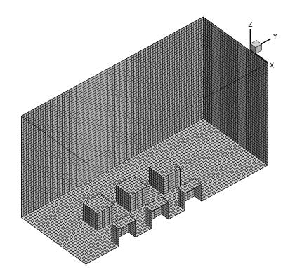
Figure 4.6 Domain and mesh size: fetch = 4H, height = 7H, mesh size = 0.25H(H=W=L=100mm)
