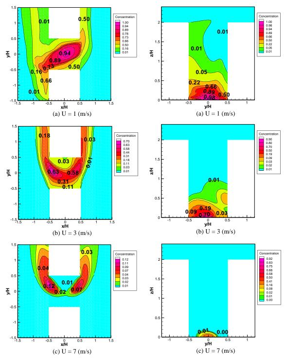
**Figure 4.19** Normalized pollution concentration: wind direction = 90 (degree) and AR = 2 (Left) Horizontal section 1.5 above the ground (Right) Vertical section in middle of the studied street canyon
