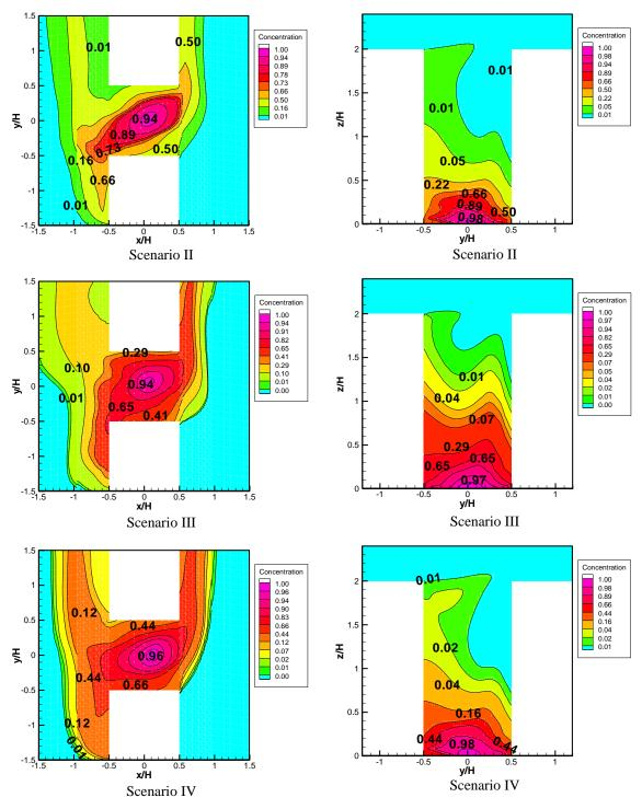
**Figure 4.24** Normalized pollution concentration: AR = 2, wind direction = 90 (degree), and wind velocity = 1 (m/s) for different scenarios (Left) Horizontal section 1.5 above the ground (Right) Vertical section in middle of the studied street canyon
