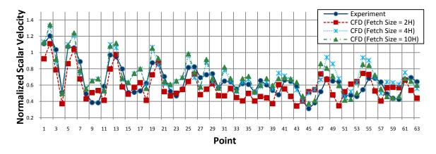
Figure 4.3 Comparison between measurement and CFD with different domain fetch
