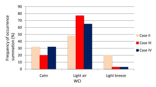
**Figure 4.16** Wind comfort index (WCI) frequency of occurrence summation for AR=2 (case II) changing albedo of buildings' surface (case III) and changing albedo of road and pavement (case IV)
