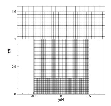
Figure 4.9 Structural meshes for pollution dispersion validation simulation domain
