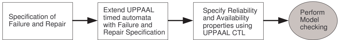
Figure 33: The process of modeling and verifying reliability and availability
