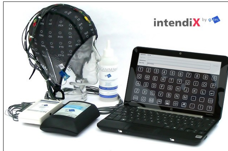
Figure 2.4: Setup of EEG operated spelling device and a skull cap
