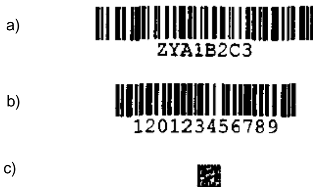
Figure 2.1. Area occupied by a 1-D bar code (a) and (b) vs. the 2-D (c) [14]
