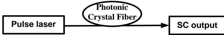
Figure 2.2: Experimental setup of a short pulse laser pumped SC source.
