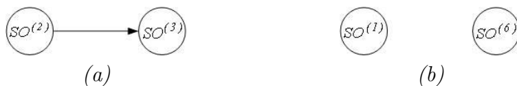
Figure 4.6: The sub-observer dependency (SOD) digraphs of (a) the supervisor-selected initial set of sub-observers \{SO^{(2)}, SO^{(3)}\} in the normal operation mode and (b) the supervisor-reconfigured set of sub-observers \{SO^{(1)}, SO^{(6)}\} in the process dynamics unreliability mode.
