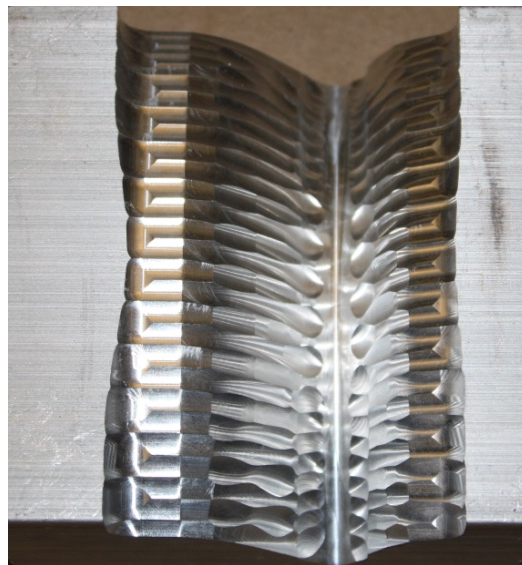
Figure 5.21 The sculptured surface cut with the CATIA NURBS CL paths.
