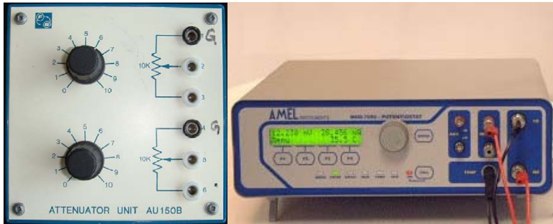
Figure 6 - Voltage Attenuator (left) and Potentiostat (right)
