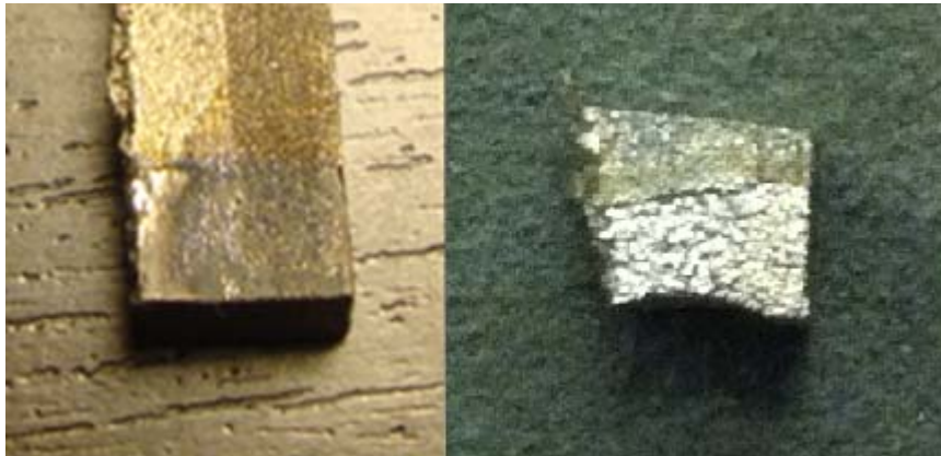
Figure 3-4 - Comparison Between Polishing Results with a Low Duty Cycle (left) and a High Duty Cycle (right).
