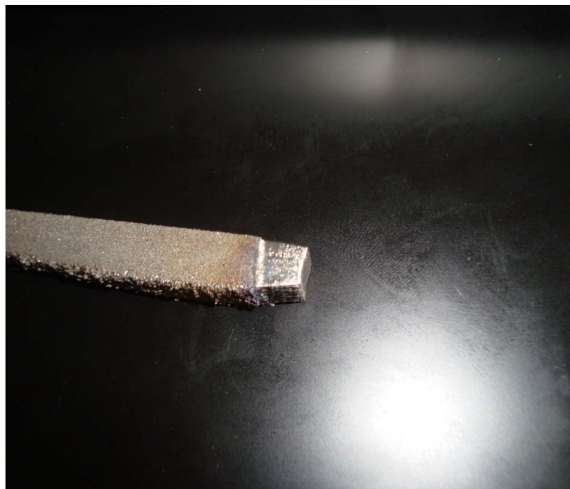
Figure 3-16 - Titanium Piece with Tip Electropolished.
