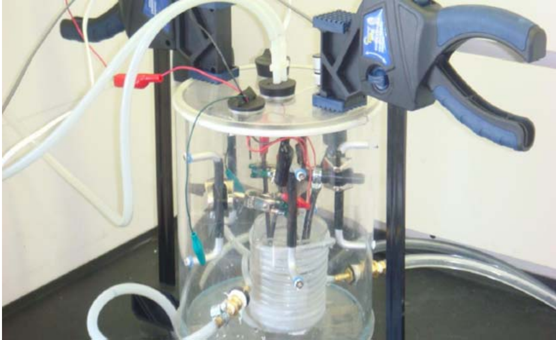
Figure 4-10 - Electrochemical Cell Designed for Polishing Ti.
