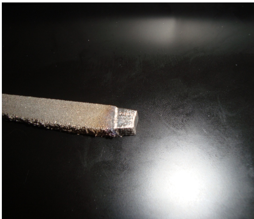
Figure 3-6 - Titanium Piece with Tip Electropolished.
