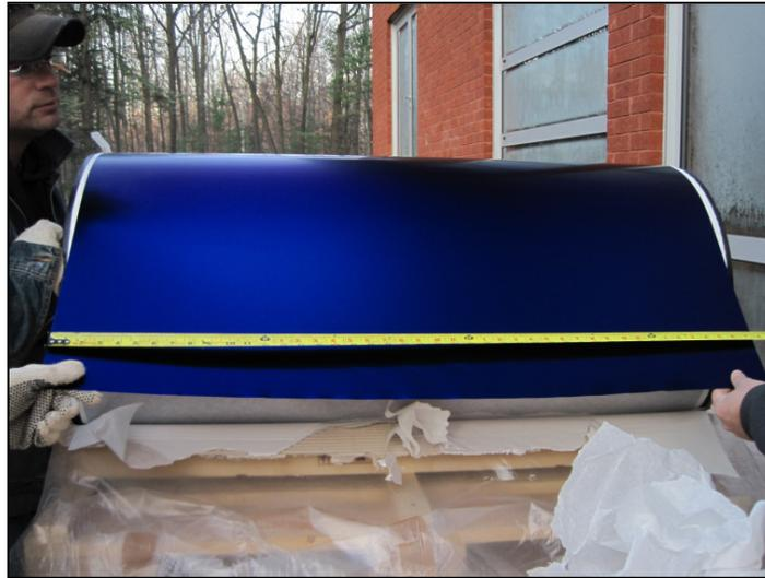
**Figure 4.12.** Low-emissivity absorber plate (TiNOX).
