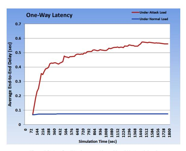
Figure 4.3: Avg.One Way Latency - Normal Load Vs Attack Load
