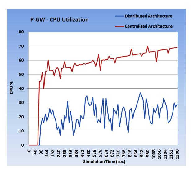
Figure 4.13: P-GW: CPU Utilization in Both Architectures
