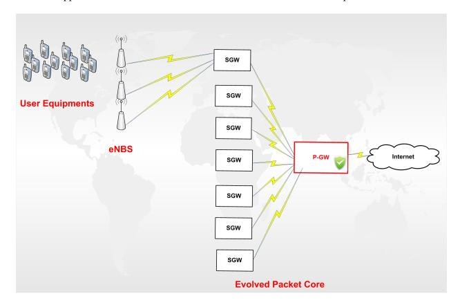
Figure 3.4: Centralized Security Architecture
