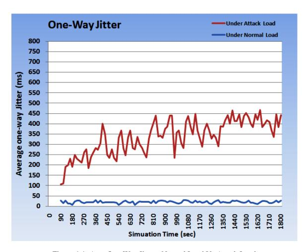
Figure 4.4: Avg. One-Way Jitter - Normal Load Vs Attack Load
