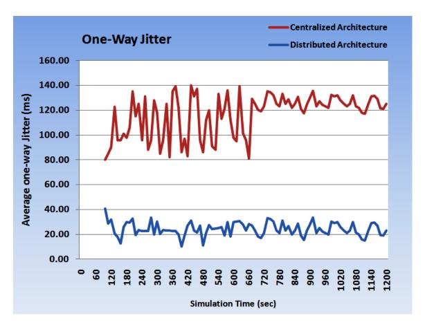
Figure 4.8: Avg. One-Way Jitter In Both Security Architectures
