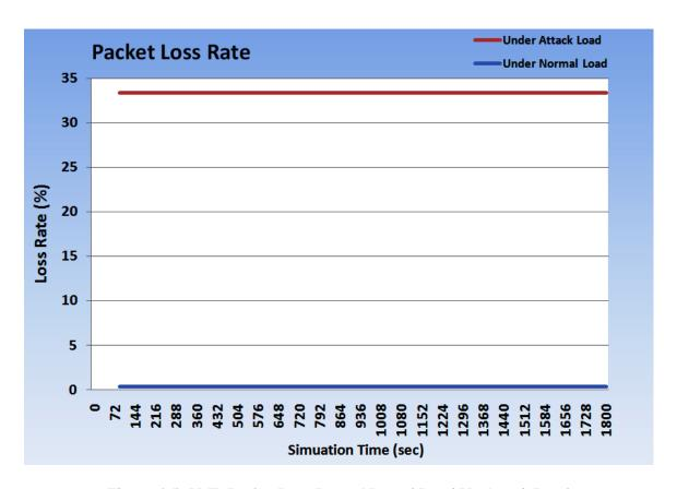
Figure 4.5: VoIP Packet Loss Rate - Normal Load Vs Attack Load
