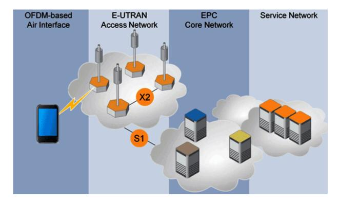
Figure 3.2: LTE 4G Mobile Architecture
