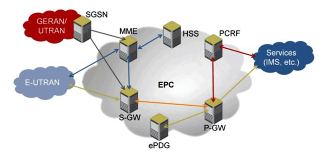
Figure 3.3: LTE Evolved Packet Core
