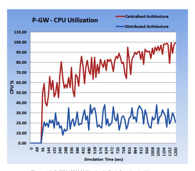
Figure 4.6: P-GW: CPU Utilization in Both Security Architectures
