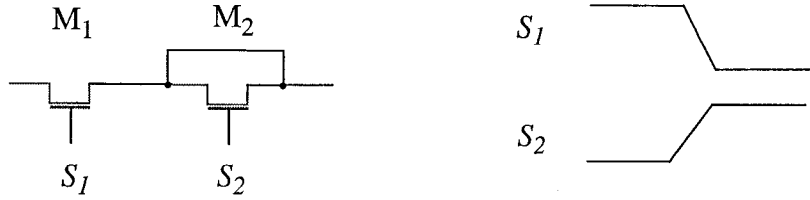
Figure 2.10 Dummy switch technique to reduce charge injection [24]. The charge released from the channel of the transistor M_1 is absorbed by the dummy transistor M_2 .
