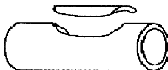
Figure 2.6 Ruptured Pipe (NRCC & FCM Sept. 2002)
