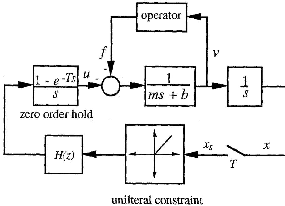
**Figure 1-6 Model of a one degree-of-freedom haptic interface [44]**
