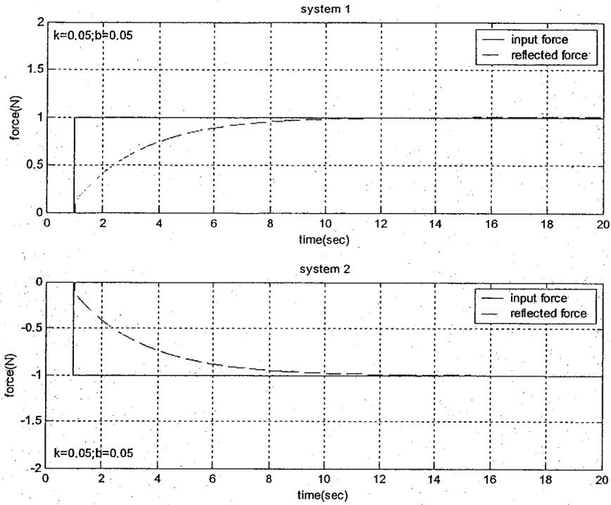
Figure 5-11 The response of case I with  $k = 0.05\text{N/m}$  and  $b = 0.05\text{N}\cdot\text{sec/m}$
