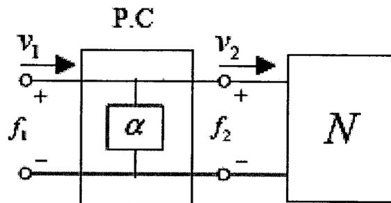
(b) Parallel or force conserving Passivity Controller.
