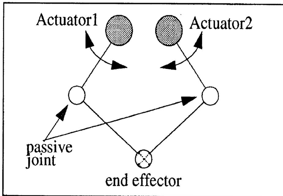
Figure 1-3 Schematic representation of a typical 2DOF parallel manipulator [26]
