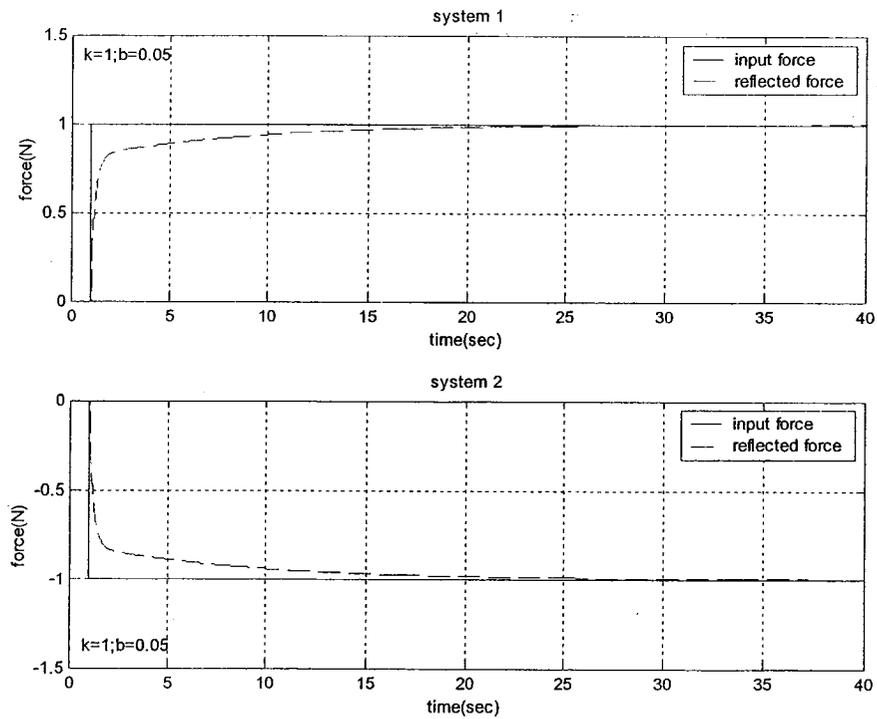
Figure 5-14 The response of case II with  $k = 1 \text{ N/m}$  and  $b = 0.05 \text{ N-sec/m}$
