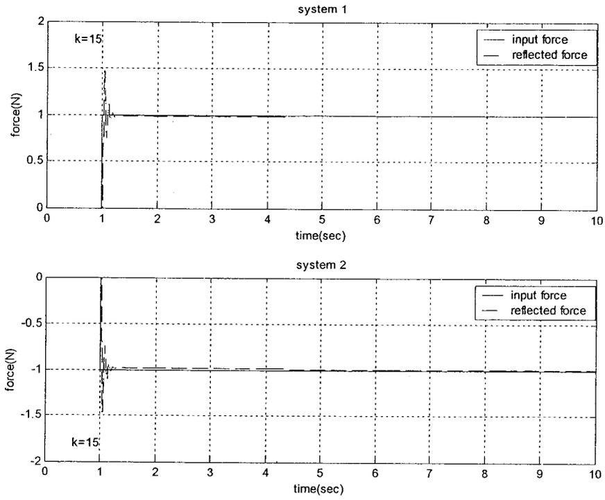
Figure 5-4 The response of spring model with coefficient  $k = 15$  N/m
