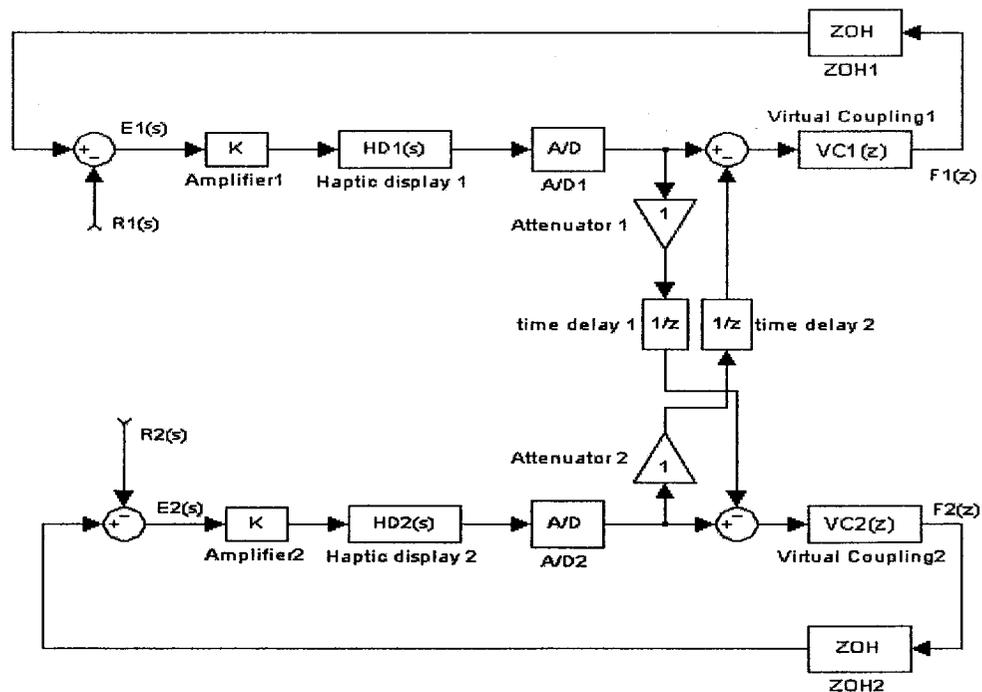
Figure 3-4 Networked haptic feedback system
