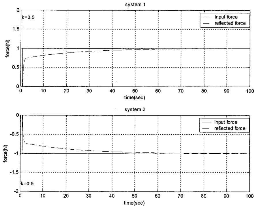
Figure 5-7 The response of spring model with coefficient  $k = 0.5 \text{ N/m}$
