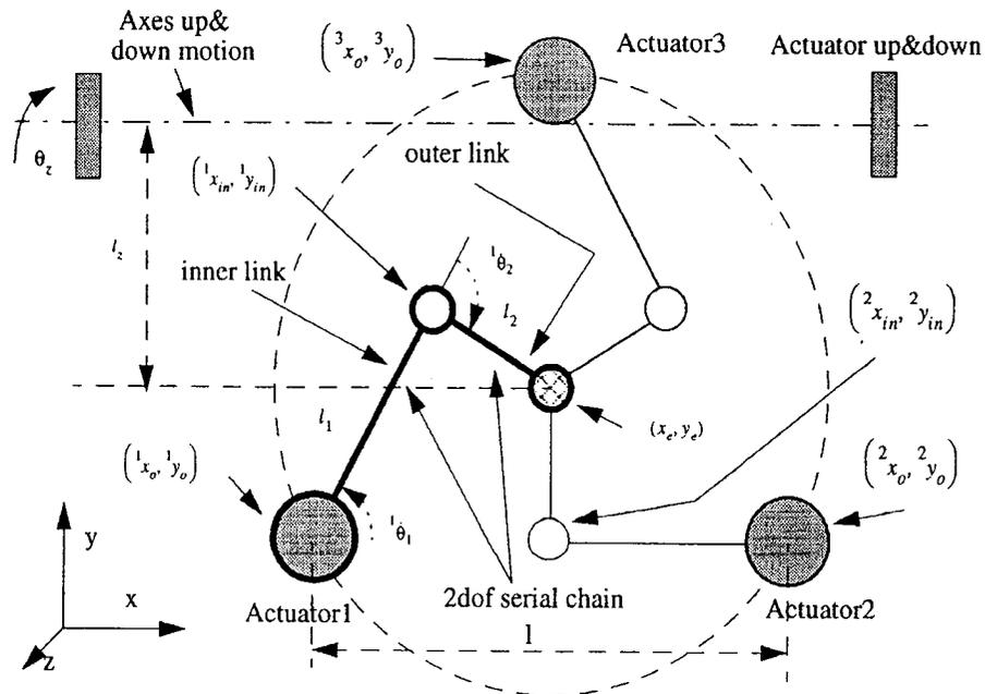
Figure 1-4 Schematic representation of the pen-based force display [26]
