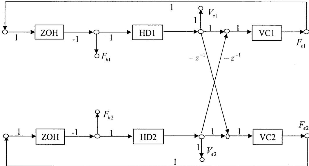
Figure 3-5 Signal flow graph of a networked haptic display
