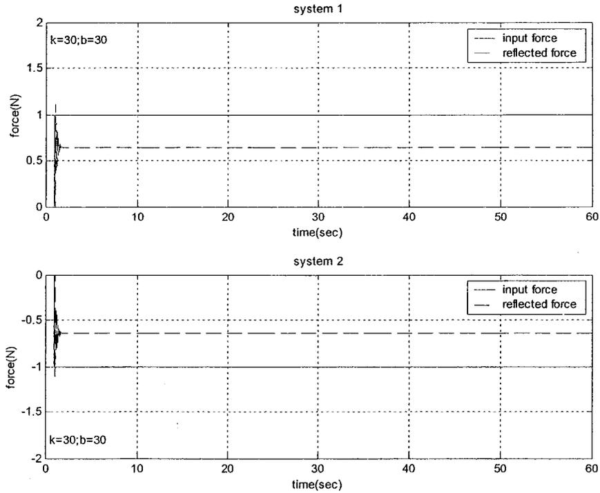
**Figure 5-19 The response of case III with  $k = 30 \text{ N/m}$  and  $b = 30 \text{ N}\cdot\text{sec/m}$**
