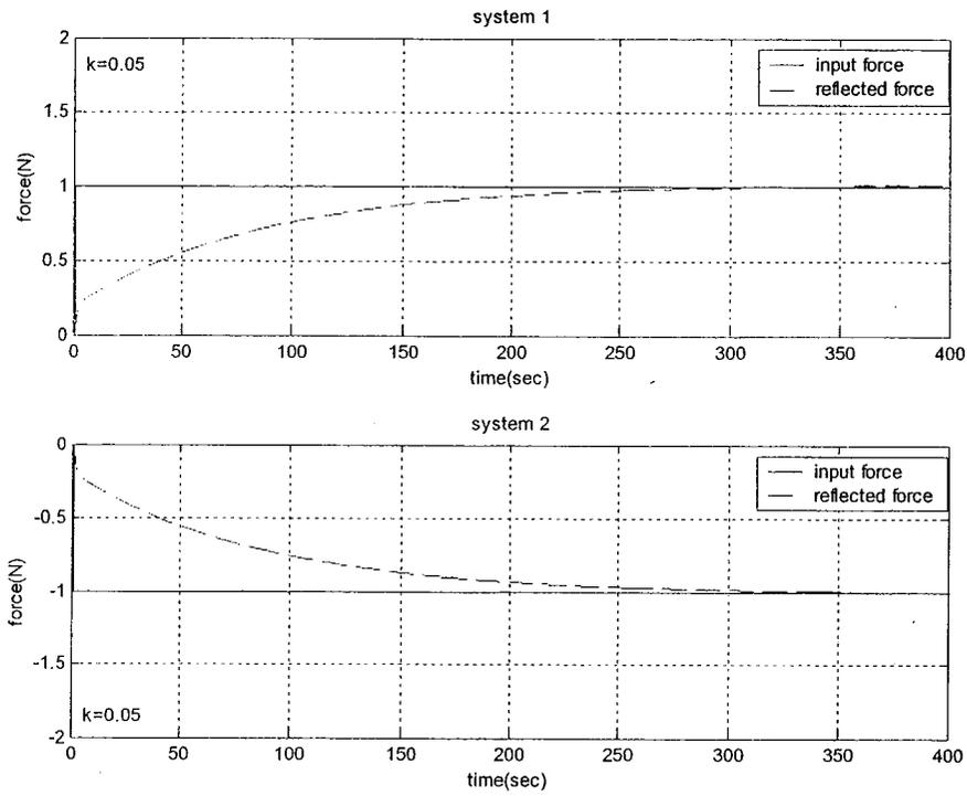
Figure 5-8 The response of spring model with coefficient  $k = 0.05 \text{ N/m}$
