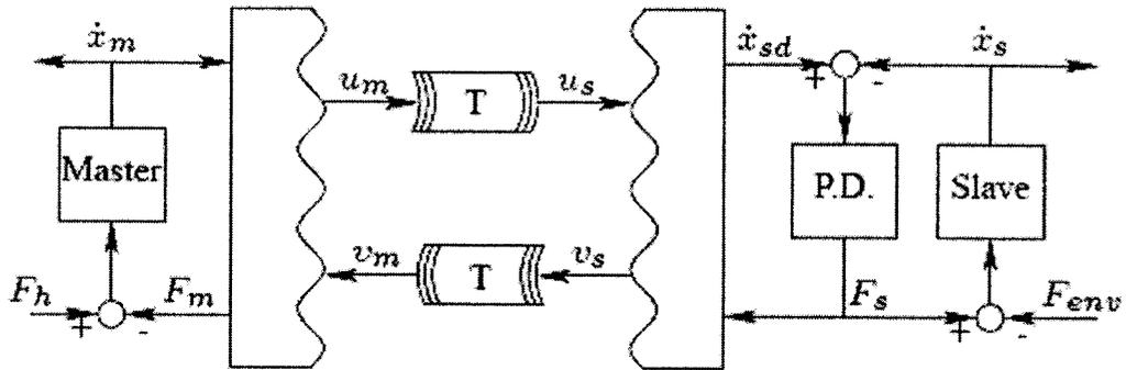
**Figure 1-10 A basic configuration for a wave variable based teleoperator system[67]**
