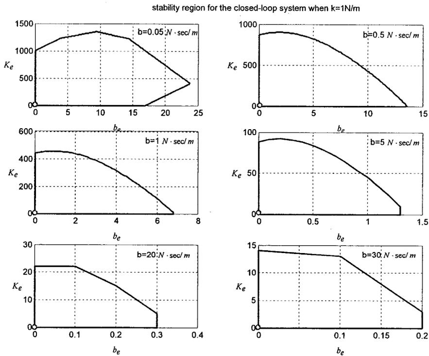
**Figure 4-7** The stability condition for the case with  $k = 1 N/m$
