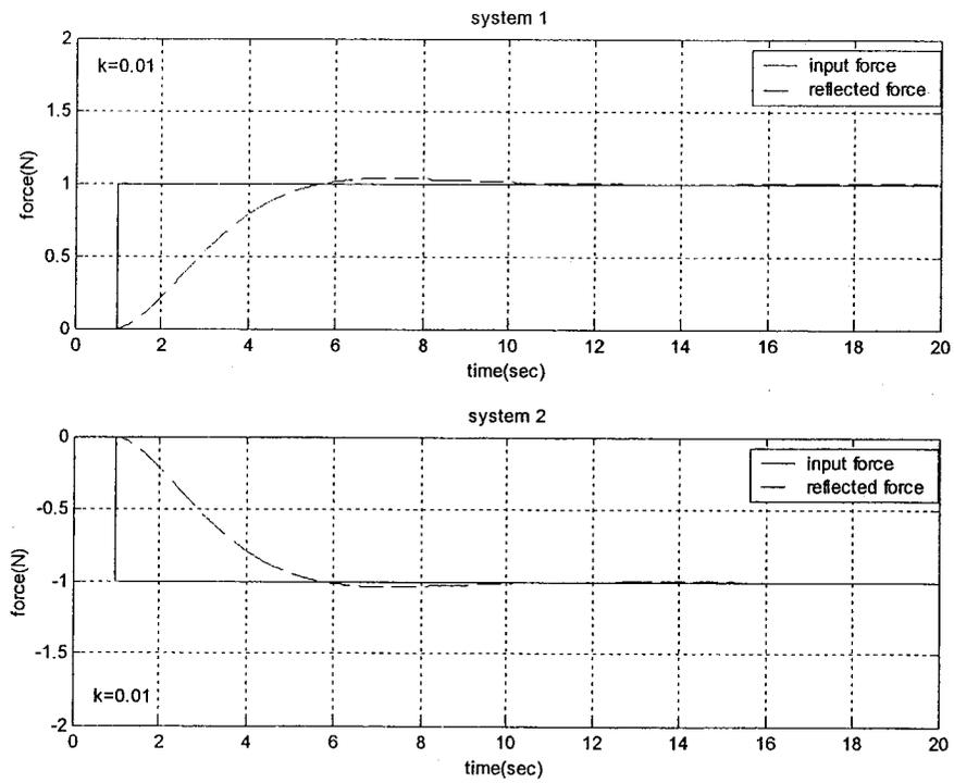
Figure 5-9 The response of spring model with coefficient  $k = 0.01 \text{ N/m}$
