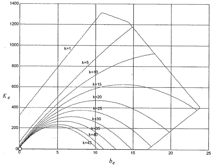
Figure 4-5 The region of parameters  $(K_e, b_e)$  for different spring coefficients
