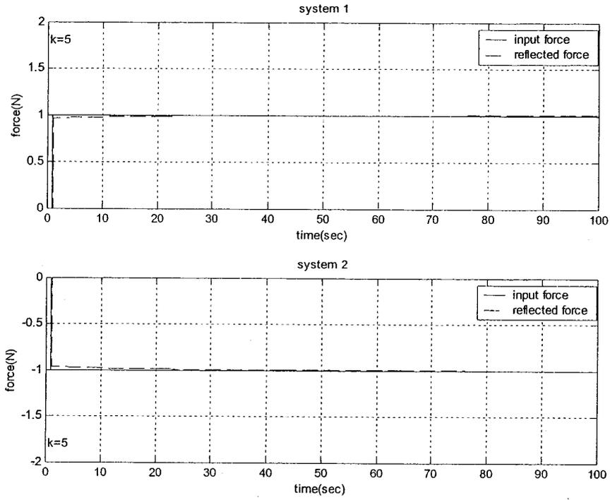
Figure 5-2 The response of spring model with coefficient  $k = 5 \text{ N/m}$
