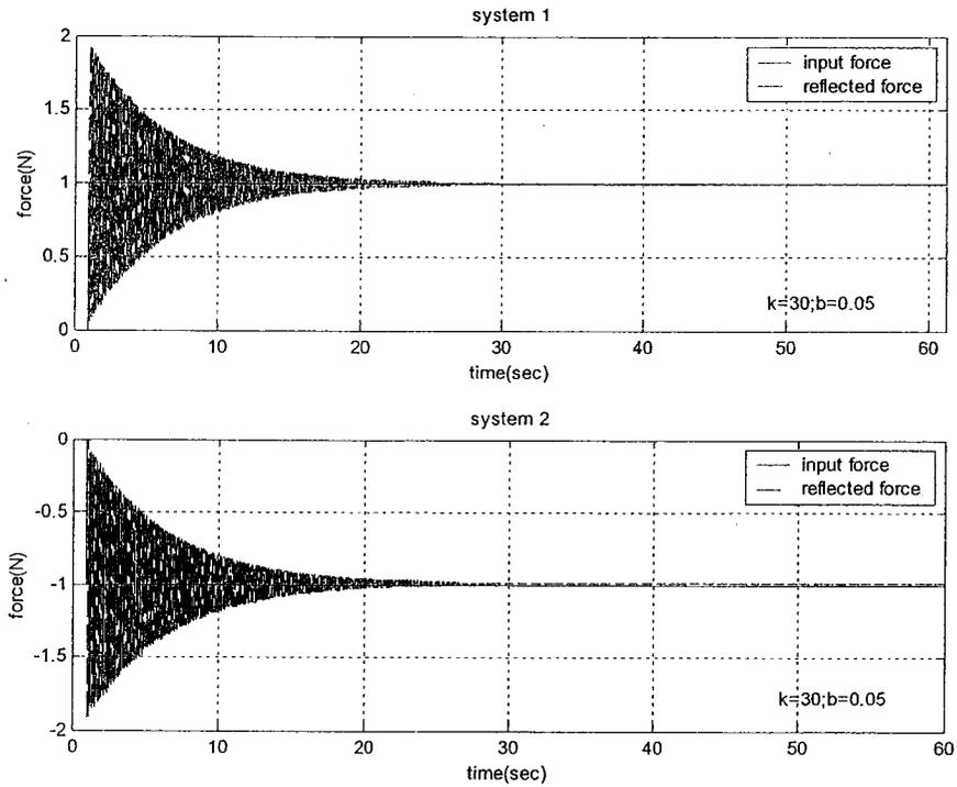
Figure 5-17 The response of case III with  $k = 30\text{N/m}$  and  $b = 0.05\text{N-sec/m}$
