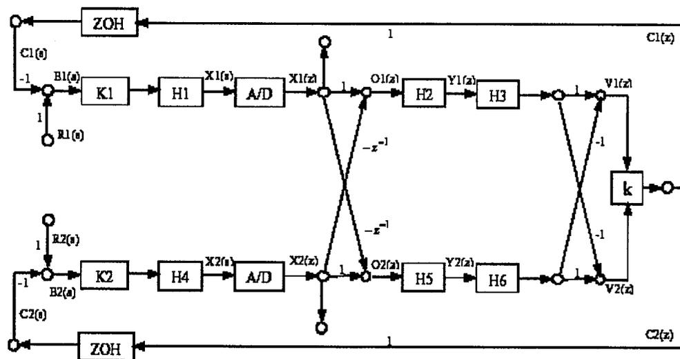
Figure 4-3 Signal flow graph of networked haptic display with VE
