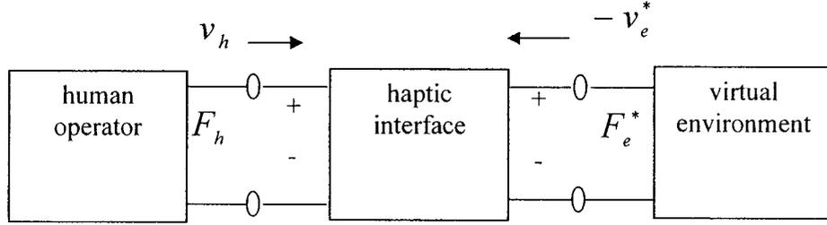
**Figure 3-2 Network model of haptic simulation**
