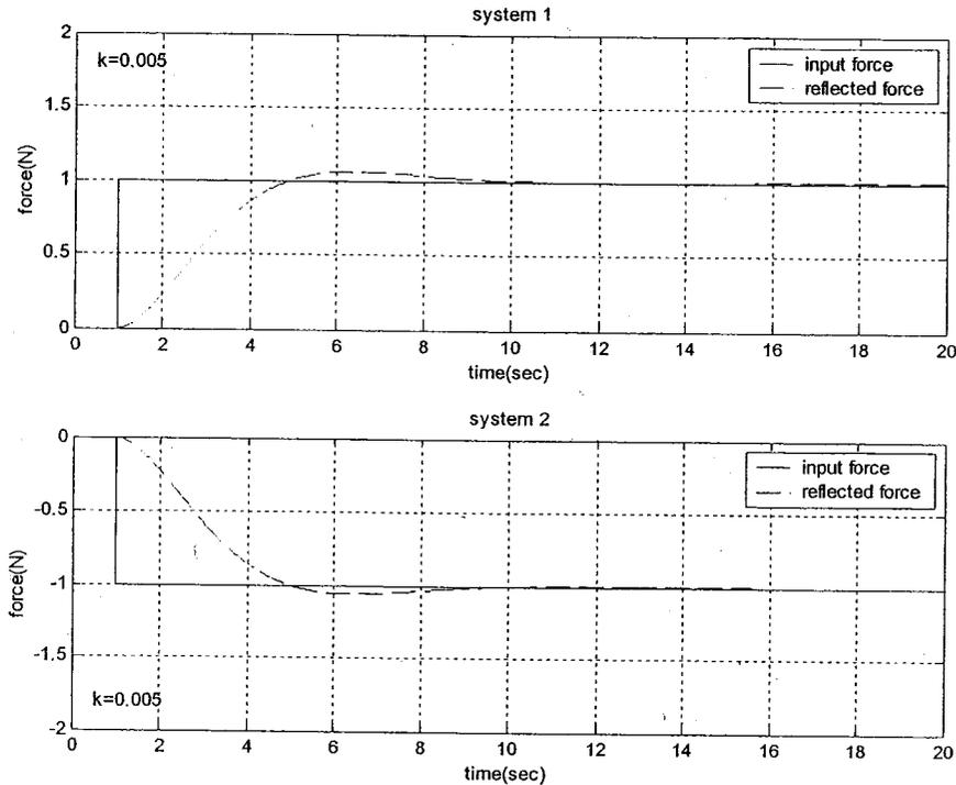
Figure 5-10 The response of spring model with coefficient  $k = 0.005 \text{ N/m}$
