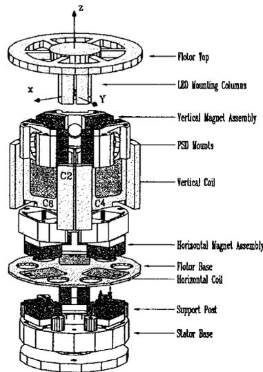
**Figure 1-1 The UBC maglev joystick assembly sketch [25]**
