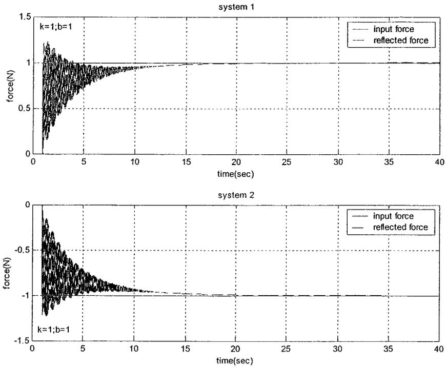
Figure 5-15 The response of case II with  $k = 1 \text{ N/m}$  and  $b = 1 \text{ N-sec/m}$
