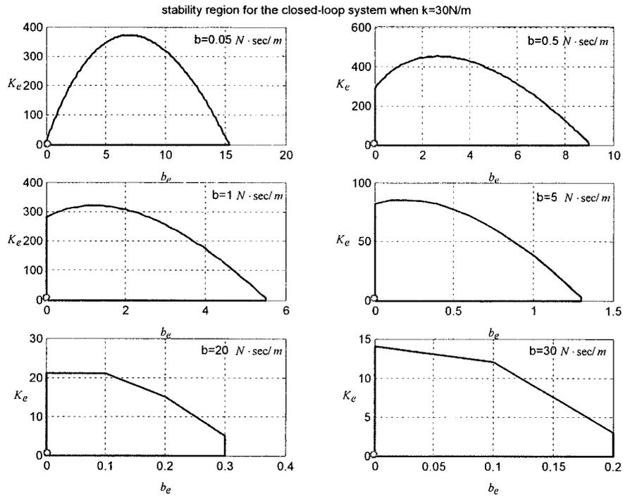
**Figure 4-8** The stability condition for the case with  $k = 30 \text{ N/m}$
