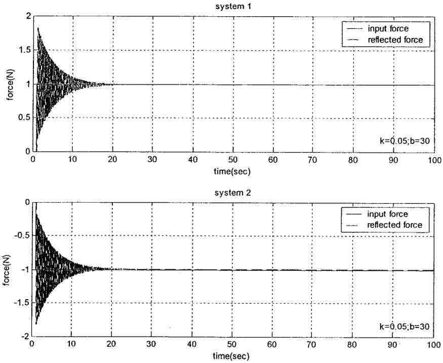
Figure 5-13 The response of case I with  $k = 0.05 \text{ N/m}$  and  $b = 30 \text{ N-sec/m}$
