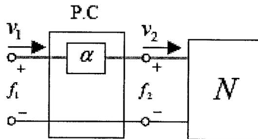
(a) Series or velocity conserving Passivity Controller
