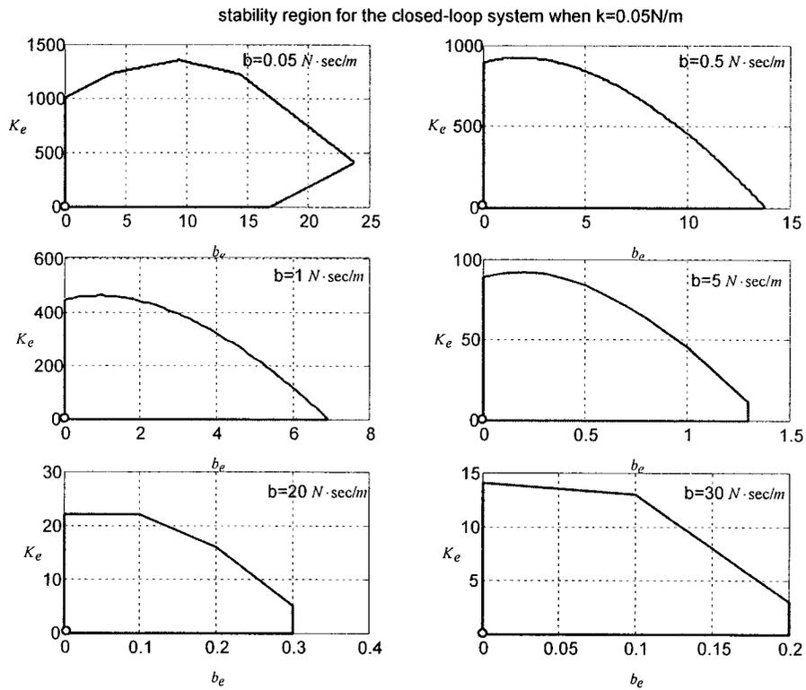
**Figure 4-6** The stability condition for the case with  $k = 0.05 N/m$
