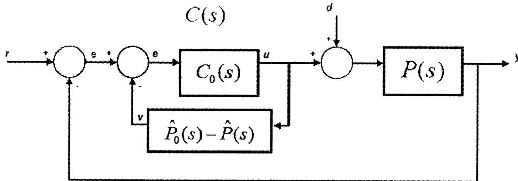
Figure 1-11 A classical diagram of a control system incorporating a Smith Predictor [83]
