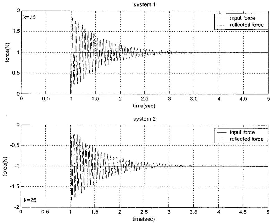
Figure 5-6 The response of spring model with coefficient  $k = 25 \text{ N/m}$
