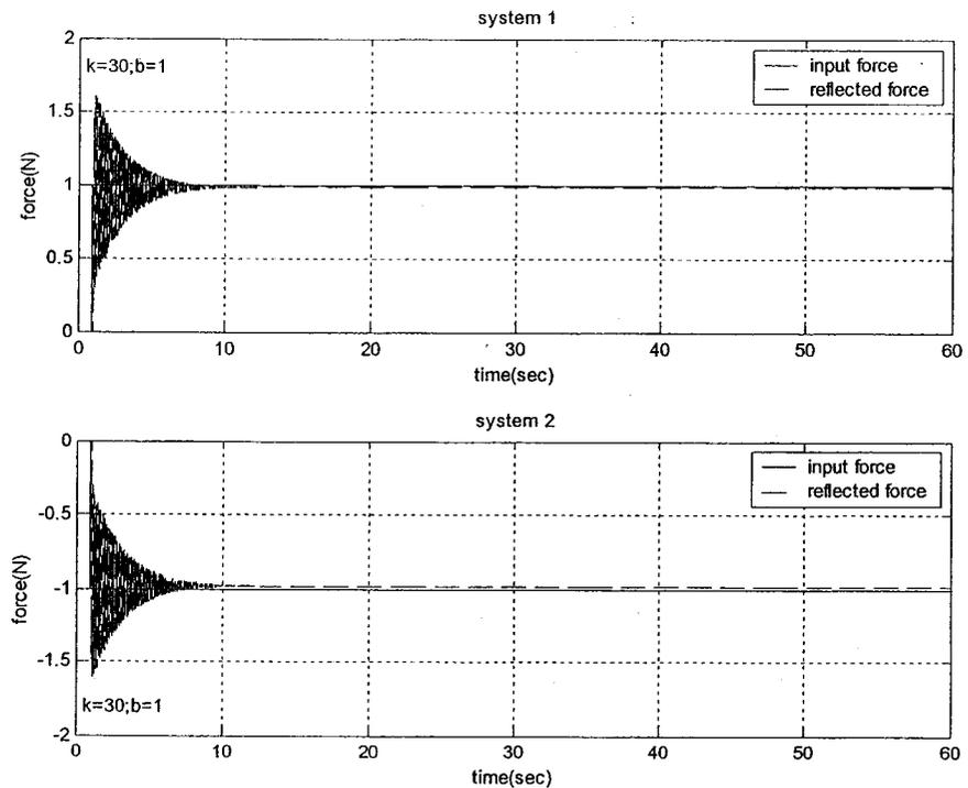
Figure 5-18 The response of case III with  $k = 30\text{N/m}$  and  $b = 1\text{N-sec/m}$
