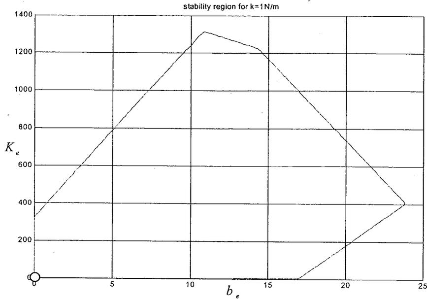
**Figure 4-4 Stability of the x-axis for the closed-loop system**
