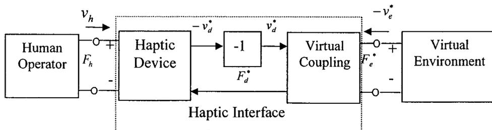
**Figure 3-3 Haptic interface for the impedance display case includes both the haptic display and a virtual coupling network**
