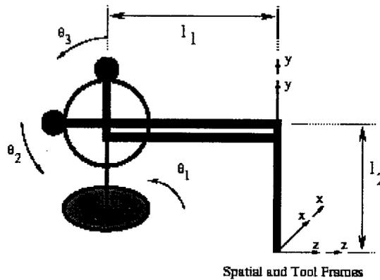
Figure 2-1 Zero configuration of the manipulator [88]
