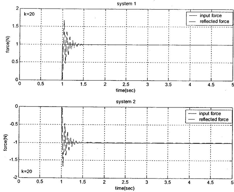
Figure 5-5 The response of spring model with coefficient  $k = 20$  N/m
