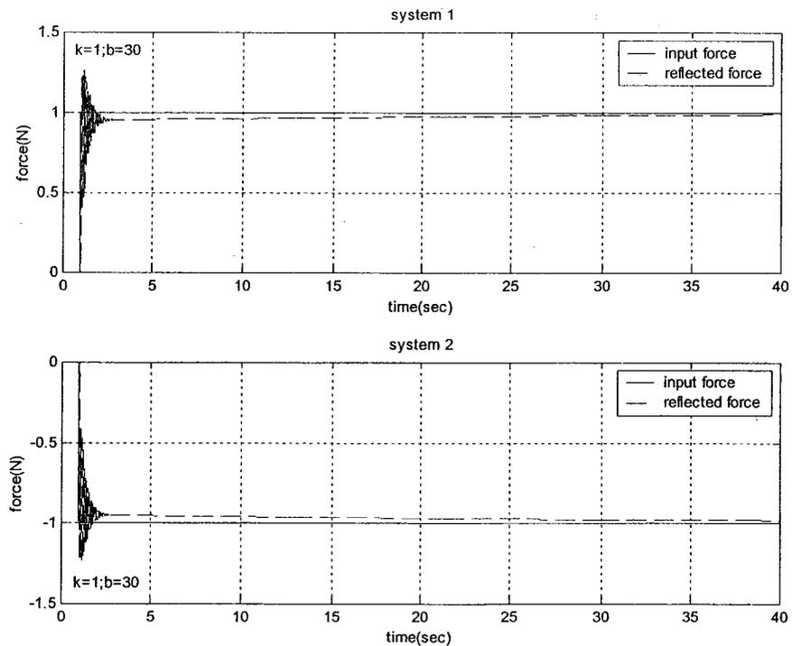
Figure 5-16 The response of case II with  $k = 1 \text{ N/m}$  and  $b = 30 \text{ N-sec/m}$
