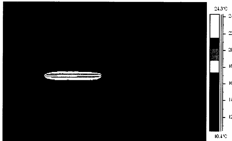
Figure 4.4 Thermogram of the panel surface temperature distribution due to air leaks using a few colors palette
