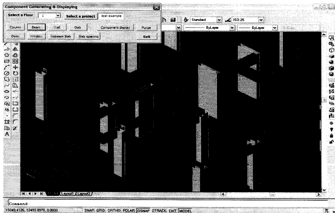
Figure 4.69 3D View of Columns and Beams
