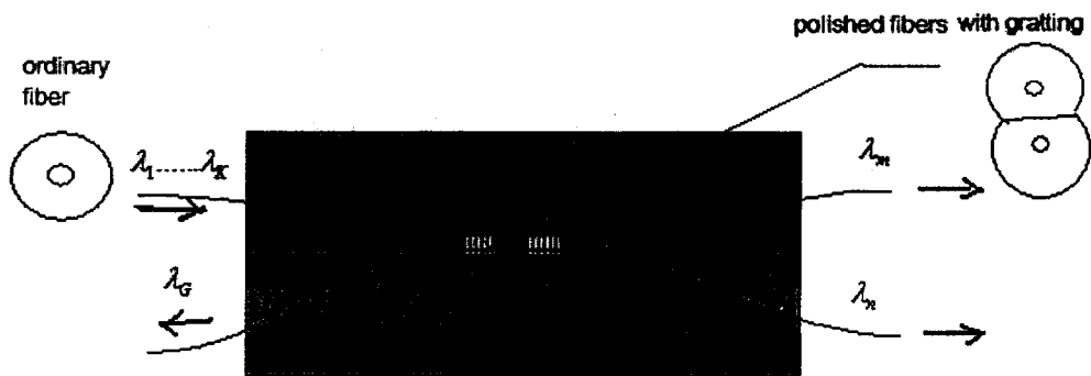
Figure 5.25 Side-polished fiber-types WDM with FBG
