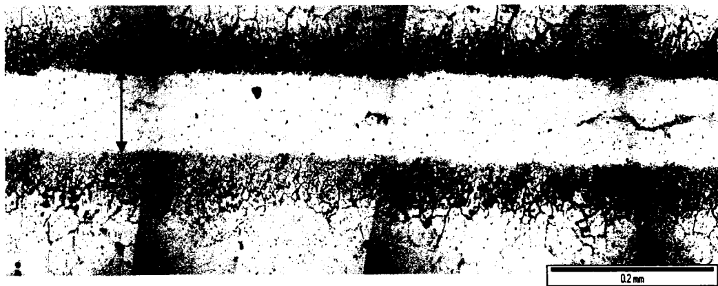
Fig. 5.12 Micrograph showing the initiation of brittle eutectic phase (Inconel 718/BNi-2 joint brazed at 1394K for 50 minutes)
