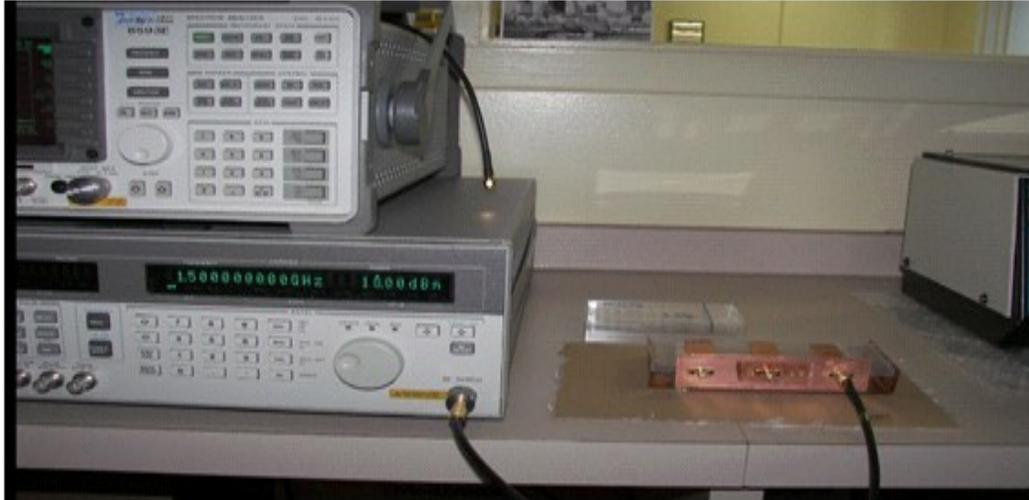
**Figure 5.2:** The generator is connected to one of the inputs of the RF apparatus for RF radiation exposure. Uveal melanoma cell lines 92.1 and Fibroblast in a media are filled in 96 well plates
