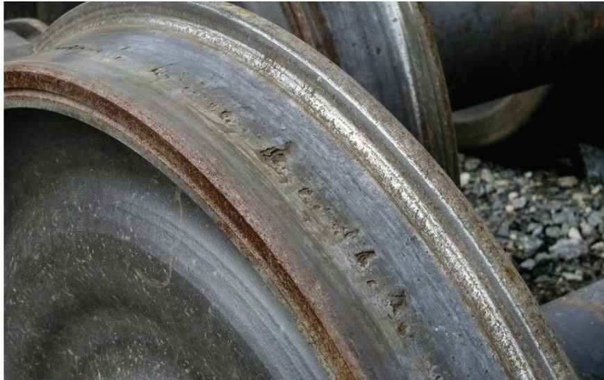
Fig. 1. 22: Wheel shelling defect.
