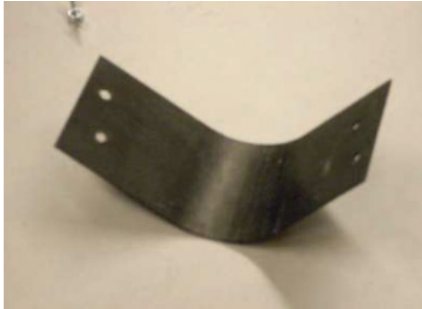
Figure 5.1: Coupon with holes for fixing
