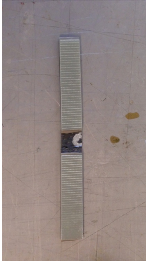
Figure 5.7: Coupon for compression test
