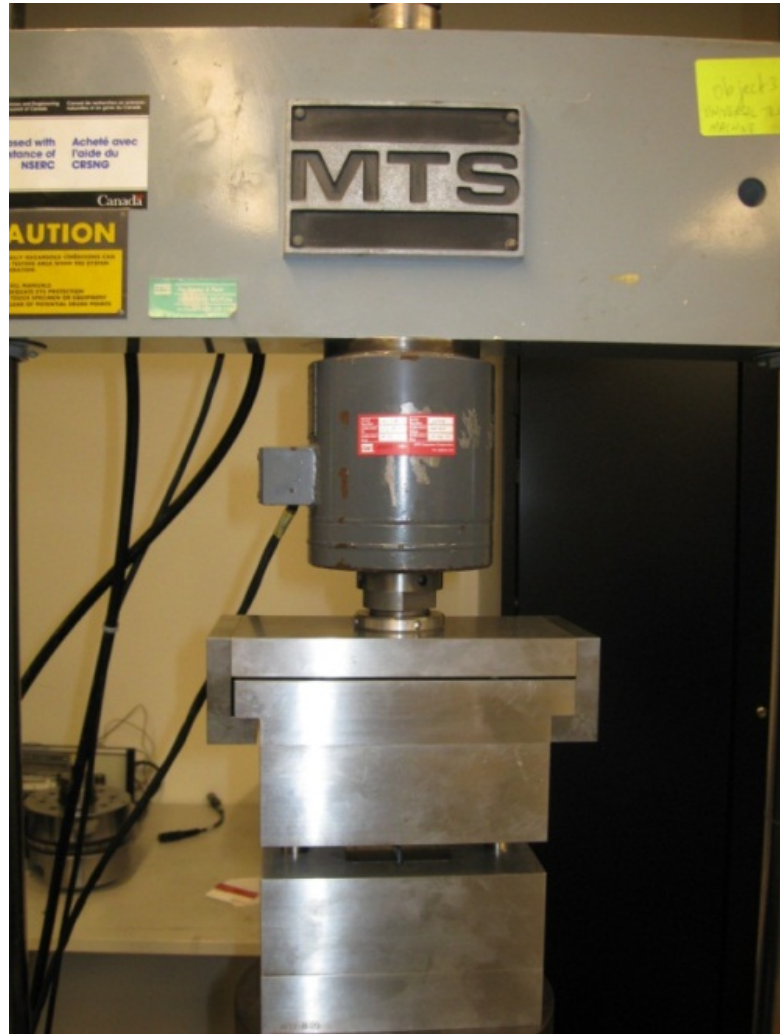
Figure 5.8: Compression test with MTS
