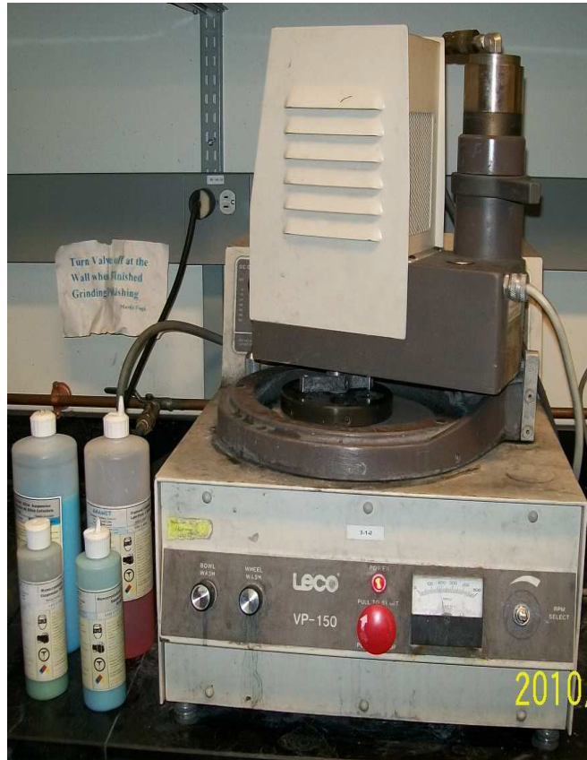
Figure 5.14: Automatic grinding machine LECO VP-150
