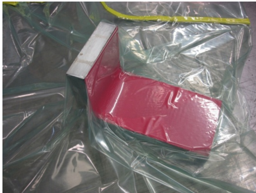
Figure 3.7 Consolidation with vacuum bag
